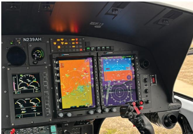
Moog's Genesys Avionics Suite™ designed for the Airbus H125 helicopter enhances the capabilities of this Airbus Helicopter workhorse platform. The solution features two IDU-680 displays in a PFD/MFD format, dual redundant ADAHRS, Dual GPS/FMS, dual Genesys GDR digital Nav/Comm radios, and IFR certified Genesys rotary-wing autopilot with Stability Augmentation System (SAS).
