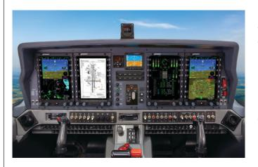
Moog's Genesys Avionics Suite provides the latest state-of-the-art avionics allowing seamless transition to modern training platforms. The primary flight display features tapes display or round dial display unique for this class of trainer aircraft. The aircraft provides for VFR and IFR day and night operations. Available safety features include Traffic Advisory System (TAS), digital Flight Data and Cockpit Voice Recorder (FDR & CVR) and Mission Debriefing System (MDS).
