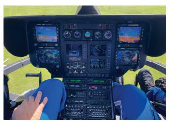
The Genesys Avionics Suite<sup>™</sup> designed for the Airbus EC-145e helicopter features four IDU-450 displays in a dual-sided PFD/MFD format, dual redundant ADAHRS, Dual GPS/FMS, and IFR certified Genesys GRC<sup>™</sup> Rotorcraft Autopilot & Stability Augmentation System (SAS).
