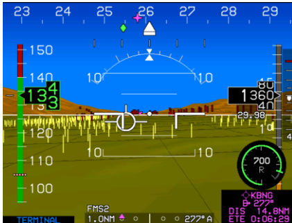
Obstructions without hazardous condition
