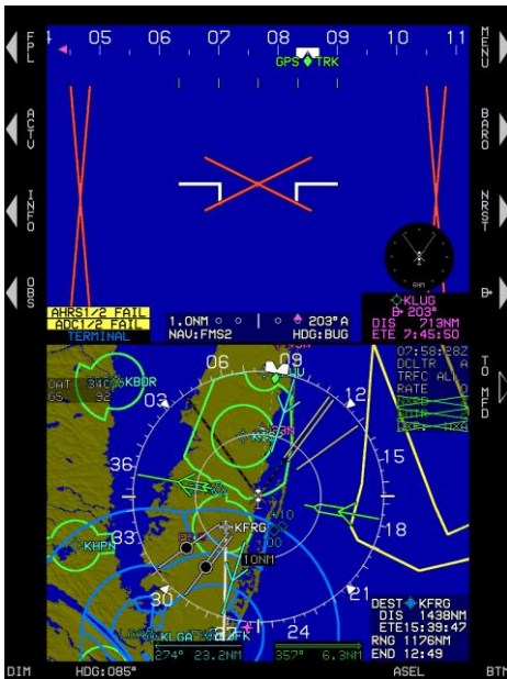
Figure 4 21: MFD Failure Mode 6 ADC and AHRs Failed, GPS/SBAS Normal
