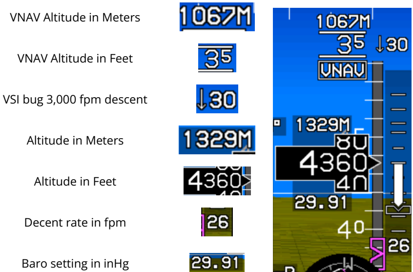
Figure 2-60: Altitude Display (Feet)
