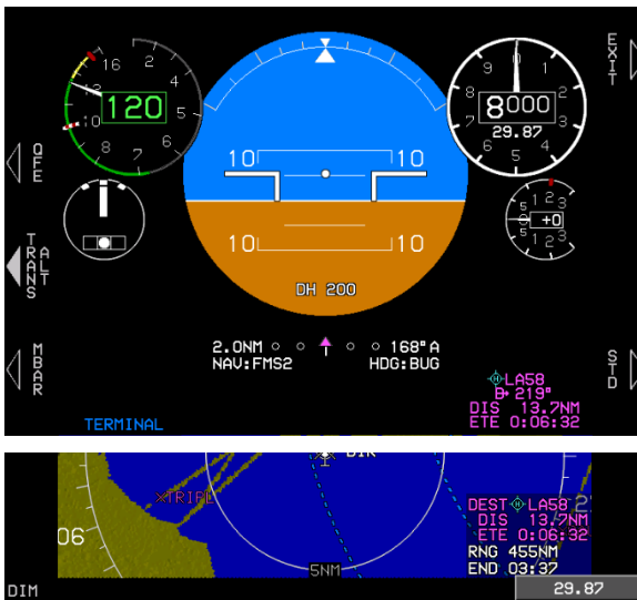
Figure RD-9: Altimeter Setting
