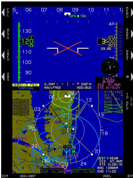
Figure 5-14: MFD Failure Mode 3 AHRS Failed, GPS/SBAS and ADC Normal
