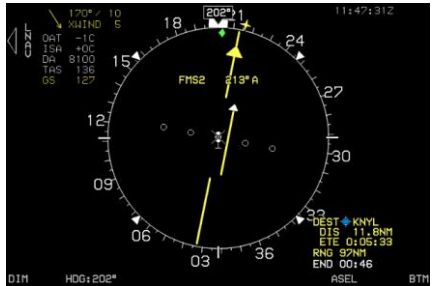
GPS Loss of Integrity or Loss of Navigation Amber (Yellow) Pointer and Waypoint Information
