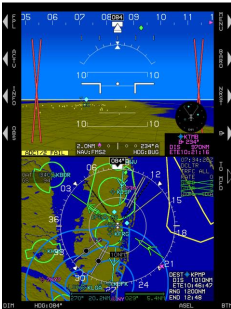
Figure 5-12: MFD Failure Mode 2 ADC Failed, GPS/SBAS and AHRS Normal
