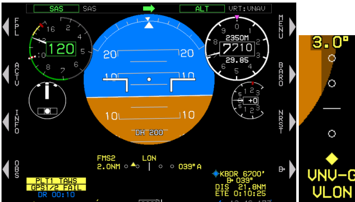
Figure RD-23: VDI Color during GPS/SBAS LOI/LON or VLON
