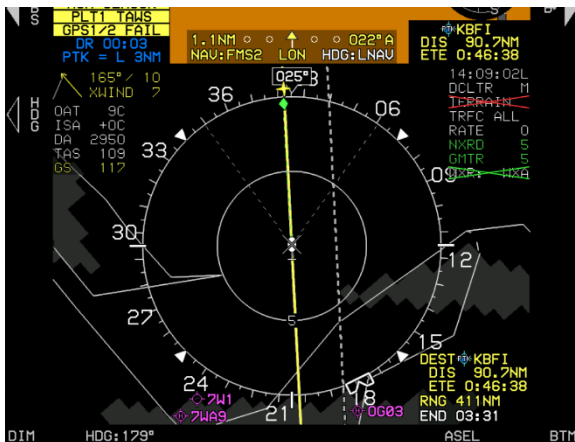
Figure 2-80: Loss of Navigation
