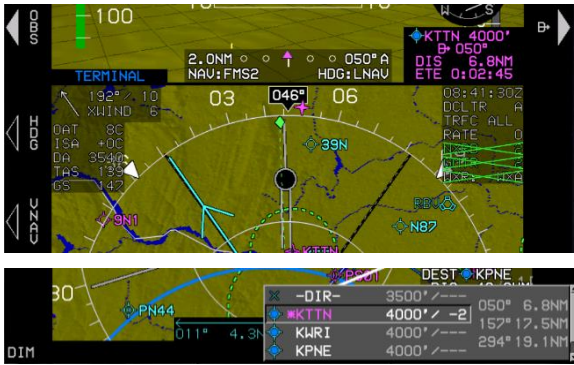
Figure 2-18: Altitude Display (VNAV)
