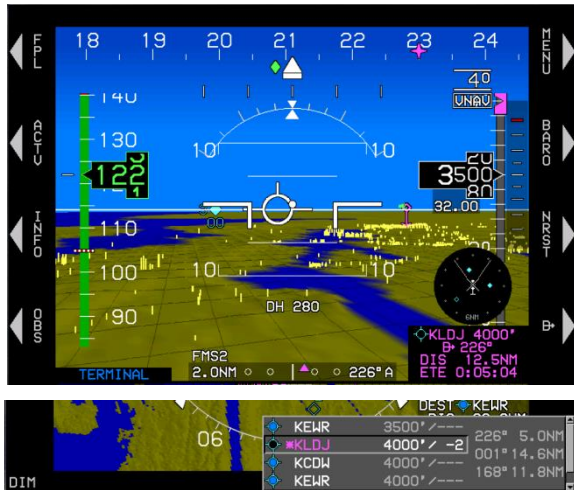
Figure 2-19: VNAV Sub-Mode (Not Vertically Integrated) (Feet for Altitude and NM for Distance)
