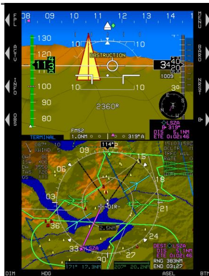
PFD SVS TAWS with Obstruction Caution (Obstruction depictions on PFD and map highlighted but do not flash)
