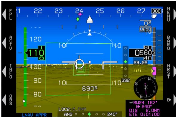
Figure 6-9: Highway in the Sky Final Approach Segment
