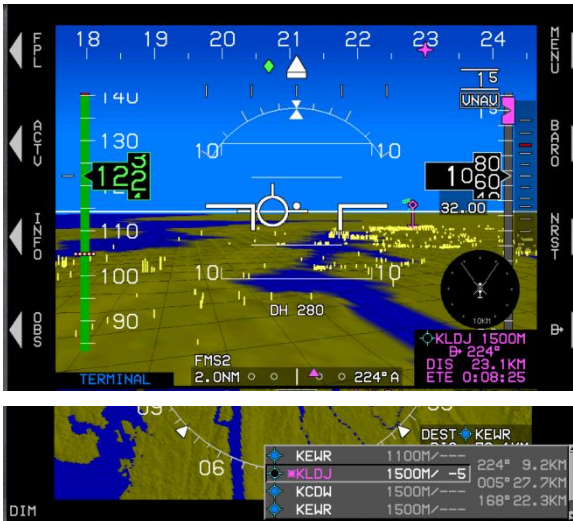
Figure 2-20: VNAV Sub-Mode (Not Vertically Integrated) (Meters for Altitude and KM for Distance)
