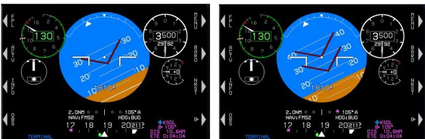
Pitch up 25° Recovery Chevrons Only Pitch up 30° Unusual Attitude Mode
