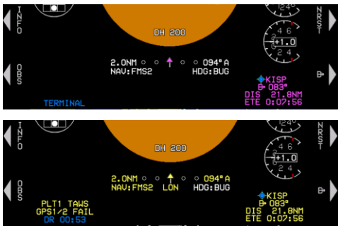
Figure RD-24: Course Deviation Indicator
