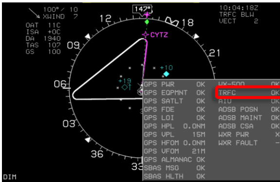
Figure T-14: Menu Faults Status
