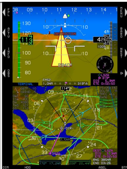
PFD SVS TAWS with Obstruction Warning (Obstruction depictions on PFD and map highlighted and flash)
