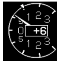
VSI bug set to +1,000 fpm without autopilot enabled
