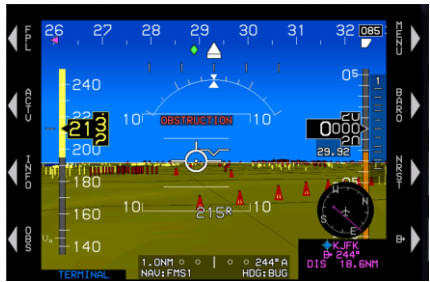
Obstructions creating an OBSTRUCTION warning
