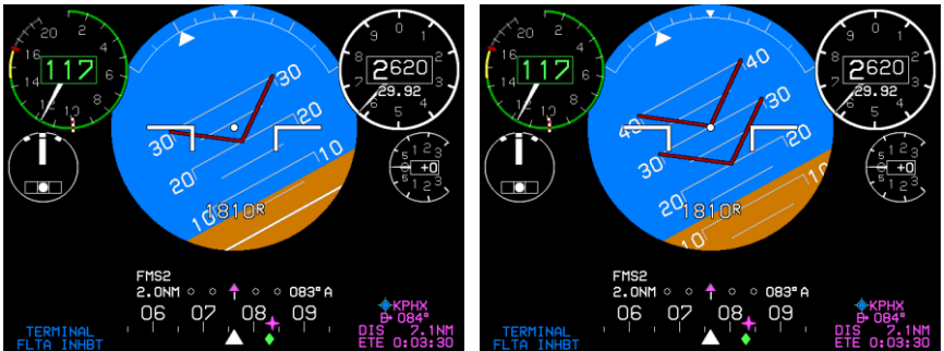
Pitch up 25° Recovery Chevrons Only Pitch up 30° Unusual Attitude
