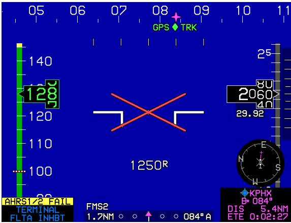
Figure 5-13: PFD Failure Mode 3 AHRs Failed; GPS/SBAS and ADC Normal
