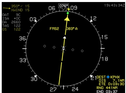
GPS Loss of Integrity or Loss of Navigation Amber (Yellow) Pointer and Waypoint Information
