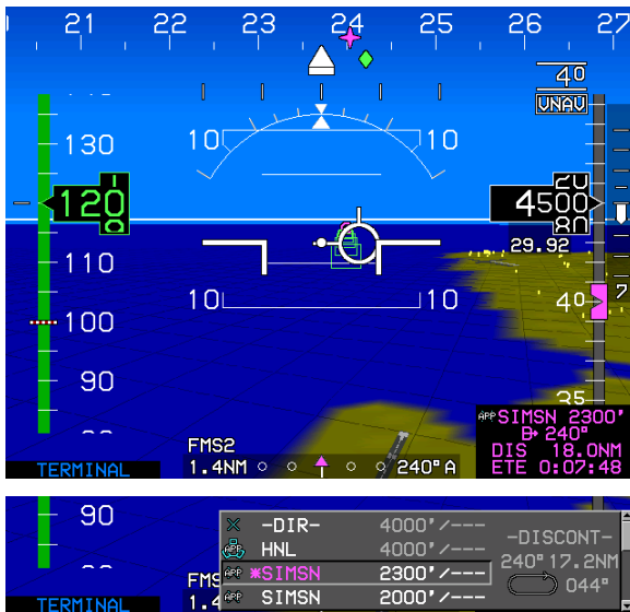
Figure 2-17: VNAV Sub-Mode (Not Vertically Integrated)
