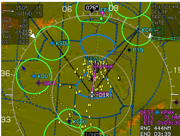
Figure 5-8: MFD Failure Mode 0 GPS, ADC, and AHRS Normal
