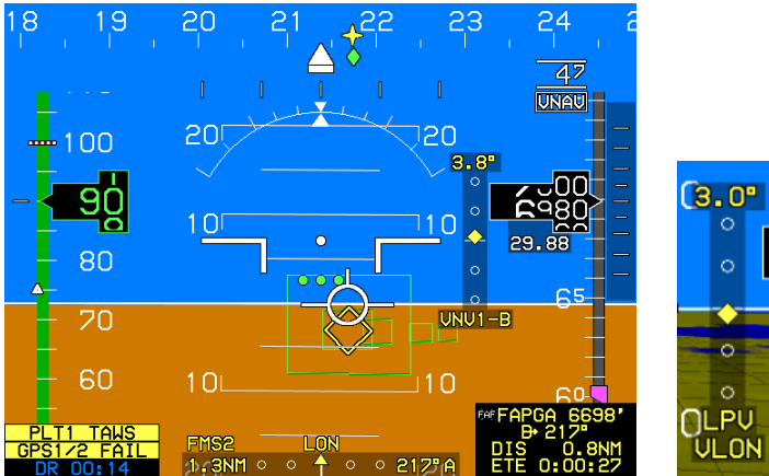
Figure 2-49: VDI Color during GPS/SBAS LOI/LON or VLON
