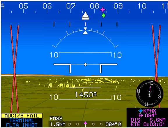
Figure 5-11: PFD Failure Mode 2 ADC Failed; GPS/SBAS and AHRS Normal
