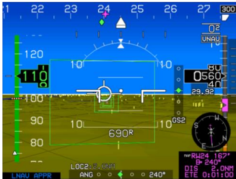
Figure 6-9: Highway in the Sky Final Approach Segment
