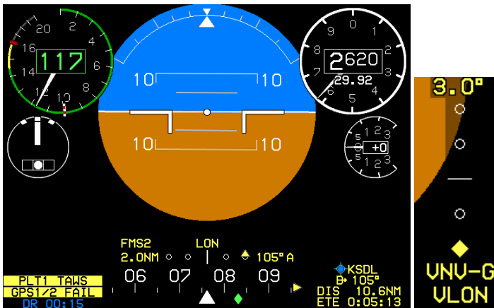
Figure RD-22: VDI Color during GPS/SBAS LOI/LON or VLON
