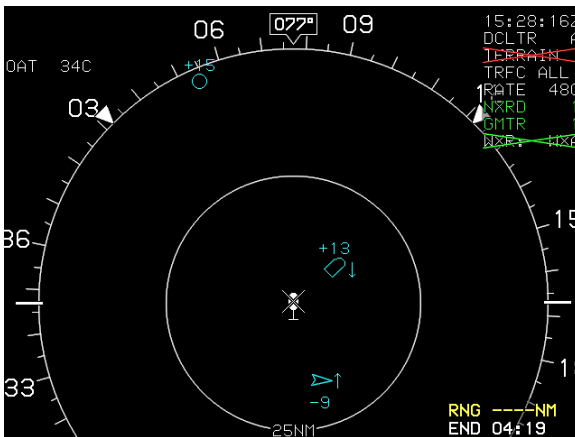
Figure 5-16: MFD Failure Mode 4 GPS/SBAS and ADC Failed; AHRS Normal
