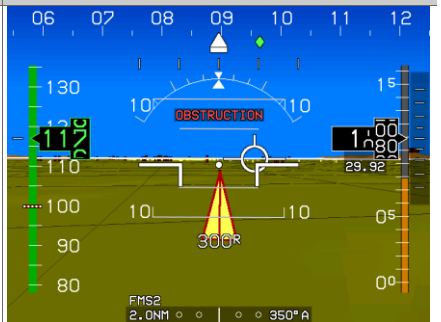
PFD SVS TAWS with Obstruction Warning (Obstruction depictions on PFD and map highlighted and flash)
