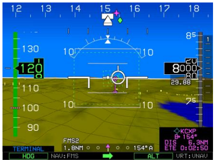
Uncoupled from skyway with autopilot
