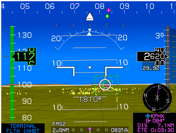
Figure 5-7: PFD Failure Mode 0 GPS, ADC, and AHRS Normal
