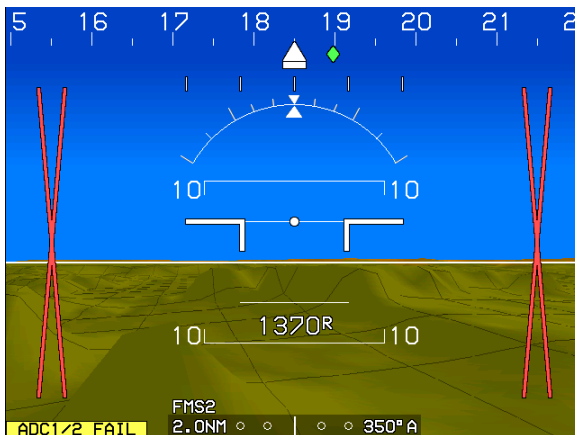
Figure 2-15: Altitude Display Single System ADC Failure (Red X's Only)
