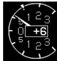
VSI bug set to +1,000 fpm without autopilot enabled
