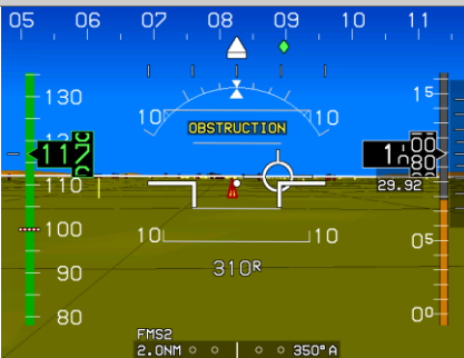
PFD SVS TAWS with Obstruction Caution (Obstruction depictions on PFD and map highlighted but do not flash)
