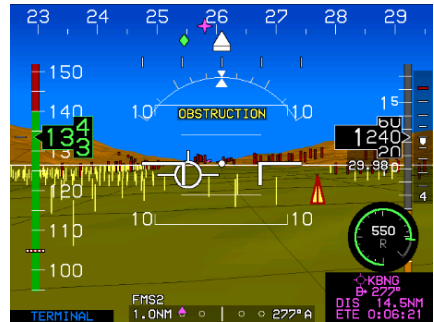
Obstructions creating an OBSTRUCTION caution
