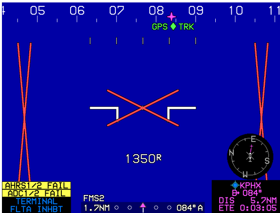
Figure 5-19: PFD Failure Mode 6 ADC and AHRS Failed; GPS/SBAS Normal
