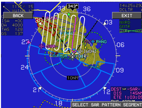
Figure SAR-5: Rising Ladder Pattern-Individual Leg Selected
