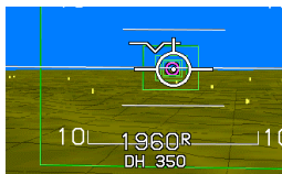
(SVS TAWS) AGL Based on Radar Altimeter
