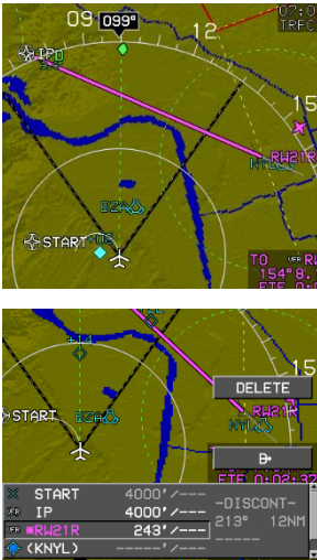
Figure 7-11: Navigating to FAF on VTF VFR Approach
