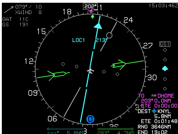
Figure 3-93: HSI Display Air Data and Groundspeed with Marker Beacon
