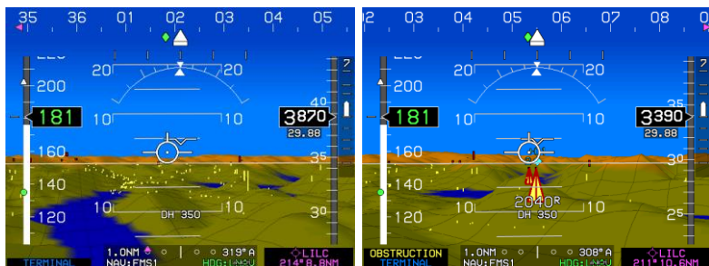
Obstructions without Hazardous Condition
