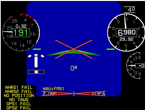
Figure RD-32: PFD (Round Dials) Failure Mode 5 GPS/SBAS and AHRS Failed; ADC Normal
