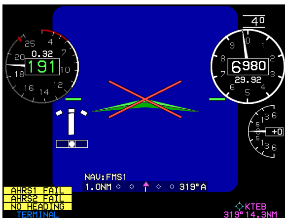
Figure RD-30: PFD (Round Dials) Failure Mode 3 AHRS Failed; GPS/SBAS and ADC Normal
