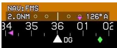
Figure RD-18: Heading Indicator when AHRS in DG Mode
