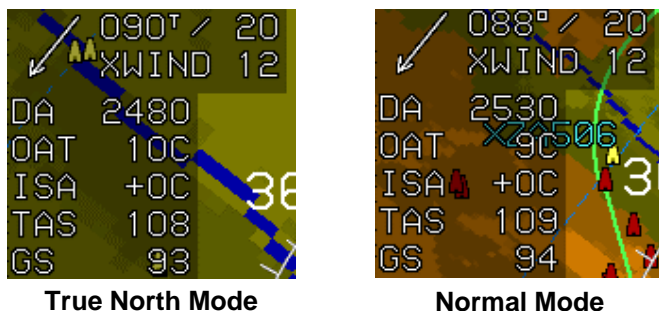
Figure 3-72: Air Data and Groundspeed
