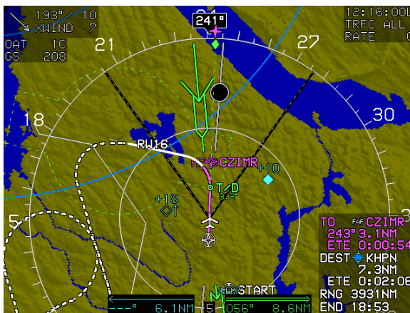
Figure 2-2: IDU-450 Multifunction Display (MFD)
