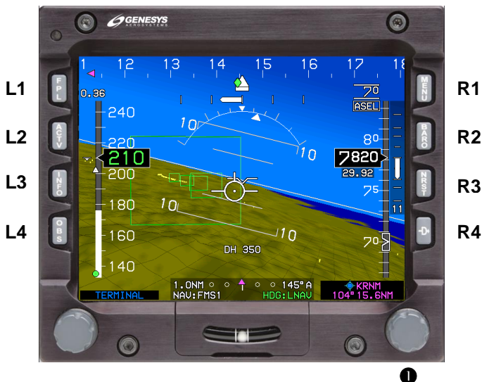
Figure 5-1: IDU-450 Input Controls
