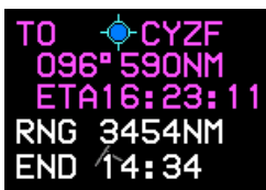
Figure S-4: Fuel Totalizer, Waypoint Bearing/Distance in Lower Right Corner
