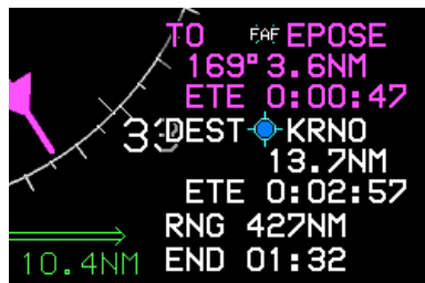
Figure 3-95: Fuel Totalizer/Waypoint Bearing and Distance Functions
