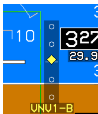
Figure 3-57: Vertical Deviation Indicator Color during GPS/SBAS LON or VLON
