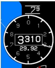
Figure RD-5: Target Altitude Bug (Not Vertically Integrated)
