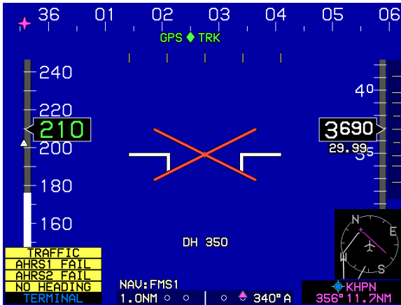
Figure 4-8: PFD Failure Mode 3 AHRs Failed; GPS/SBAS and ADC Normal
