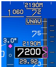
Figure 3-10: Altitude Display (Metric Units)
