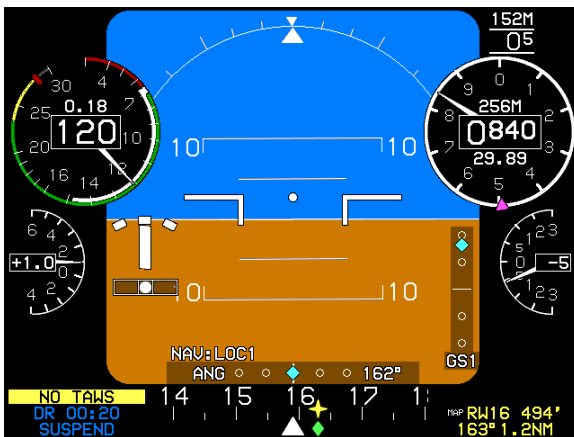
Figure RD-28: PFD (Round Dials) Failure Mode 1 GPS/SBAS Failed; ADC and AHRS Normal
