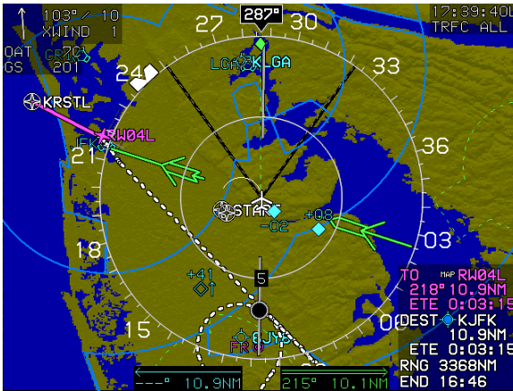
Figure 3-67: Moving Map with Instrument Approach
