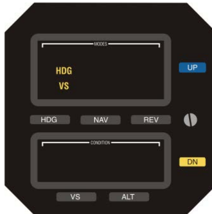
Fig. 3-8. AP Display, HDG and VS Modes Engaged
