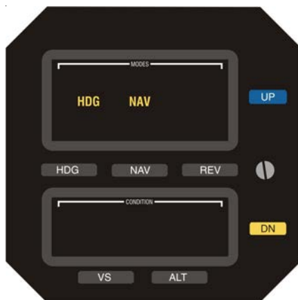
Fig. 3-6. AP Display, HDG Mode Engaged, NAV Mode Armed
