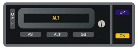
Fig. 3-2. AP Display, ALT HOLD Mode Engaged
