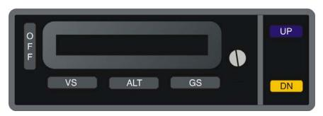
Fig. 2-2. AP Display, All Annunciations Extinguished
