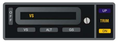
Fig. 2-5. AP Display, VS Mode Engaged, TRIM Required
