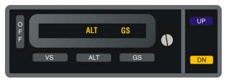
Fig. 3-6. AP Display, ALT HOLD Mode Engaged, GS Mode Armed
