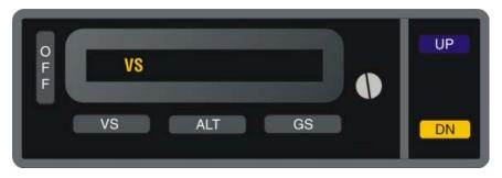
Fig. 3-1. AP Display, VS Mode Engaged
