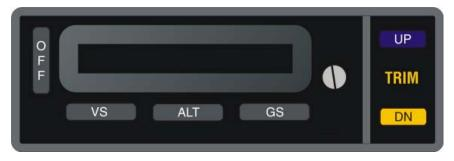
Fig. 3-4. AP Display, Manual Electric Trim in Progress
