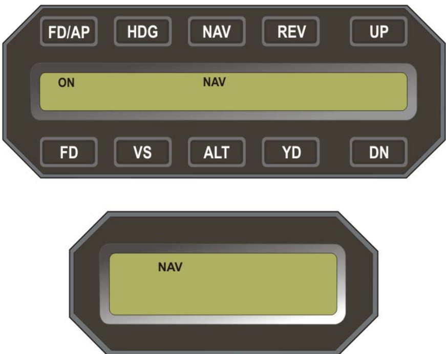
Fig. 3-29. AP Display, NAV Mode Engaged, Before VOR Front Course Intercept
