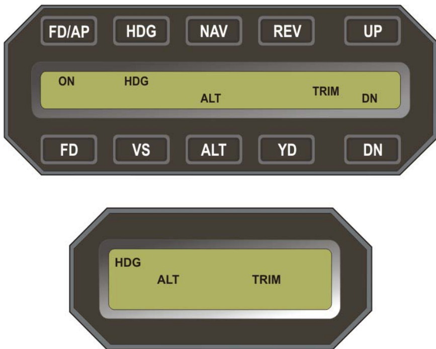
Fig. 3-10. AP Display, TRIM DN Required
