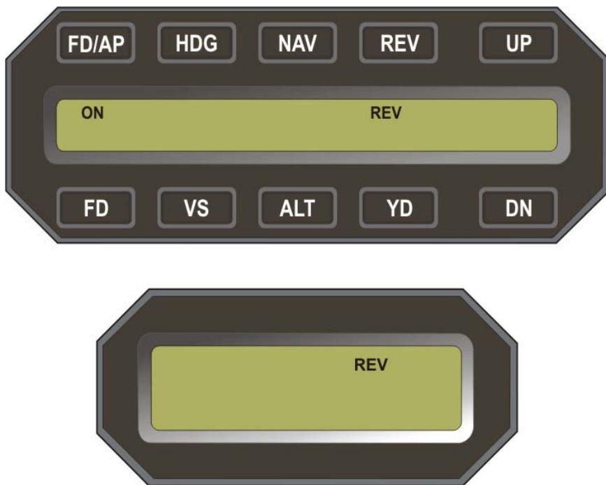
Fig. 3-37. AP Display, REV Mode Engaged, Before VOR Front Course Intercept
