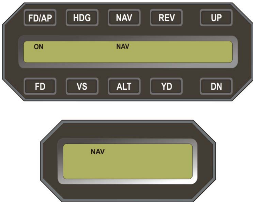
Fig. 3-39. AP Display, NAV Mode Engaged, Before VOR Front Course Intercept
