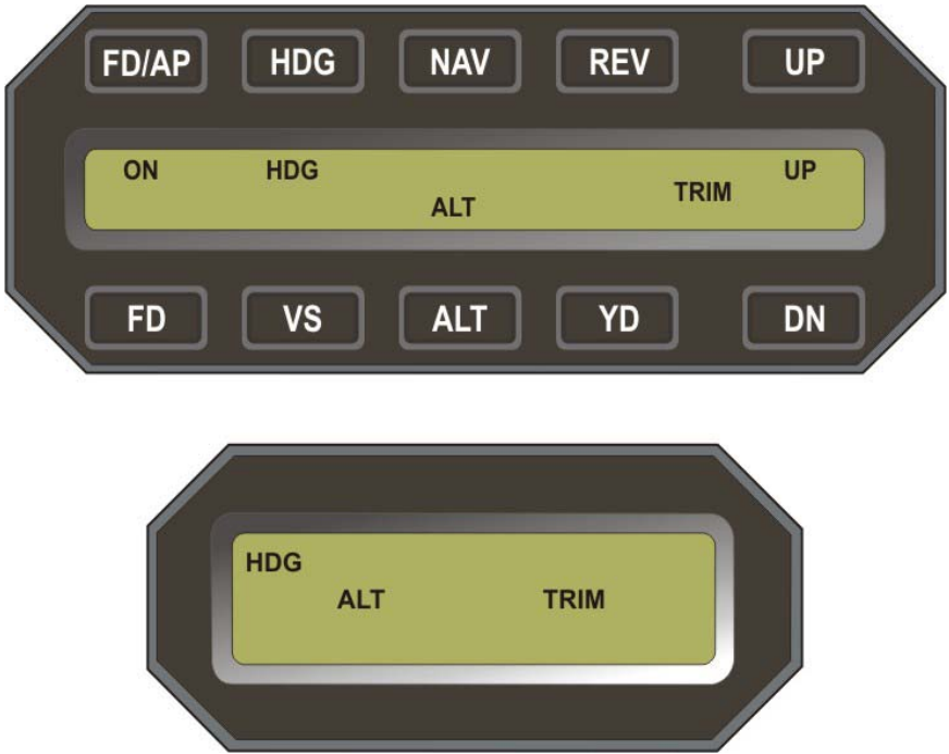
Fig. 3-9. AP Display, TRIM UP Required
