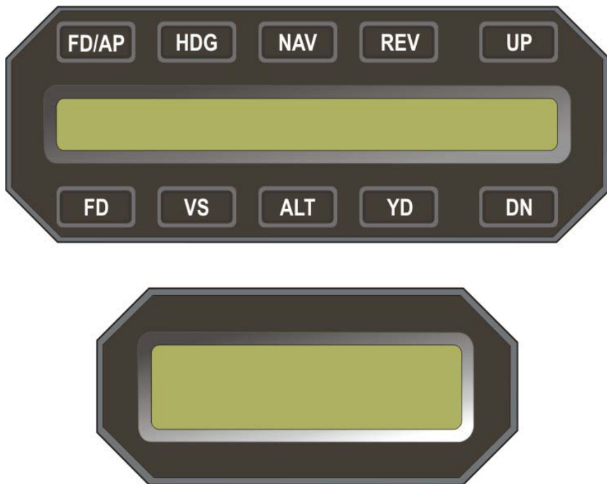
Fig. 2-2. AP Display, Turn Coordinator Failure, RDY Does Not Appear
