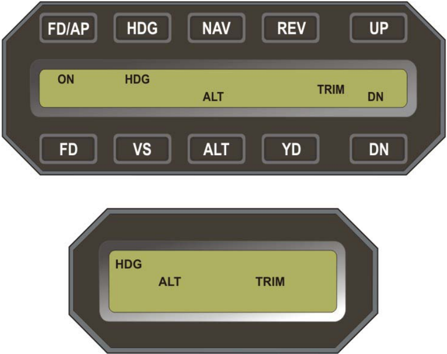
Fig. 2-9. AP Display, HDG and ALT HOLD Modes Engaged, TRIM DN Required
