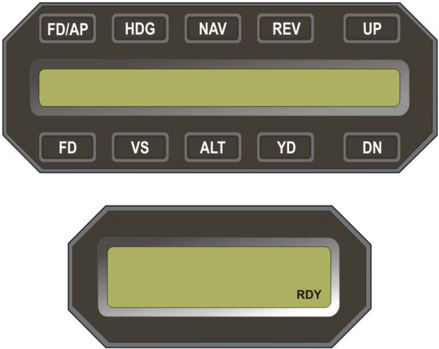
Fig. 2-1. AP Display, RDY for Operation
