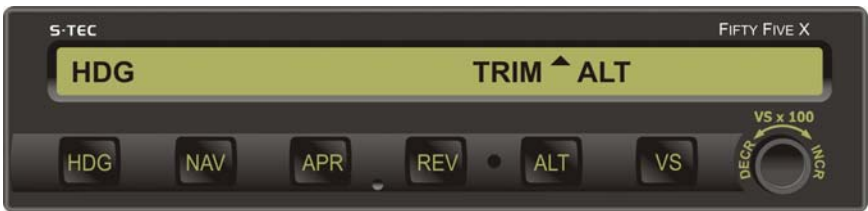
Fig. 3-18. AP Display, HDG and ALT HOLD Modes Engaged, Autotrim in Progress
