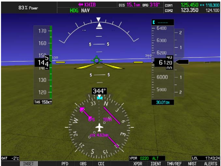
Fig. 3-9. PFD Display, HDG Mode Engaged, NAV Mode Armed
