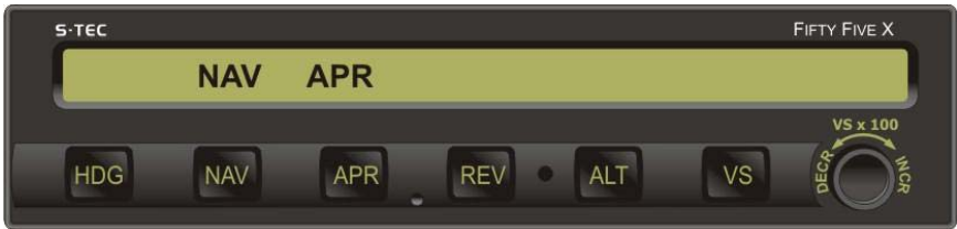
Fig. 3-29. AP Display, NAV APR Mode Engaged, Track LOC Back Course Outbound
