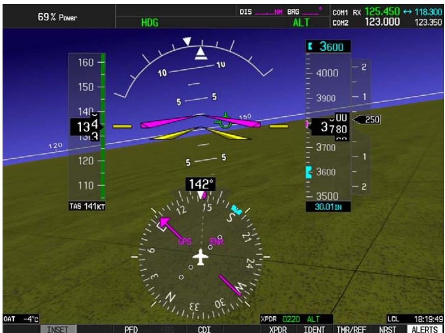
Fig. 3-44. PFD Display, AP Mode Engaged
