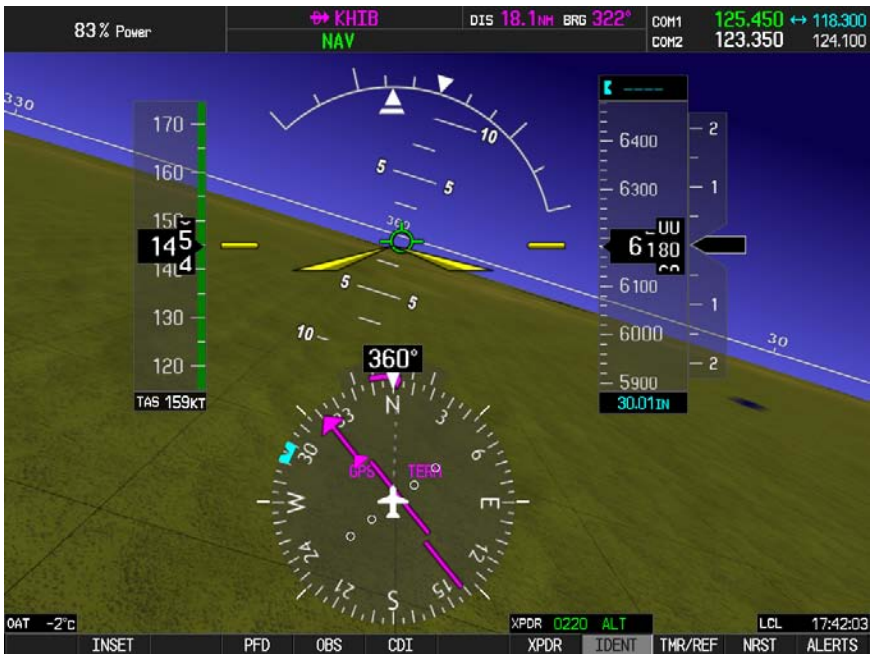
Fig. 3-5. PFD Display, NAV Mode Engaged, A/C Turning onto Course
