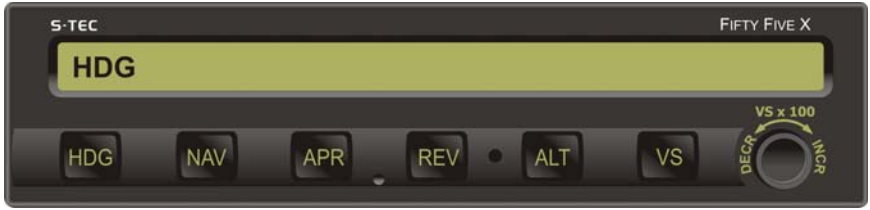
Fig. 2-5. AP Display, HDG Mode Engaged (Pre-Flight)
