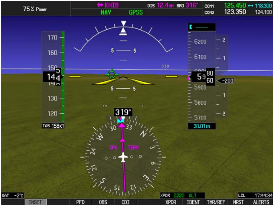
Fig. 3-11. PFD Display, NAV GPSS Mode Engaged
