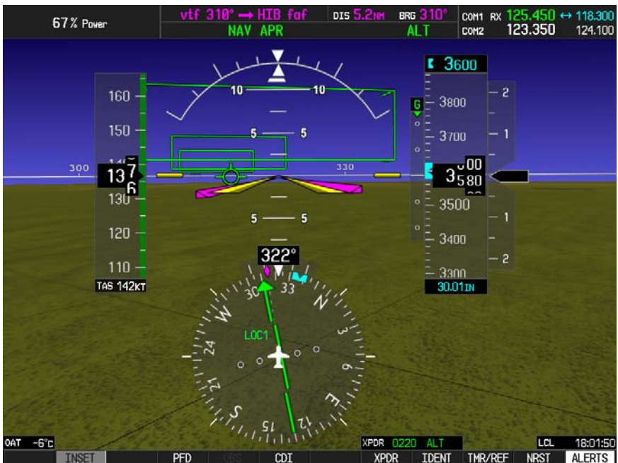
Fig. 3-20. PFD Display, NAV APR and ALT HOLD Modes Engaged
