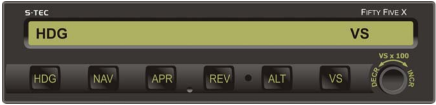
Fig. 2-7. AP Display, HDG and VS Modes Engaged (Pre-Flight)
