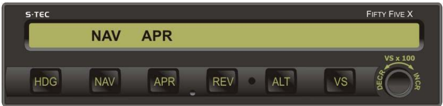
Fig. 3-39. AP Display, NAV APR Mode Engaged, Track VOR Course
