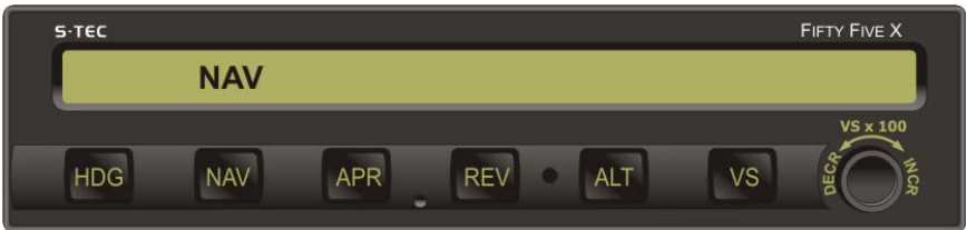
Fig. 3-3. AP Display, NAV Mode Engaged
