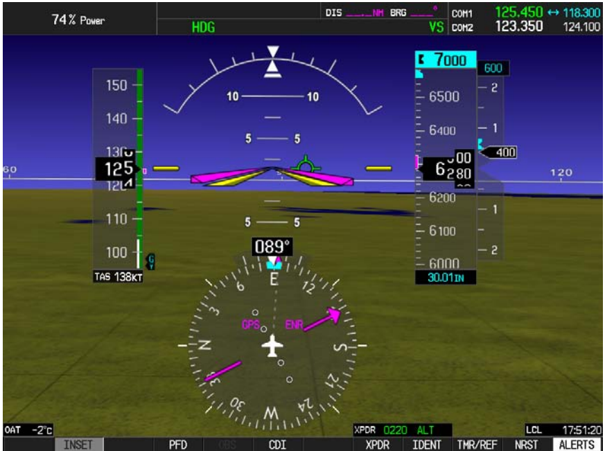
Fig. 3-17. PFD Display, HDG and VS Modes Engaged
