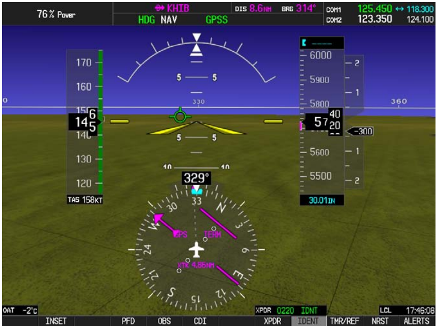
Fig. 3-13. PFD Display, HDG Mode Engaged, NAV GPSS Mode Armed
