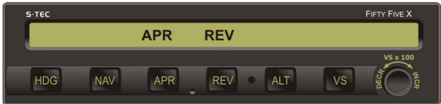
Fig. 3-34. AP Display, REV APR Mode Engaged, Track LOC Front Course Outbound
