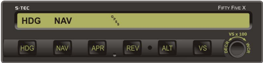
Fig. 3-12. AP Display, HDG Mode Engaged, NAV GPSS Mode Armed
