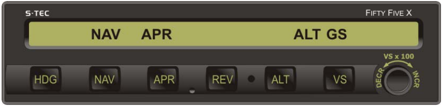
Fig. 3-21. AP Display, NAV APR and ALT HOLD Modes Engaged, GS Mode Armed
