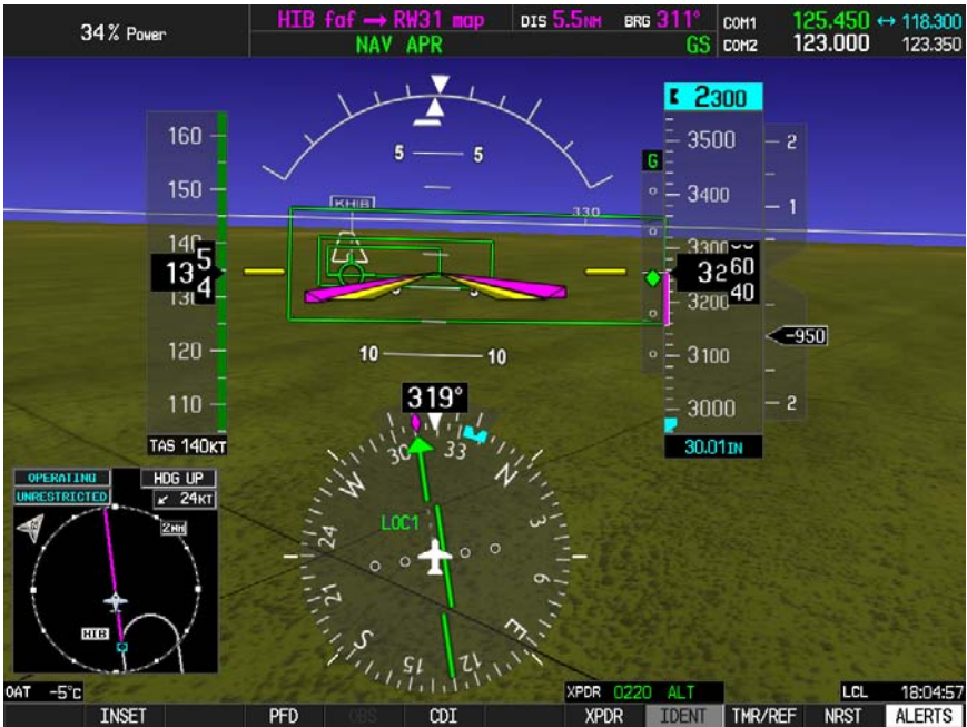
Fig. 3-23. AP Display, NAV APR and GS Modes Engaged
