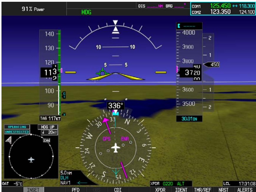
Fig. 3-1. AP Display, HDG Mode Engaged
