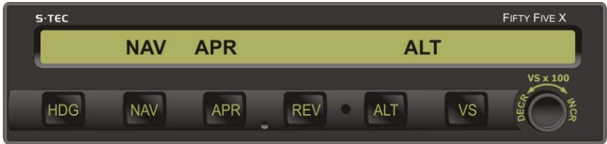
Fig. 3-19. AP Display, NAV APR and ALT HOLD Modes Engaged
