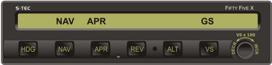
Fig. 3-23. AP Display, NAV APR and GS Modes Engaged
