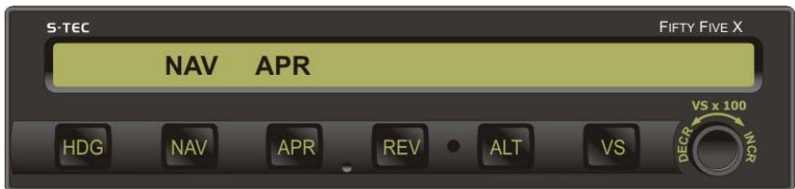
Fig. 3-35. AP Display, NAV APR Mode Engaged, Track LOC Front Course Inbound
