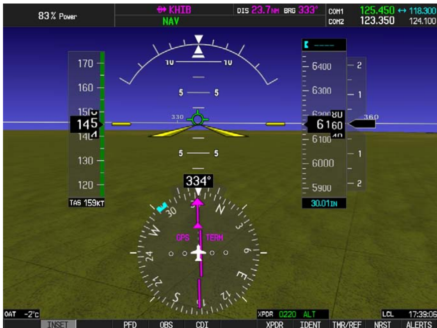
Fig. 3-6. PFD Display, NAV Mode Engaged, A/C Tracking Course
