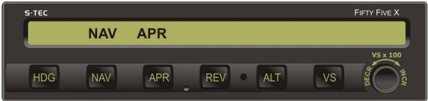
Fig. 3-32. AP Display, NAV APR Mode Engaged, Track LOC Front Course Inbound
