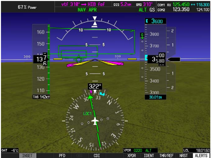
Fig. 3-21. AP Display, NAV APR and ALT HOLD Modes Engaged, GS Mode Armed
