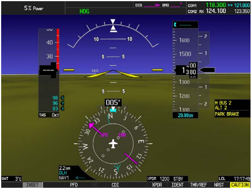
Fig. 2-5. AP Display, HDG Mode Engaged (Pre-Flight)
