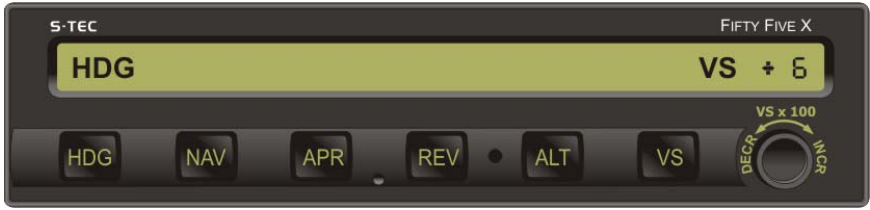
Fig. 3-16. AP Display, HDG and VS Modes Engaged
