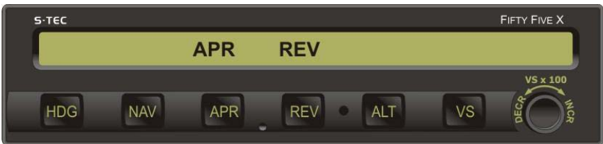
Fig. 3-30. AP Display, REV APR Mode Engaged, Track LOC Back Course Inbound
