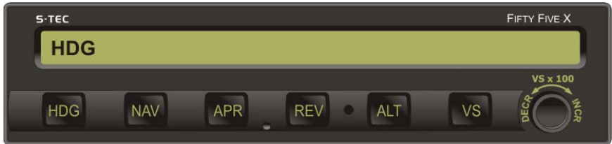
Fig. 3-1. AP Display, HDG Mode Engaged
