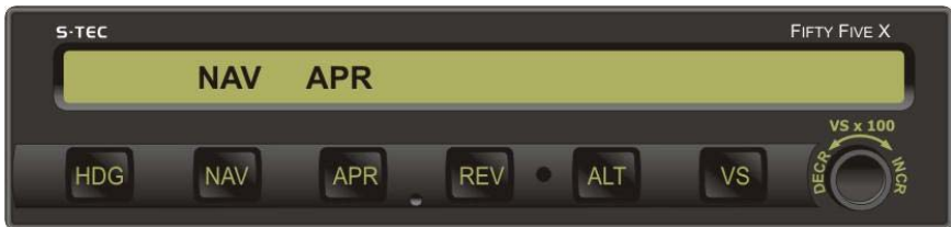
Fig. 3-37. AP Display, NAV APR Mode Engaged, Track VOR Course
