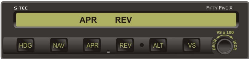
Fig. 3-26. AP Display, REV APR Mode Engaged, Back Course
