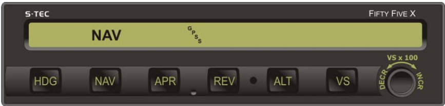
Fig. 3-10. AP Display, NAV GPSS Mode Engaged
