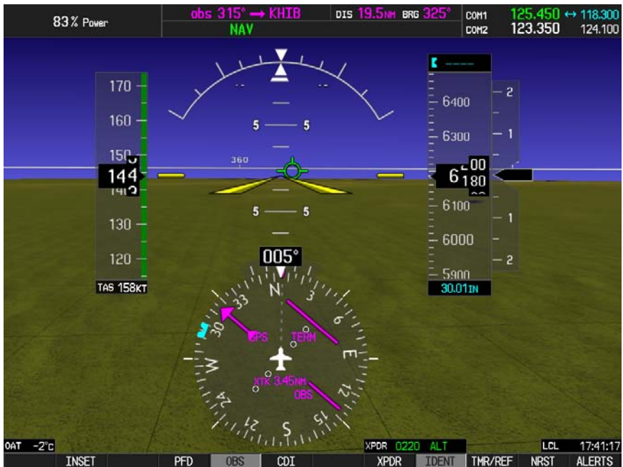
Fig. 3-4. PFD Display, NAV Mode Engaged, A/C on 45° Intercept Angle
