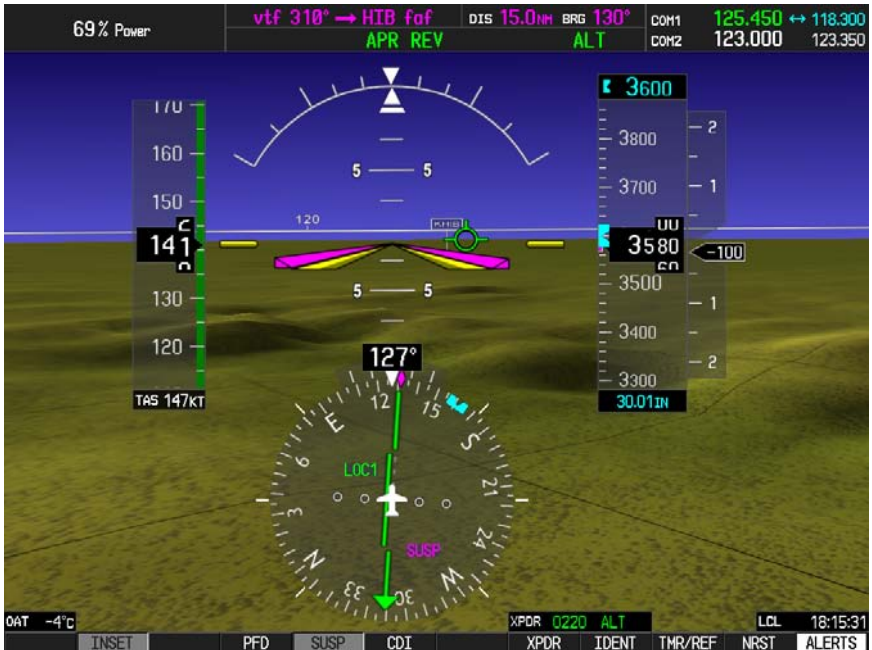
Fig. 3-27. PFD Display, REV APR Mode Engaged, Back Course
