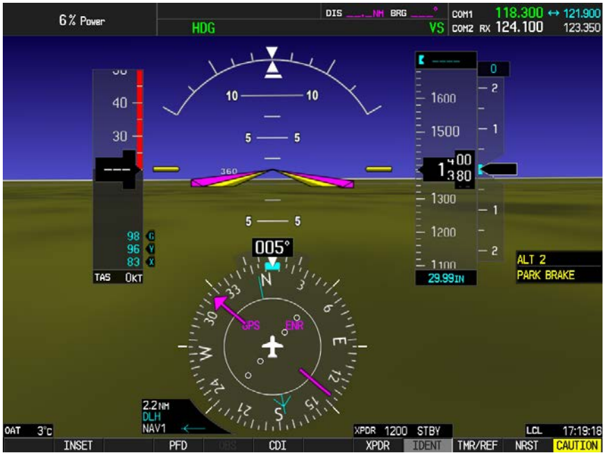
Fig. 2-7. AP Display, HDG and VS Modes Engaged (Pre-Flight)
