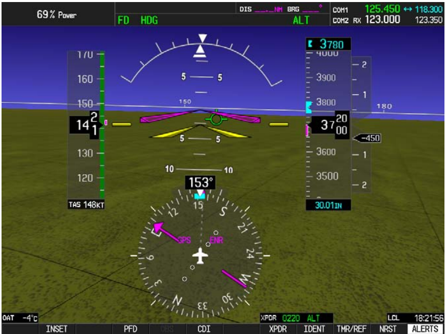
Fig. 3-45. PFD Display, FD Mode Engaged
