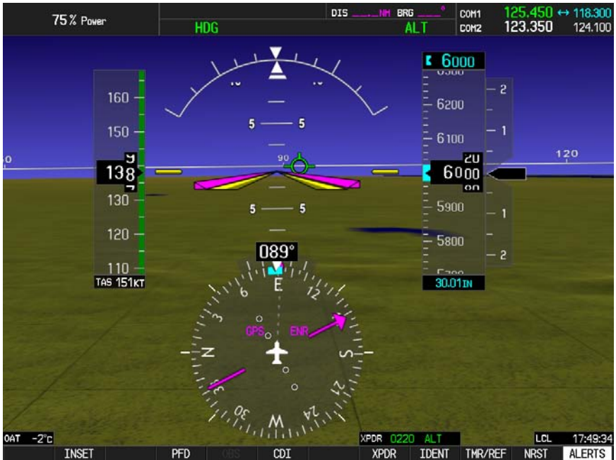
Fig. 3-15. PFD Display, HDG and ALT HOLD Modes Engaged
