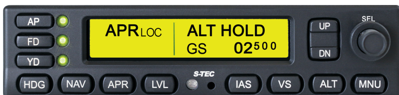
Figure 3-18: APR LOC and ALT HOLD Modes Engaged, GS Mode Armed
