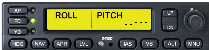
Figure 3-38: FD Mode Engaged, AP Mode Disengaged
