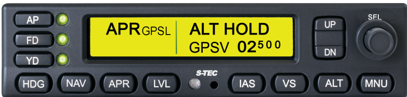
Figure 3-31: GPS and Pitch Modes Engaged, Approach ALT HOLD Mode
