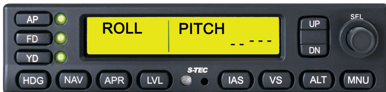
Figure 3-34: Level Mode, Roll and Pitch Hold Modes
