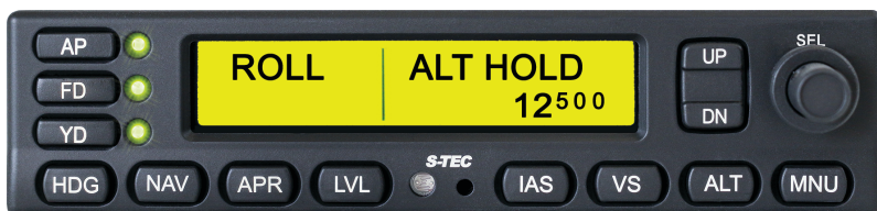
Figure 3-11: Altitude Hold (ALT HOLD) Mode
