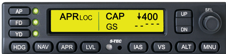
Figure 3-19: APR LOC and GS CAP Modes Engaged
