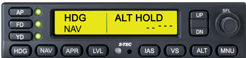
Figure 3-4: Heading Mode Engaged, Navigation Mode Armed
