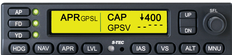
Figure 3-32: GPSV CAP Mode Engaged
