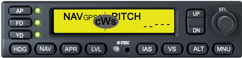
Figure 3-7: Control Wheel Steering (CWS) Mode
