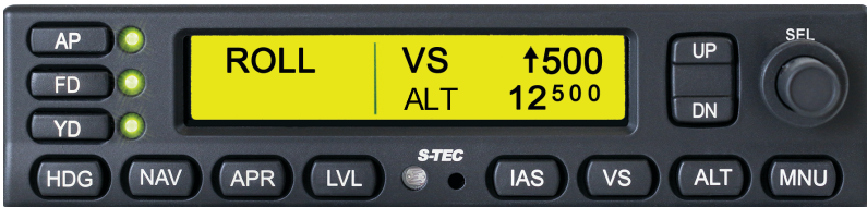
Figure 3-13: Vertical Speed in Units of FPM
