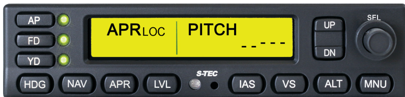
Figure 3-24: APR LOC Mode
