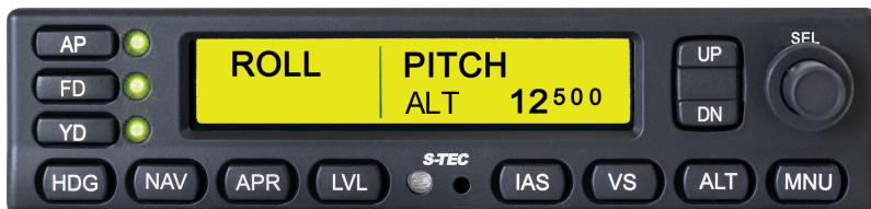
Figure 3-12: Target Altitude in Ft. with ALT HOLD Mode Armed
