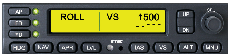
Figure 3-10: Vertical Speed (VS) Mode
