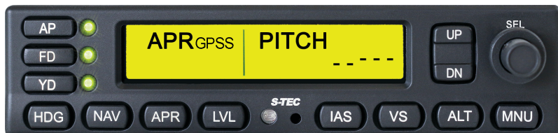
Figure 3-30: GPSS and Pitch Modes Engaged
