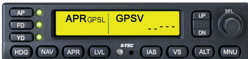
Figure 3-33: GPSV Mode Engaged
