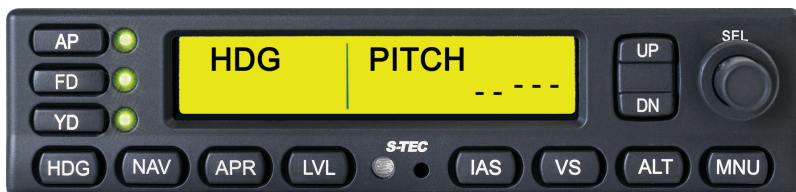
Figure 3-2: Heading (HDG) Mode
