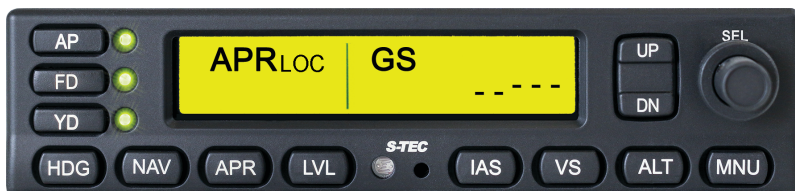
Figure 3-20: APR LOC and GS Modes Engaged
