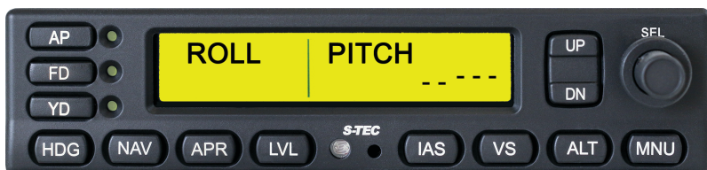
Figure 3-36: YD Mode Disengaged
