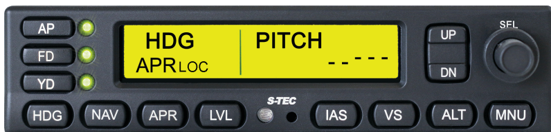
Figure 3-28: APR LOC Mode Armed
