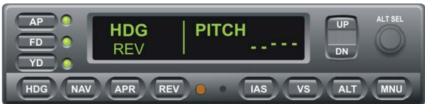
Fig. 3-40. AP Display, HDG Mode Engaged, REV Mode Armed
