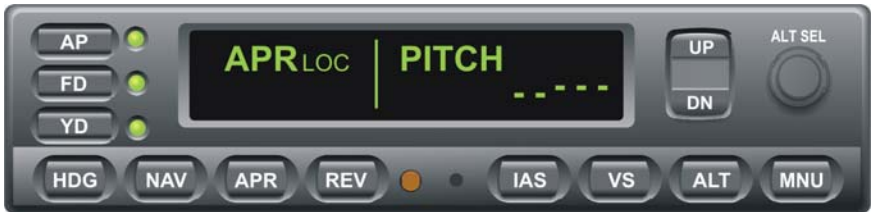
Fig. 3-49. AP Display, APR LOC Mode Engaged, Track LOC Front Course Inbound
