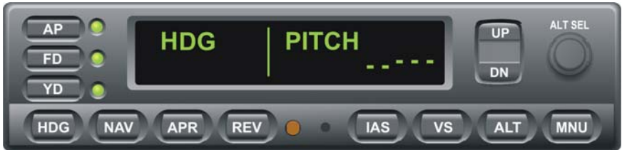
Fig. 3-47. AP Display, HDG Mode Engaged, A/C on Procedure Turn
