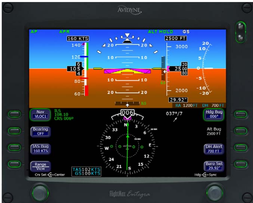
Fig. 3-30. PFD Display, APR LOC and ALT HOLD Modes Engaged, GS Mode Armed
