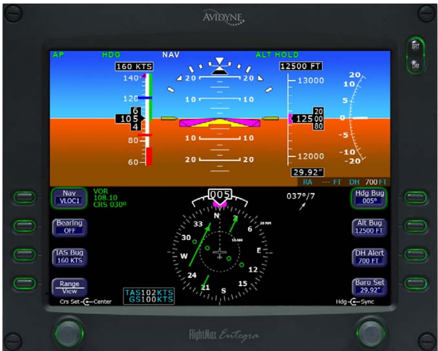
Fig. 3-10. PFD Display, HDG and ALT HOLD Modes Engaged, NAV Mode Armed
