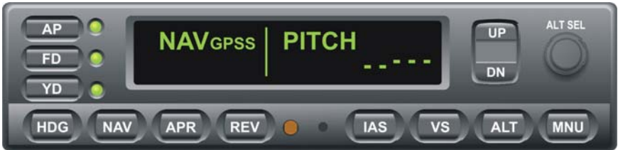
Fig. 3-11. AP Display, GPSS and PITCH Modes Engaged
