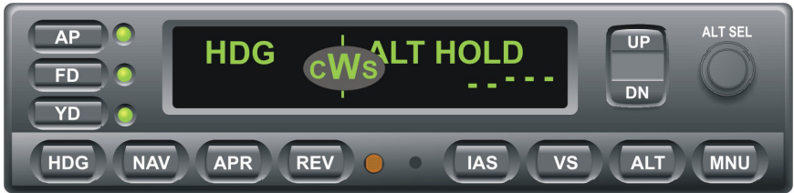
Fig. 2-20. AP Display, CWS Mode Engaged (Pre-Flight)
