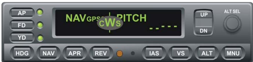
Fig. 3-13. AP Display, CWS Mode Engaged
