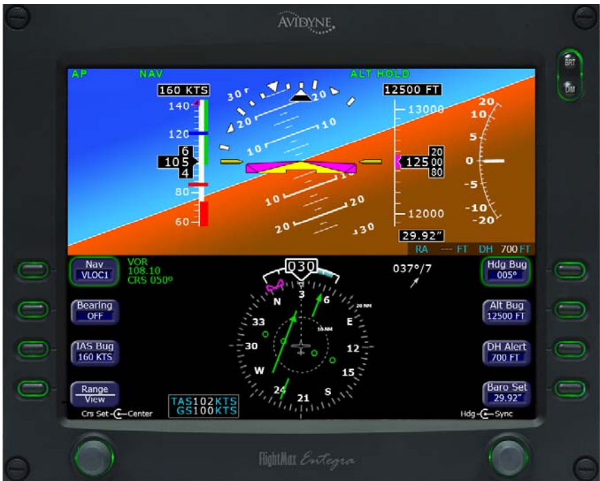
Fig. 3-7. PFD Display, NAV and ALT HOLD Modes Engaged, A/C Turning onto Course
