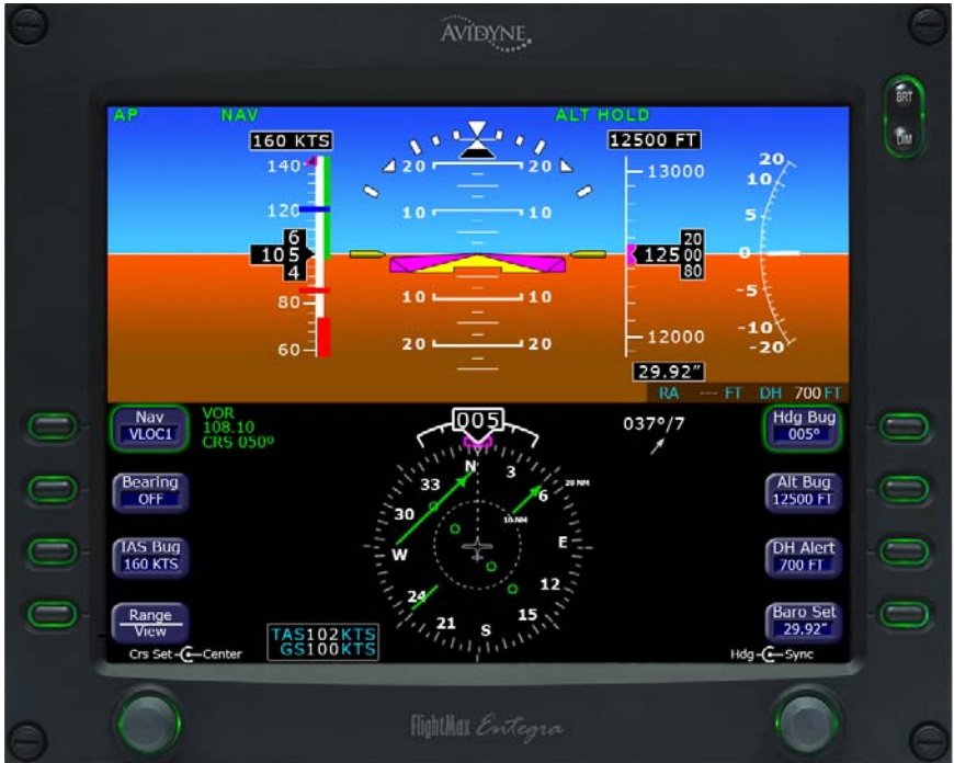
Fig. 3-6. PFD Display, NAV and ALT HOLD Modes Engaged, A/C on 45° Intercept Angle
