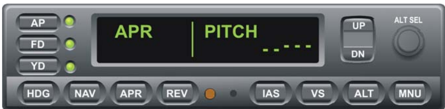
Fig. 3-45. AP Display, APR Mode Engaged, Track VOR Course
