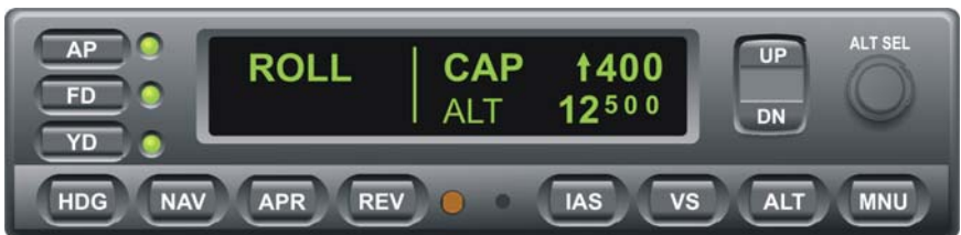
Fig. 3-24. AP Display, ROLL and ALT HOLD CAP Modes Engaged
