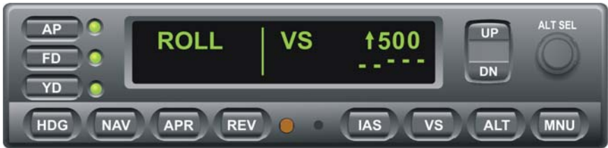
Fig. 3-18. AP Display, ROLL and VS Modes Engaged
