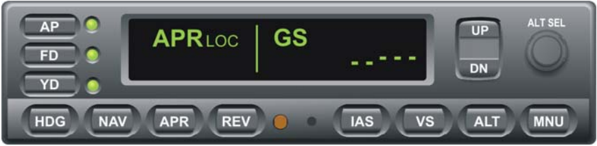
Fig. 3-32. AP Display, APR LOC and GS Modes Engaged
