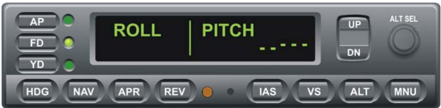
Fig. 3-64. AP Display, FD Mode Engaged, AP Mode Disengaged
