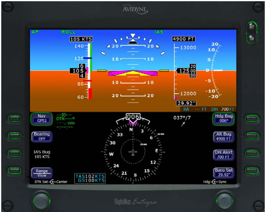
Fig. 3-17. PFD Display, ROLL and IAS Modes Engaged
