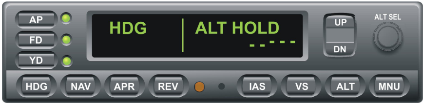
Fig. 2-18. AP Display, HDG and ALT HOLD Modes Engaged (Pre-Flight)
