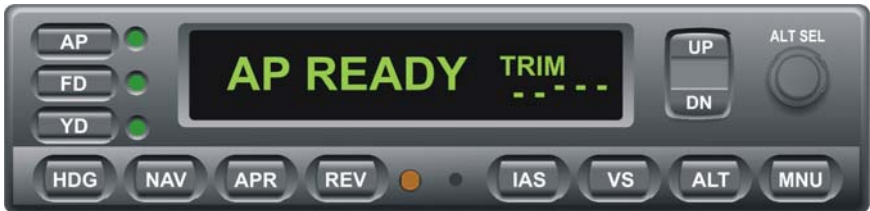
Fig. 3-28. AP Display, MANUAL ELECTRIC TRIM in Progress
