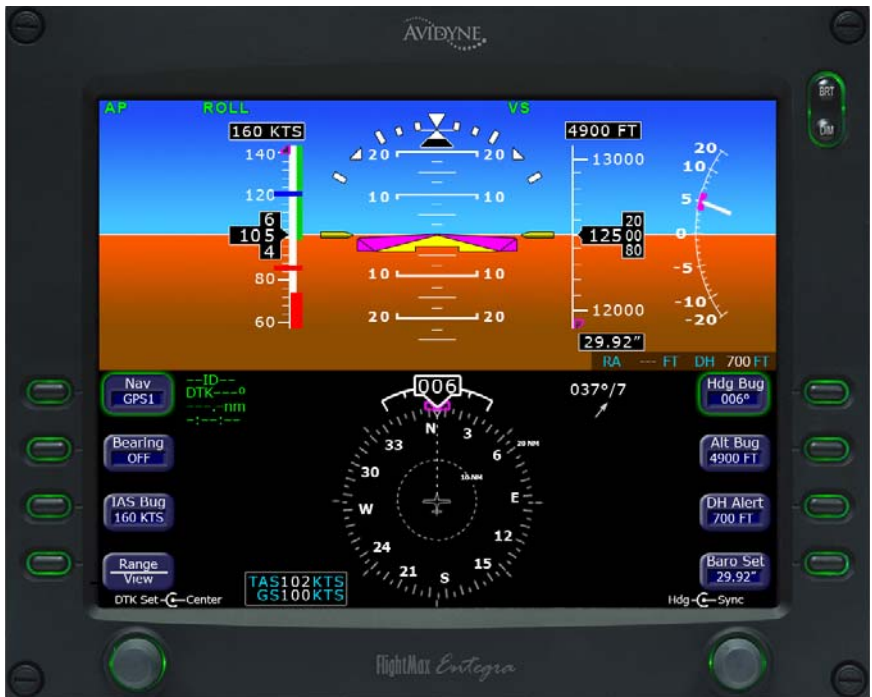
Fig. 3-19. PFD Display, ROLL and VS Modes Engaged
