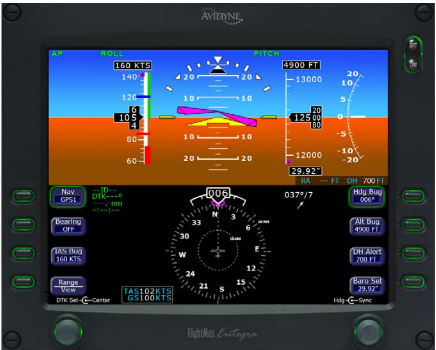
Fig. 3-63. PFD Display, Magenta Steering Command Bars
