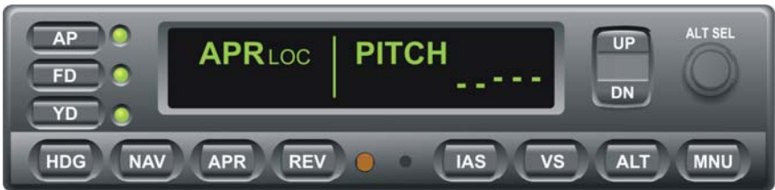
Fig. 3-38. AP Display, APR LOC Mode Engaged, Track LOC Back Course Outbound
