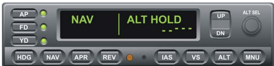
Fig. 3-5. AP Display, NAV and ALT HOLD Modes Engaged
