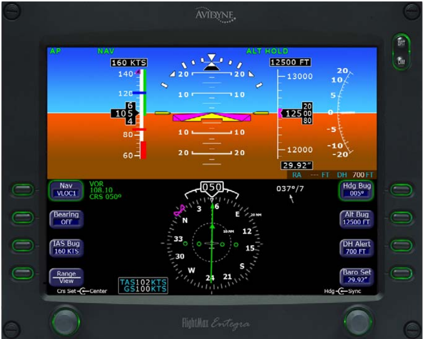
Fig. 3-8. PFD Display, NAV and ALT HOLD Modes Engaged, A/C Tracking Course
