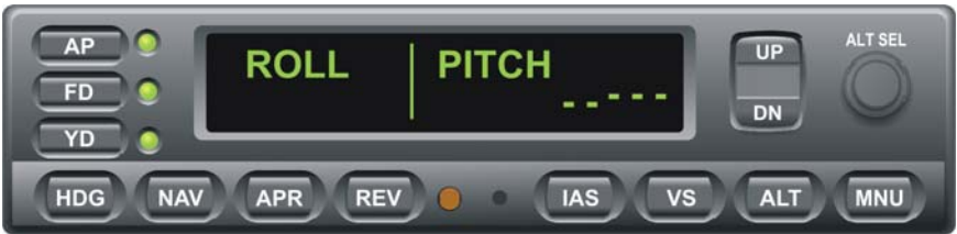
Fig. 3-62. AP Display, AP and FD Modes Engaged
