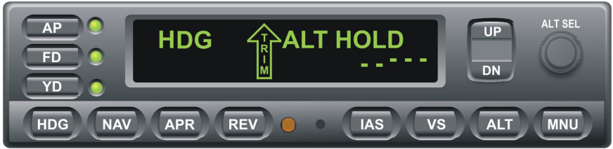
Fig. 2-24. AP Display, AUTO TRIM UP in Progress (Pre-Flight)
