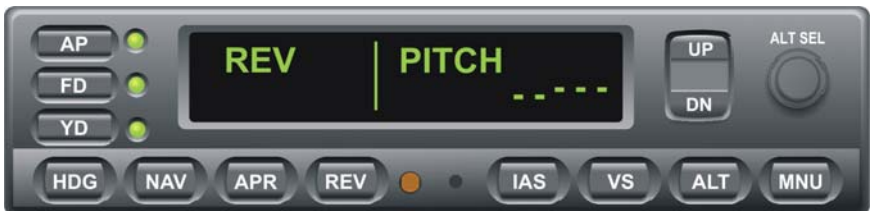
Fig. 3-41. AP Display, REV Mode Engaged, Track LOC Back Course Inbound
