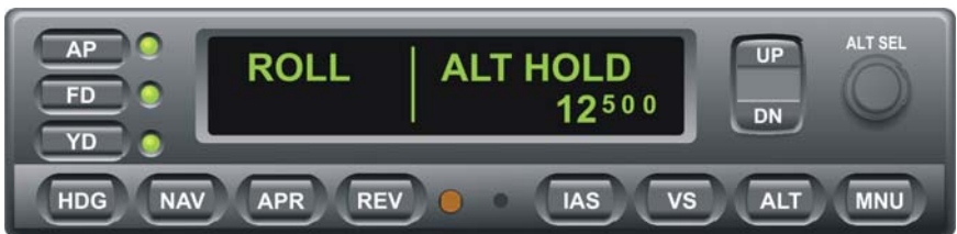
Fig. 3-25. AP Display, ROLL and ALT HOLD Modes Engaged
