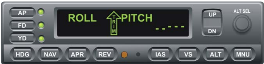
Fig. 3-26. AP Display, AUTO TRIM UP in Progress
