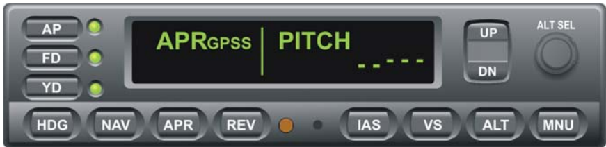
Fig. 3-55. AP Display, GPSS and PITCH Modes Engaged, T Approach
