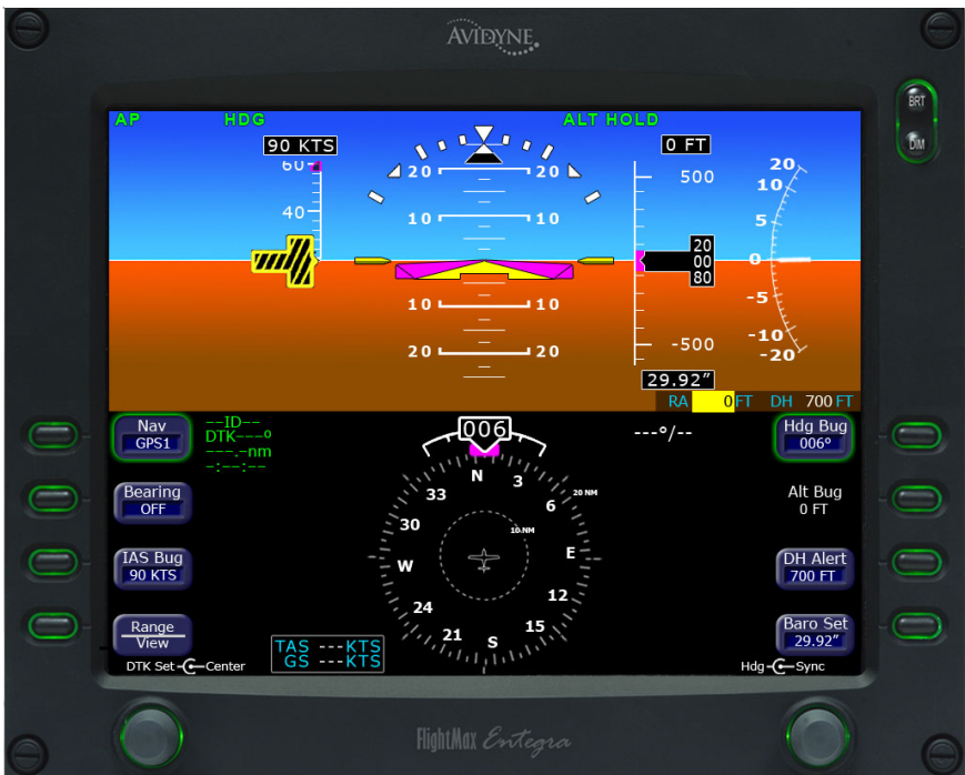
Fig. 2-19. PFD Display, HDG and ALT HOLD Modes Engaged (Pre-Flight)
