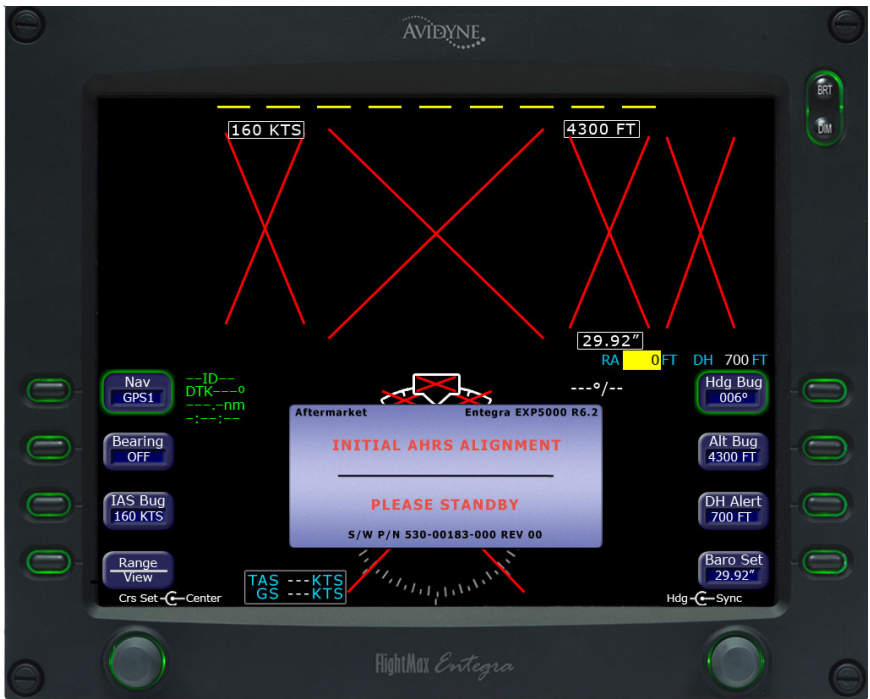
Fig. 2-3. PFD Display, INITIAL AHRS ALIGNMENT
