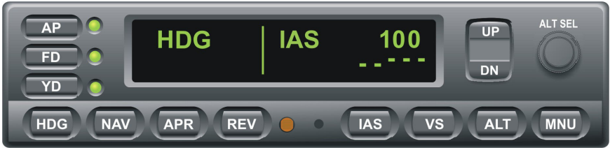
Fig. 2-14. AP Display, HDG and IAS Modes Engaged (Pre-Flight)
