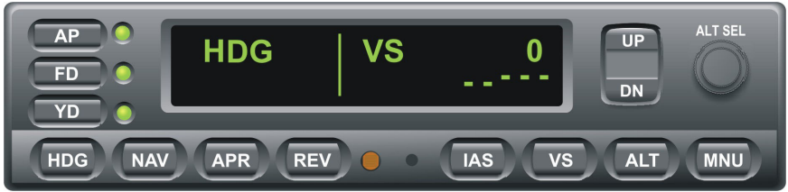
Fig. 2-16. AP Display, HDG and VS Modes Engaged (Pre-Flight)
