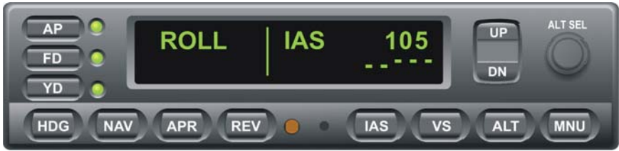
Fig. 3-16. AP Display, ROLL and IAS Modes Engaged
