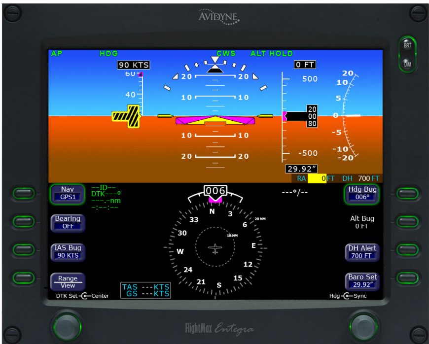
Fig. 2-21. PFD Display, CWS Mode Engaged (Pre-Flight)
