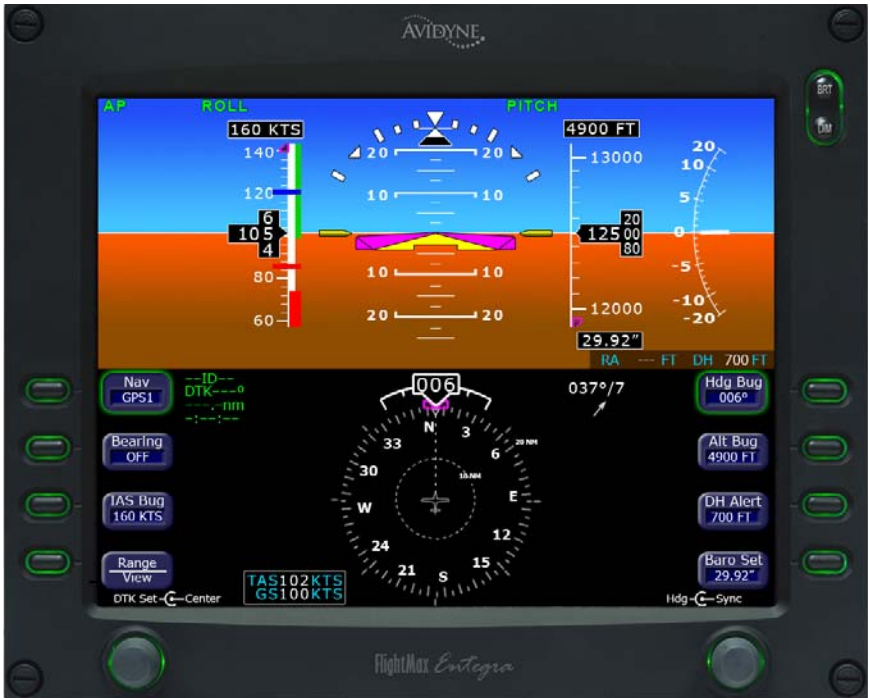
Fig. 3-2. PFD Display, ROLL and PITCH Modes Engaged
