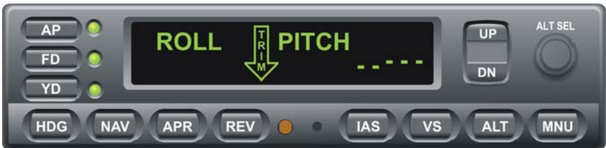
Fig. 3-27. AP Display, AUTO TRIM DN in Progress
