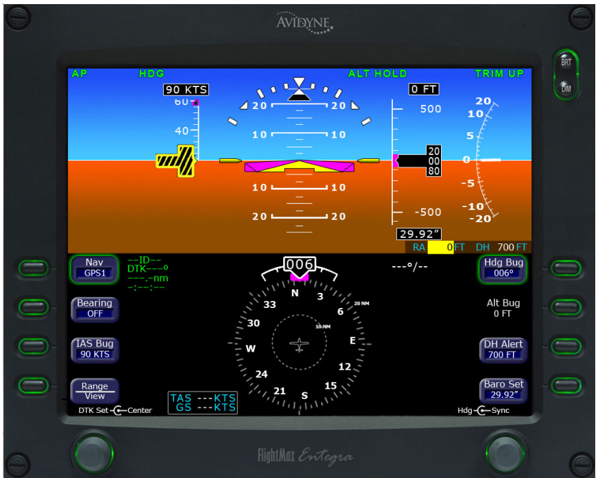
Fig. 2-25. PFD Display, AUTO TRIM UP in Progress (Pre-Flight)
