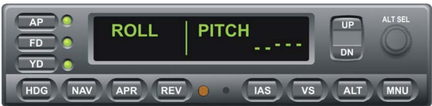
Fig. 3-1. AP Display, ROLL and PITCH Modes Engaged
