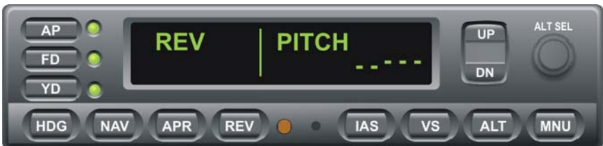
Fig. 3-51. AP Display, REV Mode Engaged, Track Reciprocal VOR Course
