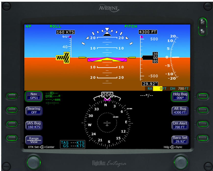
Fig. 2-11. PFD Display, ROLL and PITCH Modes Engaged (Pre-Flight)
