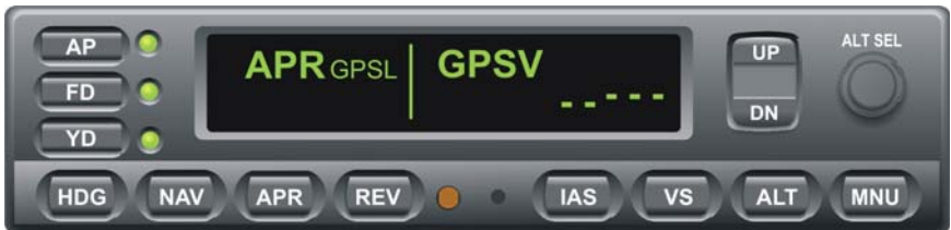
Fig. 3-59. AP Display, APR GPSL and GPSV Modes Engaged
