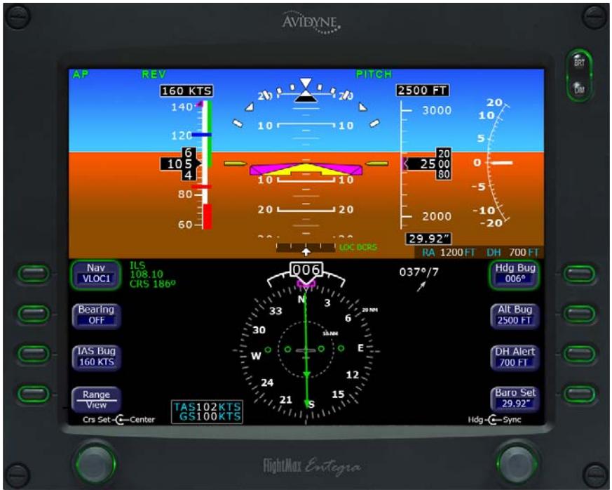
Fig. 3-36. PFD Display, REV Mode Engaged, Track LOC Back Course Inbound
