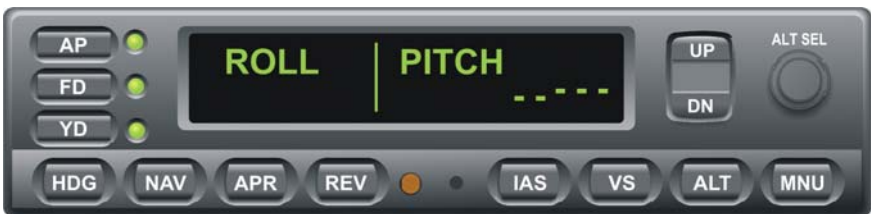
Fig. 3-60. AP Display, YD Mode Engaged
