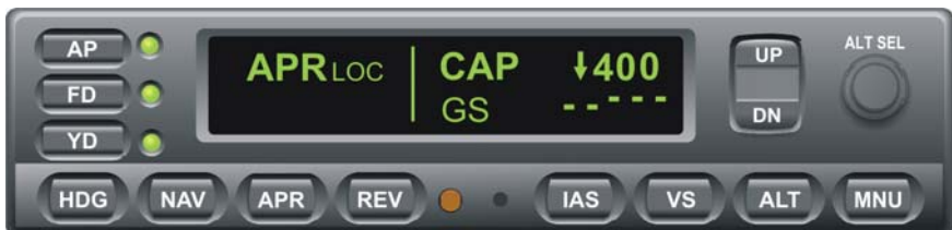
Fig. 3-31. AP Display, APR LOC and GS CAP Modes Engaged
