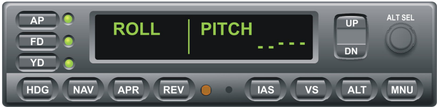
Fig. 2-10. AP Display, ROLL and PITCH Modes Engaged (Pre-Flight)
