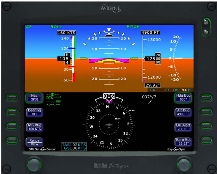
Fig. 3-15. PFD Display, ROLL and PITCH Modes Engaged
