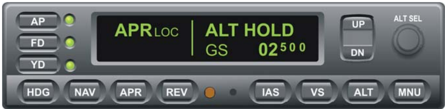
Fig. 3-29. AP Display, APR LOC and ALT HOLD Modes Engaged, GS Mode Armed
