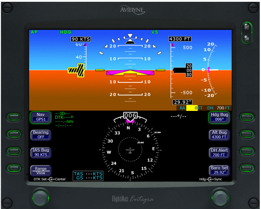
Fig. 2-17. PFD Display, HDG and VS Modes Engaged (Pre-Flight)
