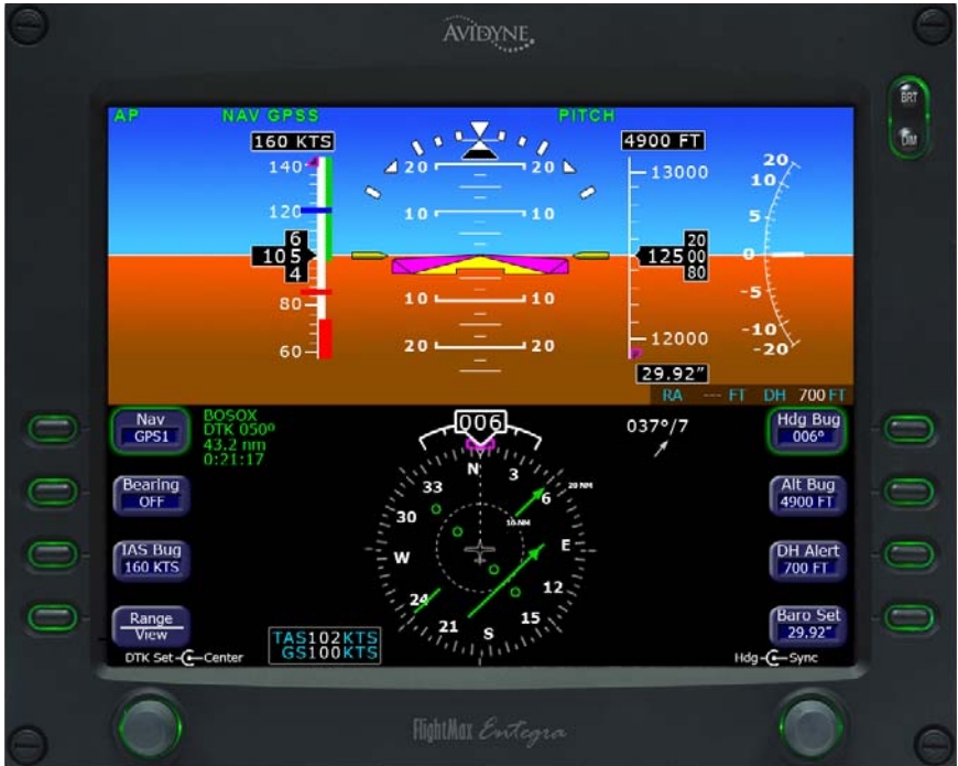
Fig. 3-12. PFD Display, GPSS and PITCH Modes Engaged
