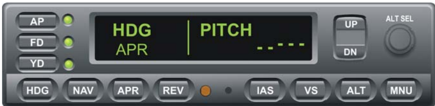
Fig. 3-53. AP Display, HDG Mode Engaged, APR Mode Armed
