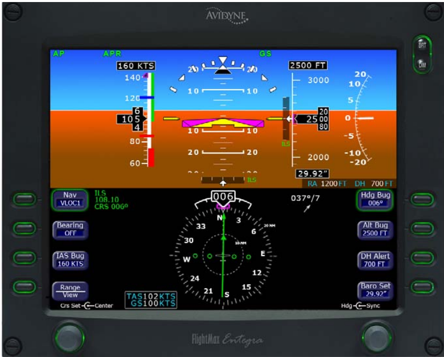
Fig. 3-33. PFD Display, APR LOC and GS Modes Engaged
