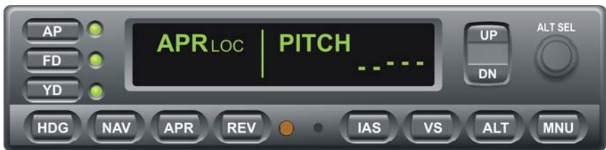
Fig. 3-43. AP Display, APR LOC Mode Engaged, Track LOC Front Course Inbound
