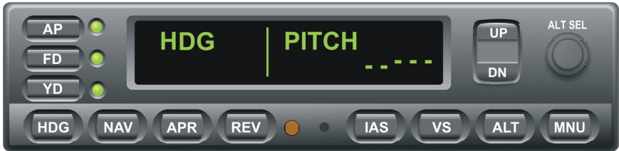
Fig. 2-12. AP Display, HDG and PITCH Modes Engaged (Pre-Flight)
