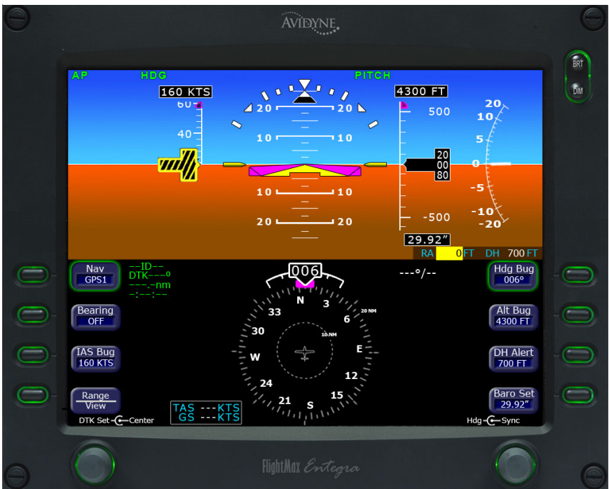
Fig. 2-13. PFD Display, HDG and PITCH Modes Engaged (Pre-Flight)
