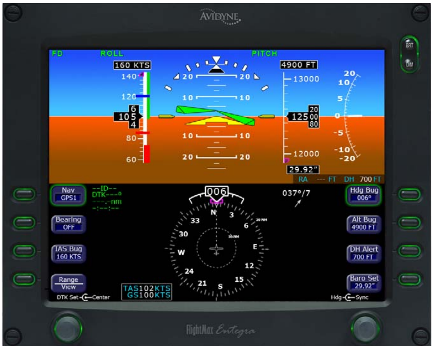
Fig. 3-65. PFD Display, Green Steering Command Bars
