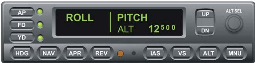
Fig. 3-22. AP Display, ROLL and PITCH Modes Engaged, ALT HOLD Mode Armed
