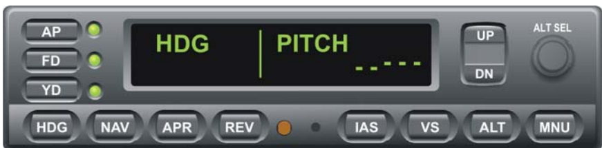
Fig. 3-3. AP Display, HDG and PITCH Modes Engaged
