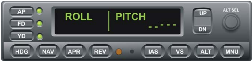
Fig. 3-14. AP Display, ROLL and PITCH Modes Engaged
