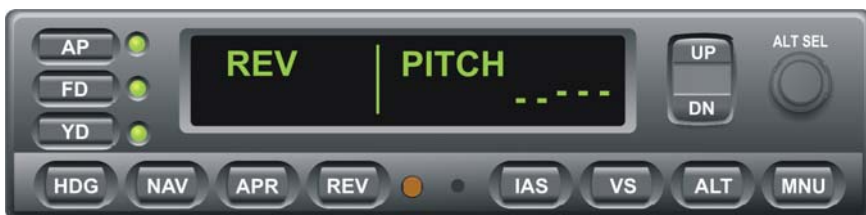
Fig. 3-46. AP Display, REV Mode Engaged, Track LOC Front Course Outbound
