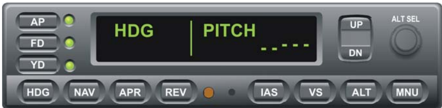
Fig. 3-52. AP Display, HDG Mode Engaged, A/C on Procedure Turn
