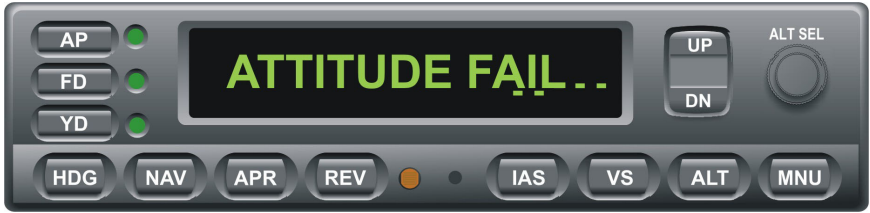
Fig. 2-2. AP Display, INITIAL AHRS ALIGNMENT
