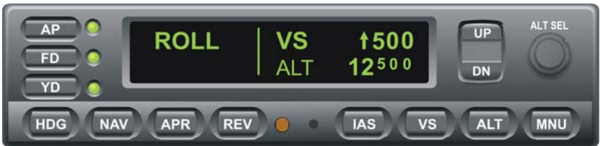
Fig. 3-23. AP Display, ROLL and VS Modes Engaged, ALT HOLD Mode Armed
