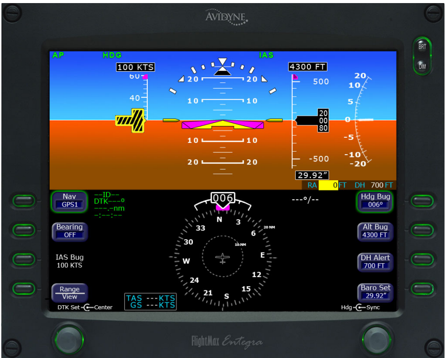
Fig. 2-15. PFD Display, HDG and IAS Modes Engaged (Pre-Flight)
