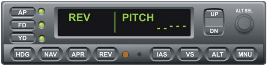
Fig. 3-35. AP Display, REV Mode Engaged, Track LOC Back Course Inbound
