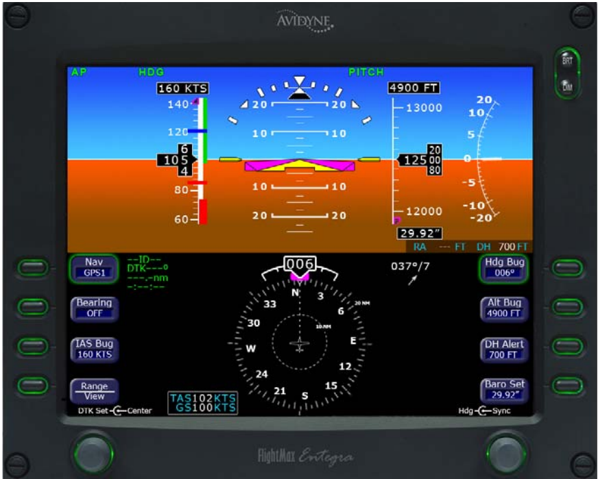
Fig. 3-4. PFD Display, HDG and PITCH Modes Engaged
