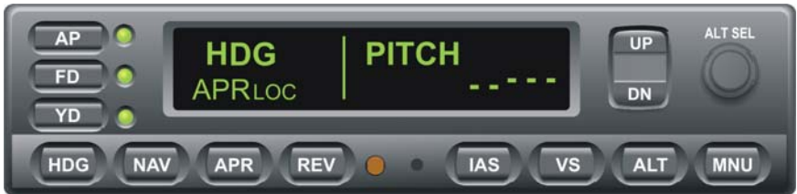
Fig. 3-48. AP Display, HDG Mode Engaged, APR LOC Mode Armed
