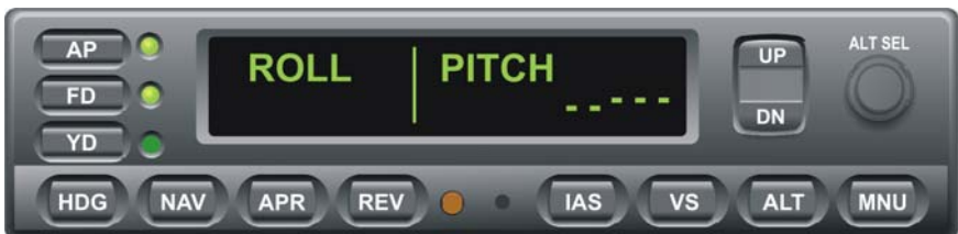
Fig. 3-61. AP Display, YD Mode Disengaged
