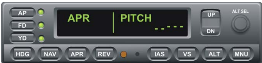
Fig. 3-54. AP Display, APR Mode Engaged, Track VOR Course
