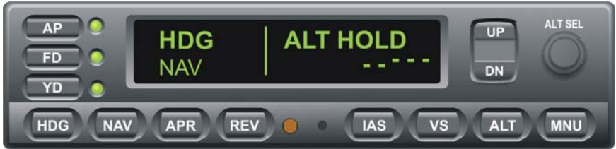
Fig. 3-9. AP Display, HDG and ALT HOLD Modes Engaged, NAV Mode Armed
