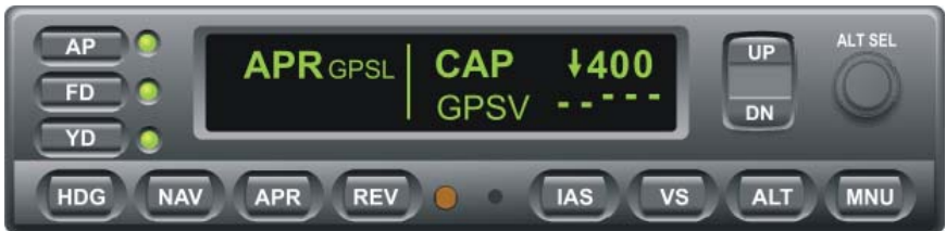
Fig. 3-46. AP Display, APR GPSL and GPSV CAP Modes Engaged
