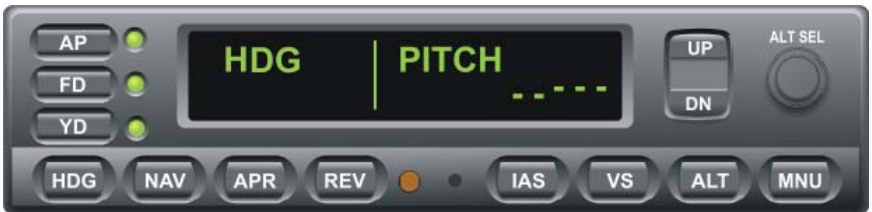
Fig. 3-2. AP Display, HDG and PITCH Modes Engaged
