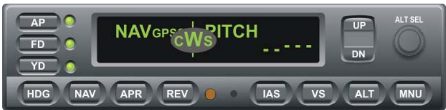
Fig. 3-6. AP Display, CWS Mode Engaged
