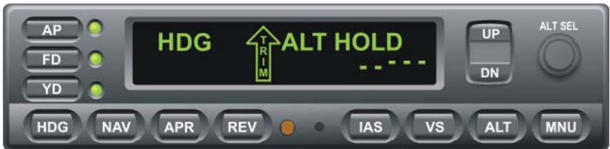
Fig. 2-13. AP Display, AUTO TRIM UP in Progress (Pre-Flight)
