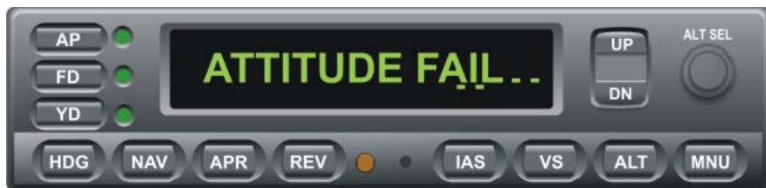
Fig. 2-5. AP Display, ADAHRS Failure
