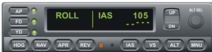
Fig. 3-8. AP Display, ROLL and IAS Modes Engaged
