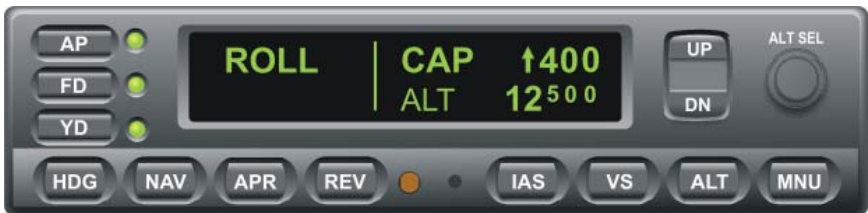
Fig. 3-13. AP Display, ROLL and ALT HOLD CAP Modes Engaged
