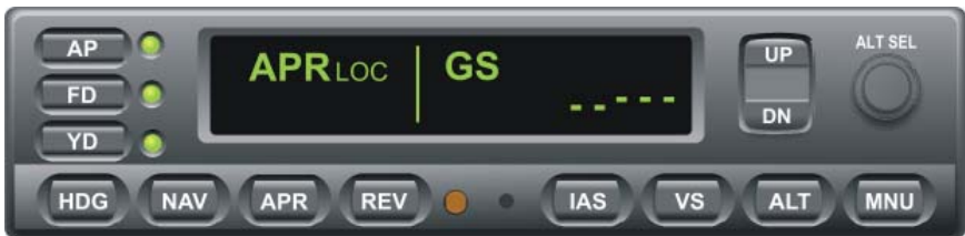
Fig. 3-20. AP Display, APR LOC and GS Modes Engaged
