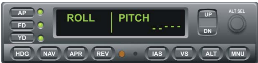
Fig. 3-1. AP Display, ROLL and PITCH Modes Engaged
