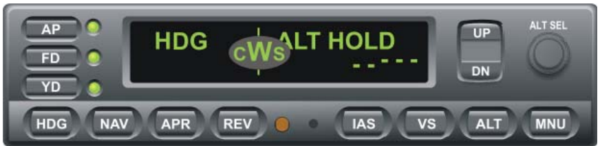
Fig. 2-11. AP Display, CWS Mode Engaged (Pre-Flight)
