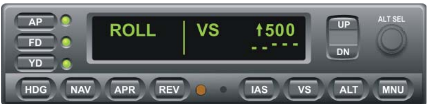
Fig. 3-9. AP Display, ROLL and VS Modes Engaged
