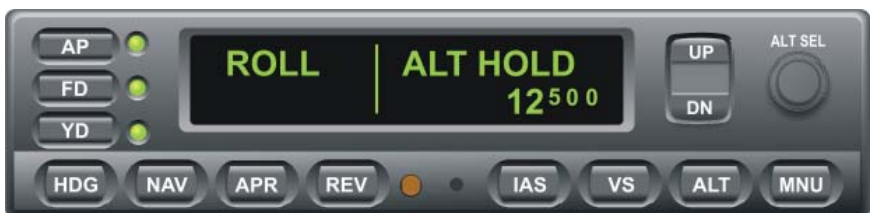
Fig. 3-10. AP Display, ROLL and ALT HOLD Modes Engaged
