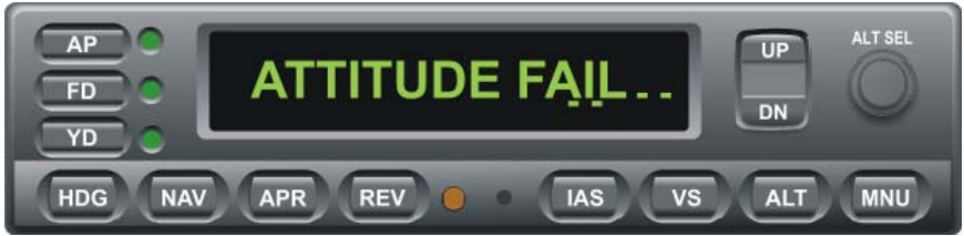
Fig. 2-2. AP Display, INITIAL ADAHRS ALIGNMENT
