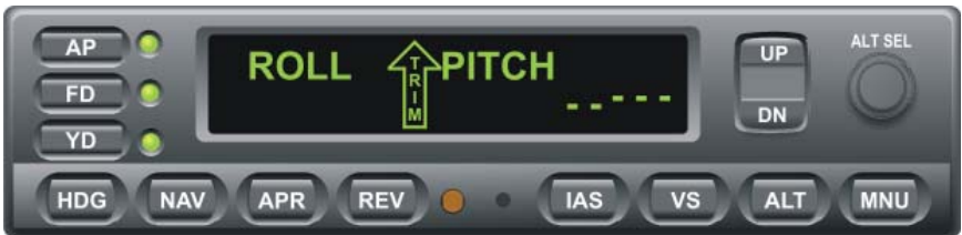
Fig. 3-15. AP Display, AUTO TRIM UP in Progress
