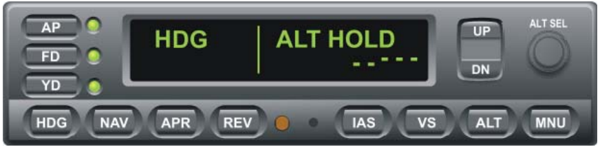
Fig. 2-10. AP Display, HDG and ALT HOLD Modes Engaged (Pre-Flight)
