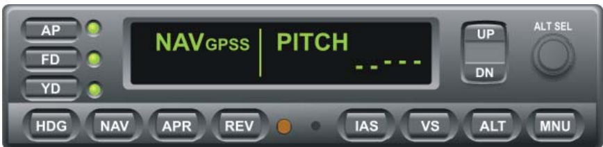
Fig. 3-5. AP Display, GPSS and PITCH Modes Engaged
