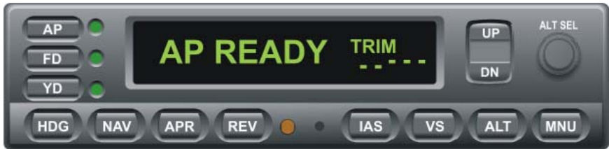
Fig. 3-17. AP Display, MANUAL ELECTRIC TRIM in Progress
