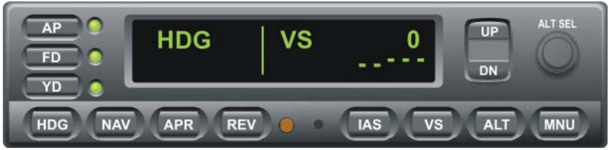
Fig. 2-9. AP Display, HDG and VS Modes Engaged (Pre-Flight)
