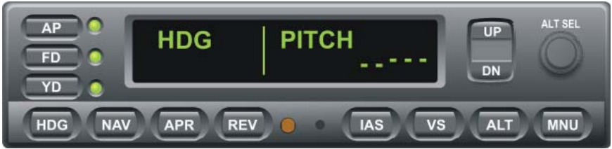
Fig. 2-7. AP Display, HDG and PITCH Modes Engaged (Pre-Flight)
