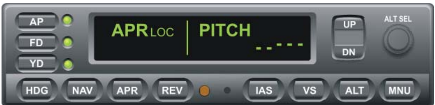
Fig. 3-36. AP Display, APR LOC Mode Engaged, Track LOC Front Course Inbound
