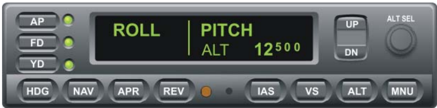
Fig. 3-11. AP Display, ROLL and PITCH Modes Engaged, ALT HOLD Mode Armed
