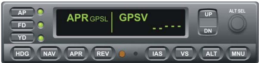
Fig. 3-47. AP Display, APR GPSL and GPSV Modes Engaged
