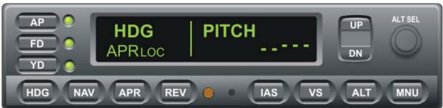
Fig. 3-35. AP Display, HDG Mode Engaged, APR LOC Mode Armed
