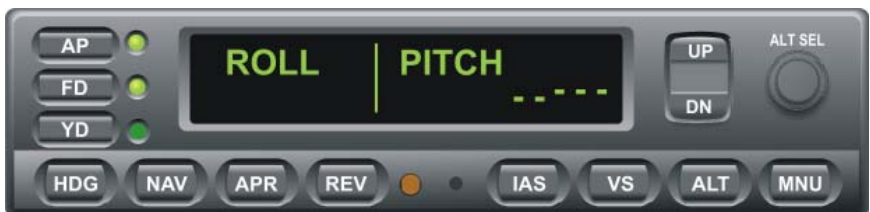
Fig. 3-49. AP Display, YD Mode Disengaged
