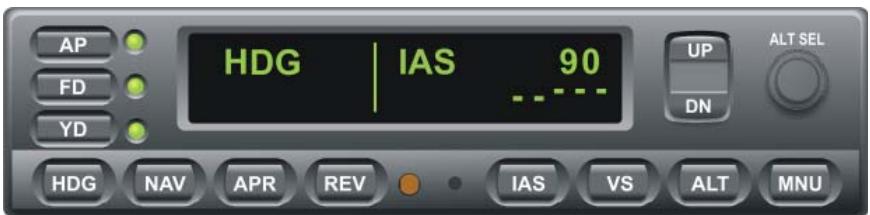
Fig. 2-8. AP Display, HDG and IAS Modes Engaged (Pre-Flight)
