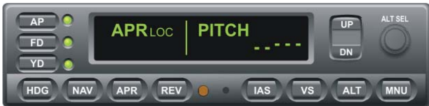
Fig. 3-29. AP Display, APR LOC Mode Engaged, Track LOC Front Course Inbound
