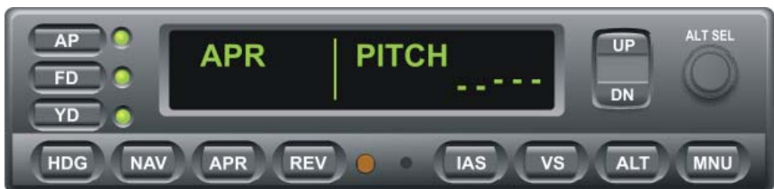
Fig. 3-31. AP Display, APR Mode Engaged, Track VOR Front Course Inbound
