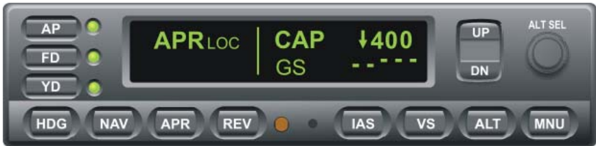
Fig. 3-19. AP Display, APR LOC and GS CAP Modes Engaged
