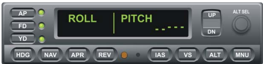
Fig. 3-48. AP Display, YD Mode Engaged
