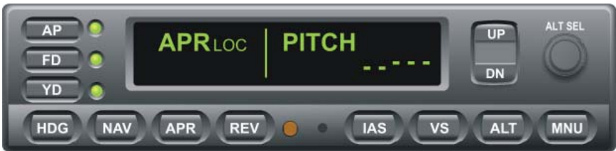
Fig. 3-24. AP Display, APR LOC Mode Engaged, Track LOC Back Course Outbound
