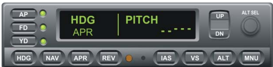
Fig. 3-40. AP Display, HDG Mode Engaged, APR Mode Armed
