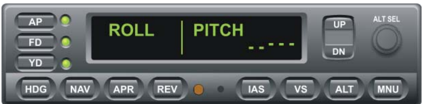
Fig. 3-7. AP Display, ROLL and PITCH Modes Engaged
