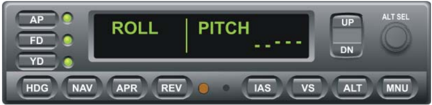
Fig. 2-6. AP Display, ROLL and PITCH Modes Engaged (Pre-Flight)
