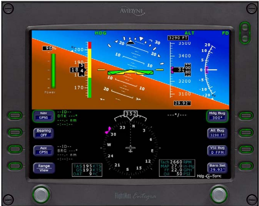
Fig. 3-47. PFD Display, FD Only Mode Engaged
