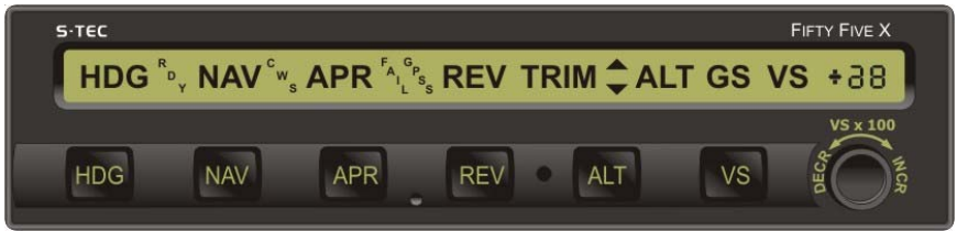
Fig. 2-1. AP Display, Power-Up Annunciations
