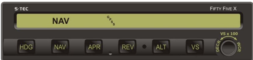
Fig. 3-10. AP Display, GPSS Mode Engaged
