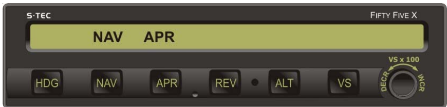
Fig. 3-38. AP Display, APR Mode Engaged, Track VOR Front Course Inbound
