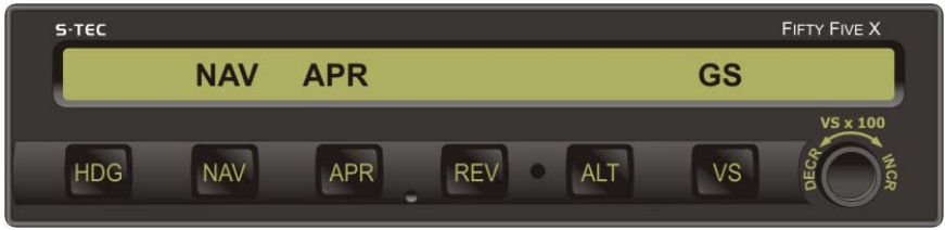
Fig. 3-27. AP Display, NAV, APR, and GS Modes Engaged
