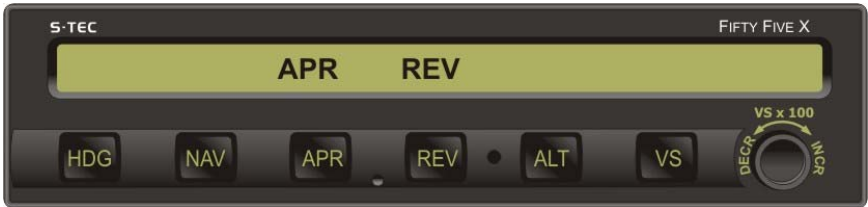
Fig. 3-40. AP Display, APR Mode Engaged, Track LOC Front Course Outbound
