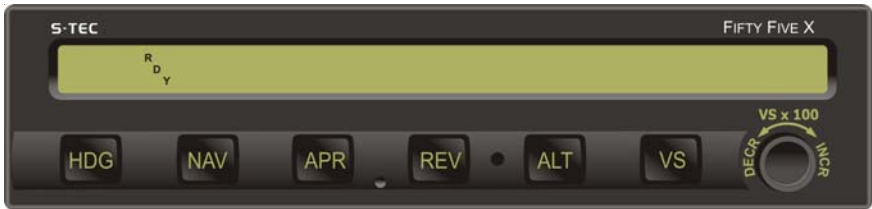
Fig. 2-4. AP Display, RDY Annunciation
