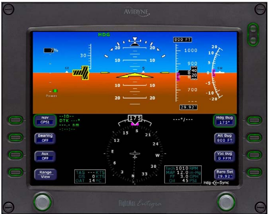
Fig. 2-9. PFD Display, HDG Mode Engaged (Pre-Flight)
