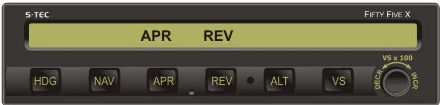
Fig. 3-30. AP Display, APR Mode Engaged, Back Course
