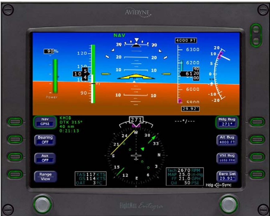
Fig. 3-4. PFD Display, NAV Mode Engaged, A/C on 45° Intercept Angle
