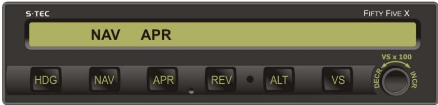
Fig. 3-7. AP Display, APR Mode Engaged
