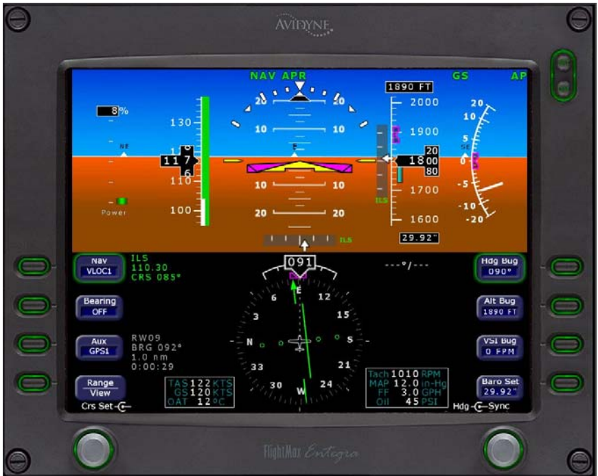
Fig. 3-28. PFD Display, NAV, APR, and GS Modes Engaged
