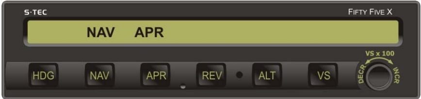
Fig. 3-36. AP Display, APR Mode Engaged, Track LOC Front Course Inbound
