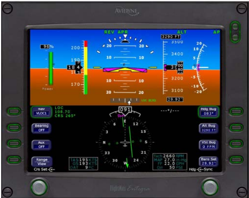
Fig. 3-31. AP Display, APR Mode Engaged, Back Course
