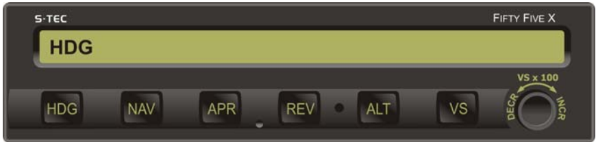
Fig. 2-8. AP Display, HDG Mode Engaged (Pre-Flight)
