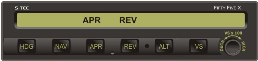
Fig. 3-34. AP Display, APR Mode Engaged, Track LOC Back Course Inbound
