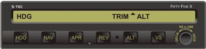
Fig. 3-22. AP Display, HDG and ALT HOLD Modes Engaged, Autotrim in Progress
