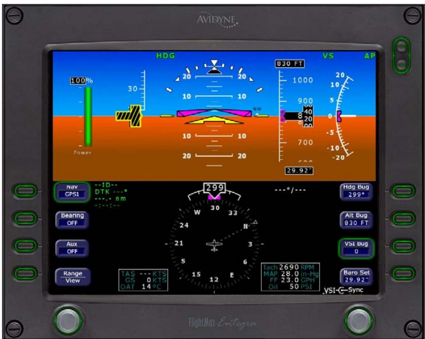
Fig. 2-13. PFD Display, HDG and VS Modes Engaged (Pre-Flight)
