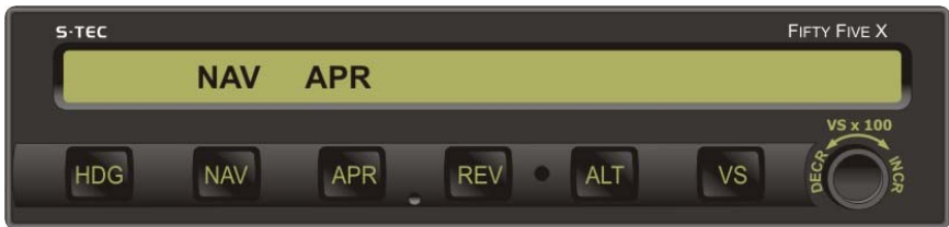
Fig. 3-44. AP Display, APR Mode Engaged, Track VOR Front Course Inbound
