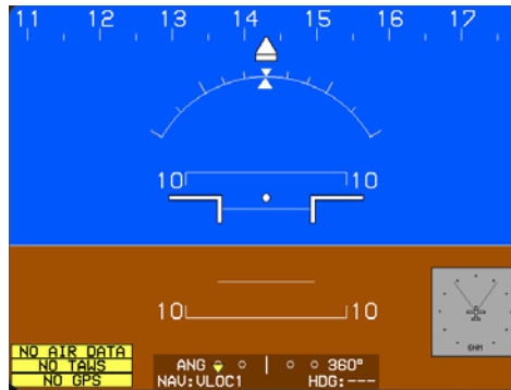
PFD page during ADC and GPS failure
