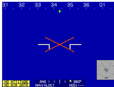
PFD page during ADC and AHRS failure
