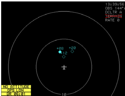
ND during GPS, ADC, and AHRS failure
