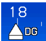
Figure 3-36: DG Indicated when AHRS in DG Mode
