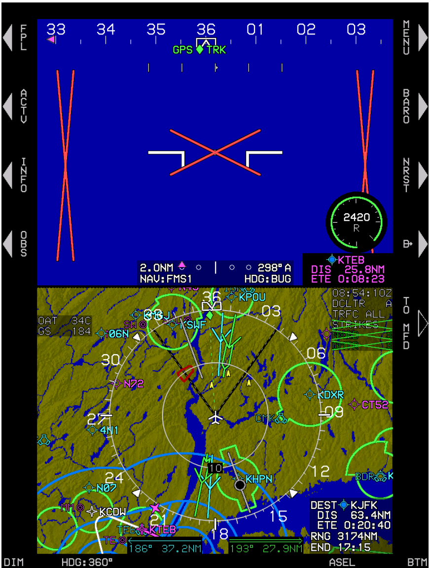
Figure 4-22: MFD Failure Mode 6 (Essential Mode) ADC and AHRS Failed, GPS/SBAS Normal
