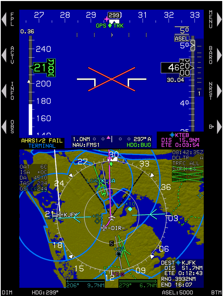
Figure 4-12: PFD Failure Mode 3 (Normal Mode) AHRS Failed, GPS/SBAS and ADC Normal
