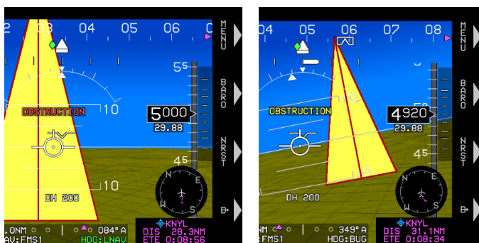
Figure 2-12: Time-Critical Warning and Caution Alerts
