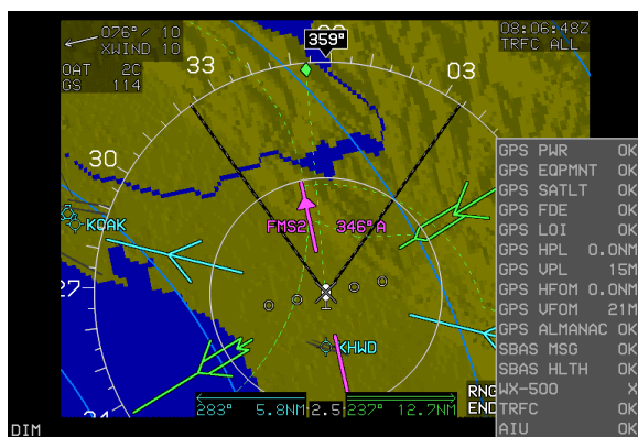
Figure 4-1: FAULTS Page on MFD
