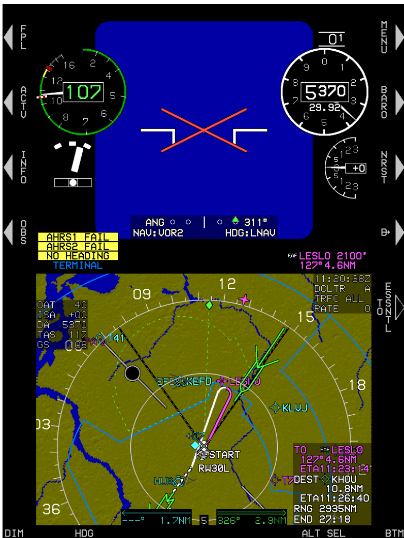
Figure 4-14: PFD Failure Mode 3 (Normal Mode) AHRS Failed, GPS/SBAS and ADC Normal (Round Dials)
