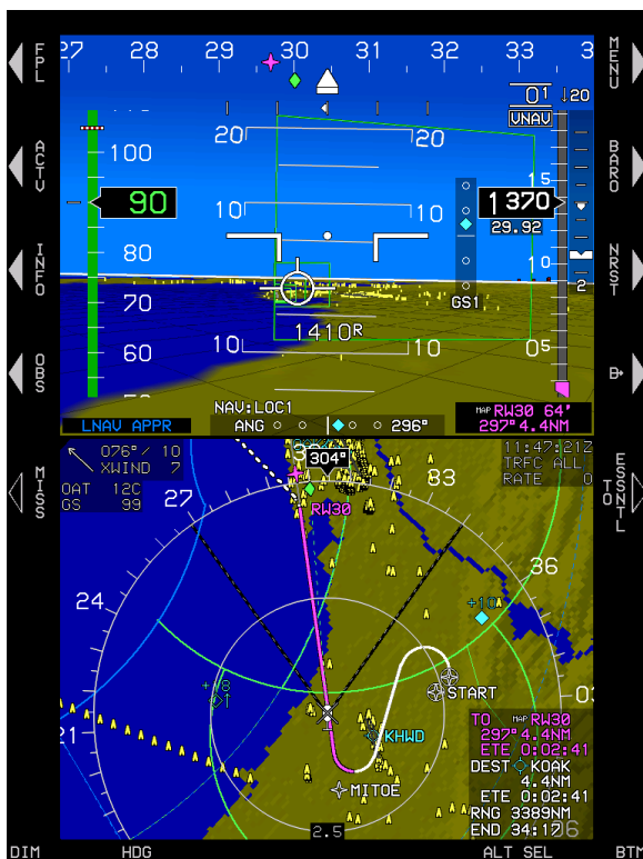
Figure 7-5: Highway in the Sky Final Approach Segments
