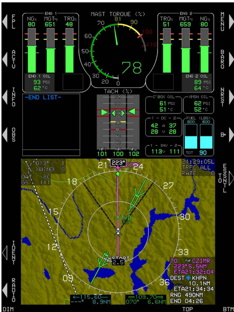
Figure 3-5: MFD in Normal Mode with EICAS Page on Top and MAP on Bottom
