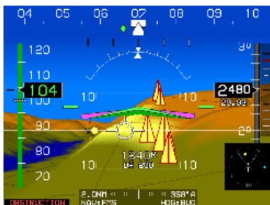
Obstructions creating an OBSTRUCTION warning
