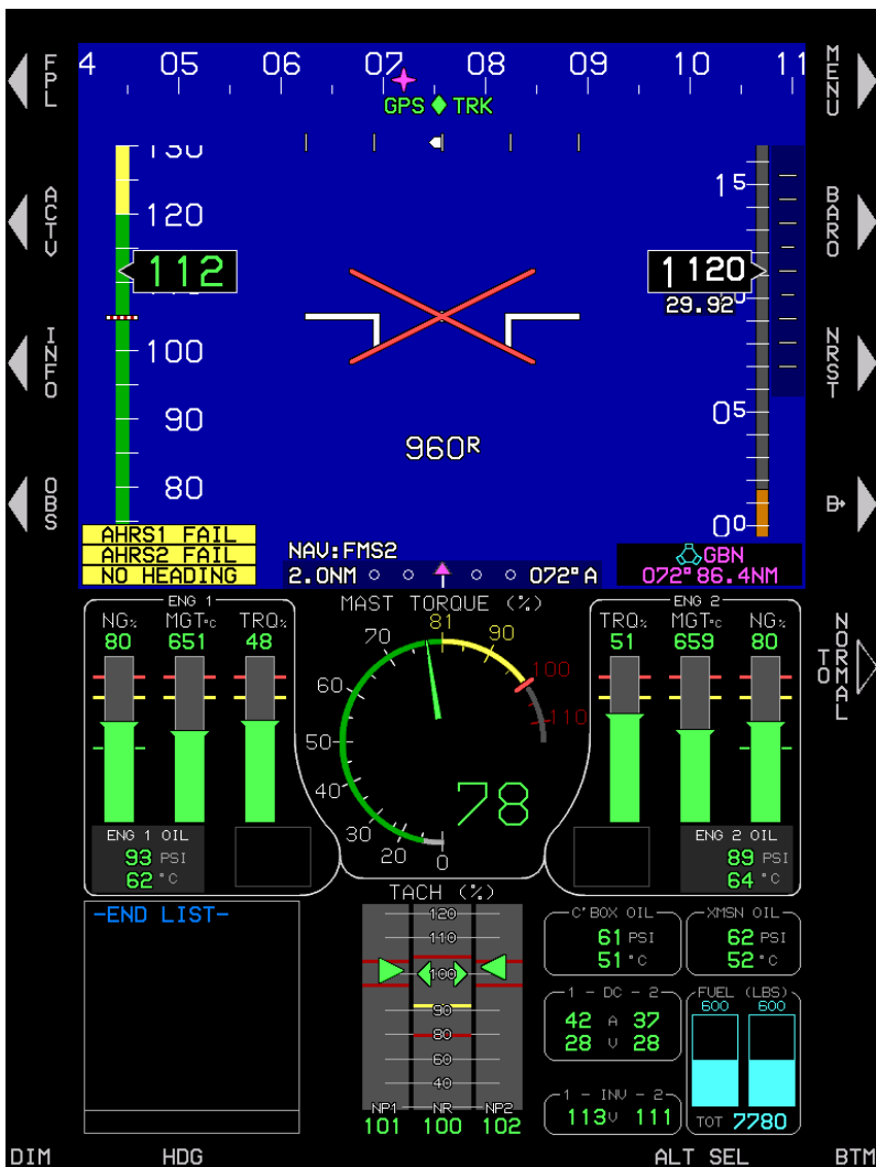
Figure 4-13: PFD Failure Mode 3 (Normal Mode) AHRS Failed, GPS/SBAS and ADC Normal (Tapes)
