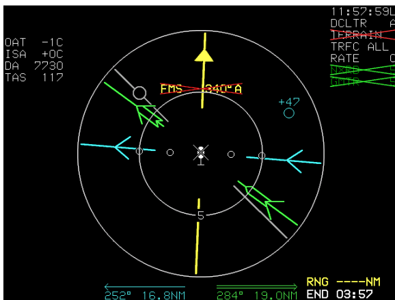
Figure 4-19: MFD Failure Mode 5 GPS/SBAS and AHRs Failed; ADC Normal
