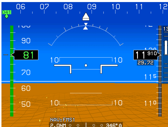
Figure 3-54: PFD with Flight Path Marker Removed (Tapes only)
