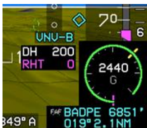
Figure 3-29: AW-109SP Decision Height and Radar Height Readout
