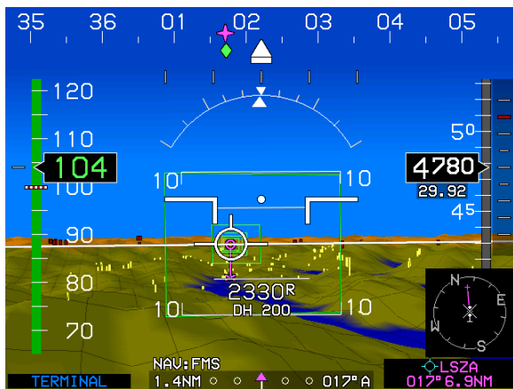
Figure 4-2: PFD (Tapes) Failure Mode 0 GPS, ADC, and AHRS Normal
