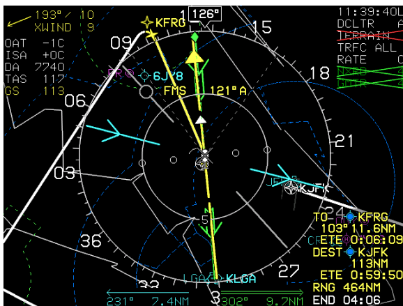
Figure 4-7: MFD Failure Mode 1 GPS/SBAS Failed; ADC and AHRS Normal
