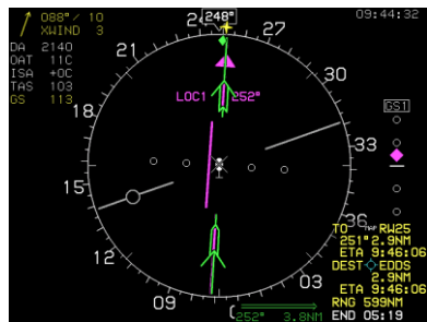
GPS Loss of Navigation Condition Amber (Yellow) Pointer Color
