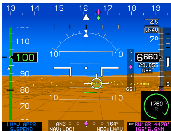
Figure 3-71: EFIS Coupled Vertically with Glideslope Mode Engaged
