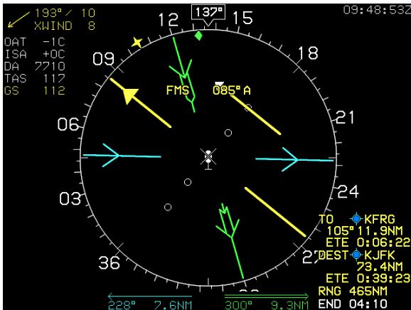
Figure 3-101: Conventional HSI/PTR Format with Loss of Navigation Condition
