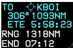
Figure 3-88: Identifier, Bearing, Distance and Time to Active Waypoint (AW-109SP)
