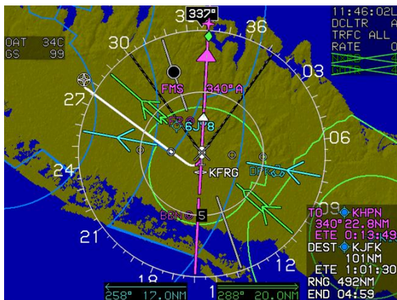
Figure 4-10: MFD Failure Mode 2 ADC Failed; GPS/SBAS and AHRS Normal
