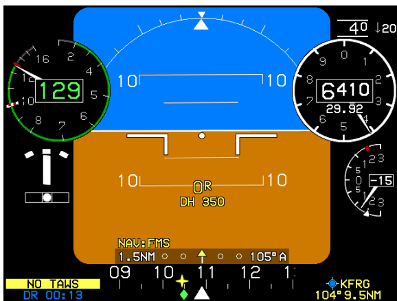
Figure 4-6: PFD (Round Dials) Failure Mode 1 GPS/SBAS Failed; ADC and AHRS Normal
