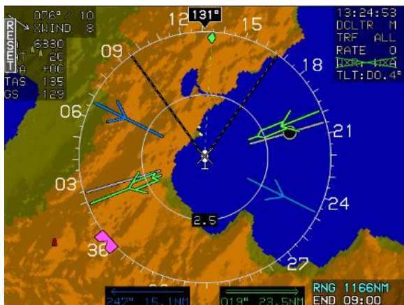
Figure 8-6: Popup Mode Excessive Rate of Descent (GPWS Mode 1)
