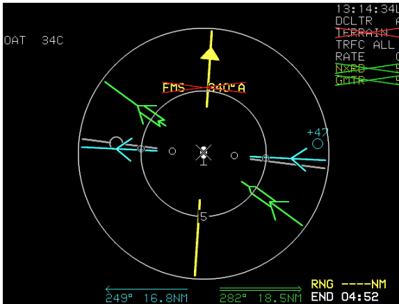
Figure 4-25: MFD Failure Mode 7 GPS/SBAS, ADC, and AHRs Failed
