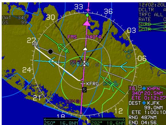
Figure 4-22: MFD Failure Mode 6 ADC and AHRS Failed; GPS/SBAS Normal
