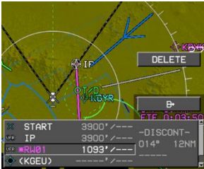
Figure 7-11: Navigating to FAF on VTF VFR Approach
