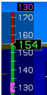
Figure 3-36: Airspeed Display (AW-109SP)
