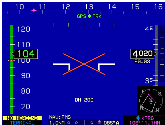
Figure 4-11: PFD (Tapes) Failure Mode 3 AHRS Failed; GPS/SBAS and ADC Normal
