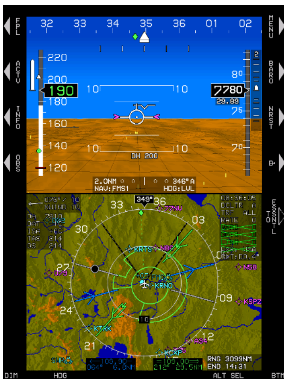
Figure 2-2: Primary IDU-680 PFI on Top Half and ND on Bottom Half
