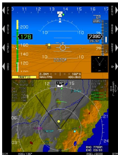
Figure 2-2: Primary IDU-680 PFI on top half and ND on bottom half.
