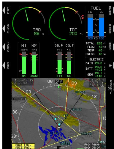
Figure 4-7: MFD Failure Mode 2, (Normal Mode) ADC failed, GPS/SBAS and AHRS normal
