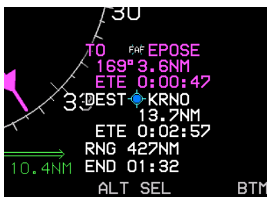
Figure 3-95: HSI Fuel Totalizer / Waypoint Bearing
