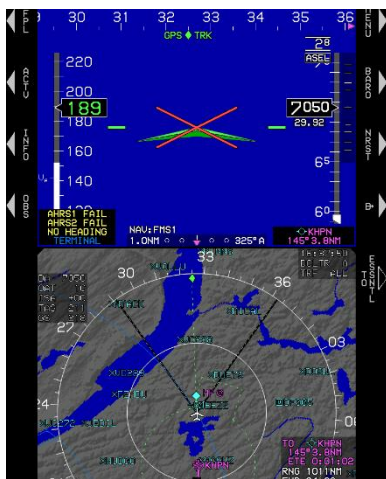
Figure 4-9: PFD Failure Mode 3 (Normal Mode) AHRS failed, GPS/SBAS and ADC normal
