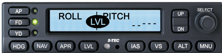
Figure 3-24: Emergency Level Mode; Servos Engaged, No AP
