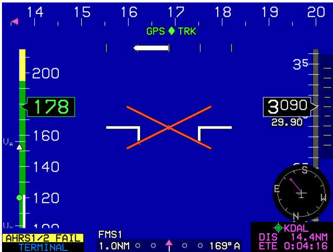
Figure 4-12: PFD Failure Mode 3 AHRs Failed, GPS/SBAS and ADC Normal
