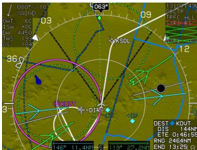
Figure SAR-9: Orbit Pattern
