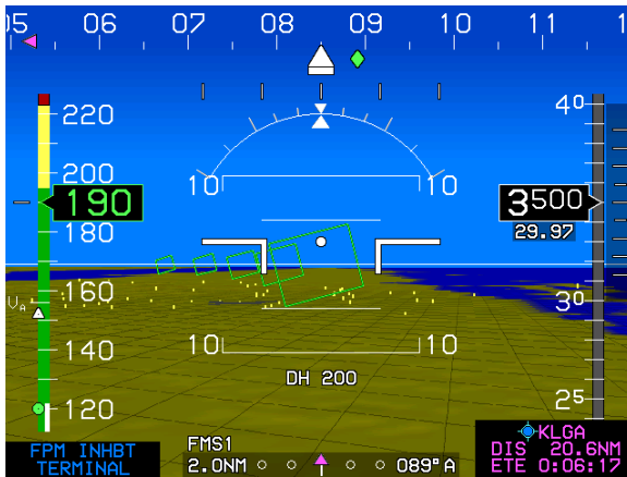
Figure 3-43: Flight Path Marker Absence
