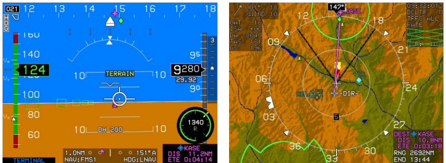
Figure 3-38: Terrain Deselected on PFD and Retained on MFD Map
