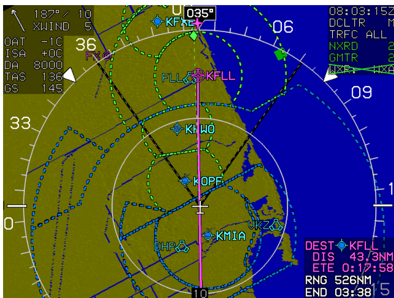
Figure 3-61: Basic Moving Map
