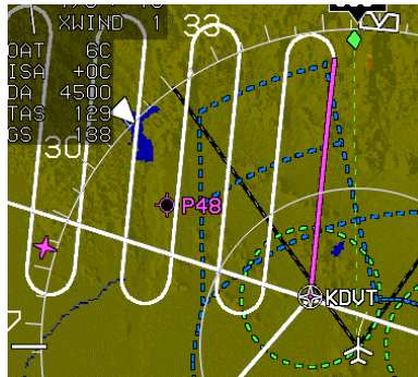
Figure SAR-5: Rising Ladder Pattern
