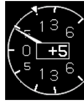
VSI bug set to +1,000 fpm without Genesys/S-TEC DFCS enabled
