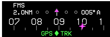
Figure RD-28: Heading Indicator with Heading Failure and Good GPS
