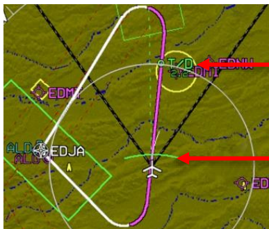
Figure 3-68: Top-of-Descent and Bottom-of-Descent
