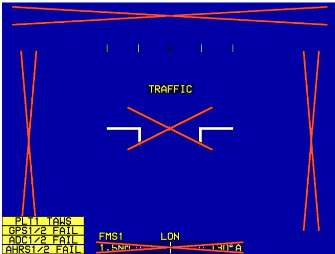
Figure 4-20: PFD Failure Mode 7 GPS/SBAS, ADC and AHR Failed
