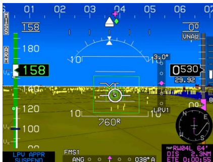
Obstructions without hazardous condition
