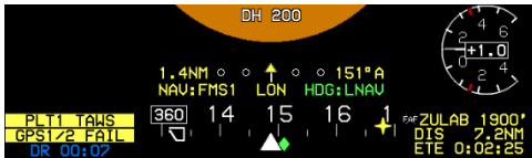
Figure RD-36: Course Deviation Indicator
