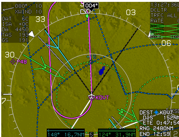
Figure SAR-12: Race Track Pattern
