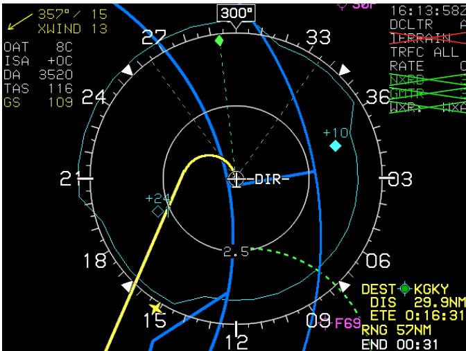
Figure 4-9: MFD Failure Mode 1 GPS/SBAS Failed, ADC and AHRS Normal
