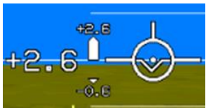
Figure 3-32: G-Force Indicator Telltale Indications
