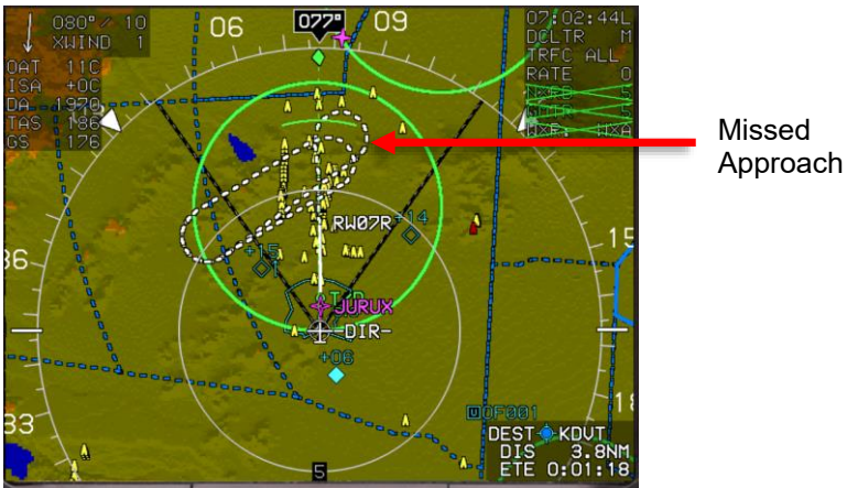
Figure 7-17: Missed Approach and Departure Path
