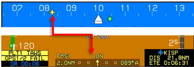
Figure 3-25: GPS Loss of Navigation (LON)
