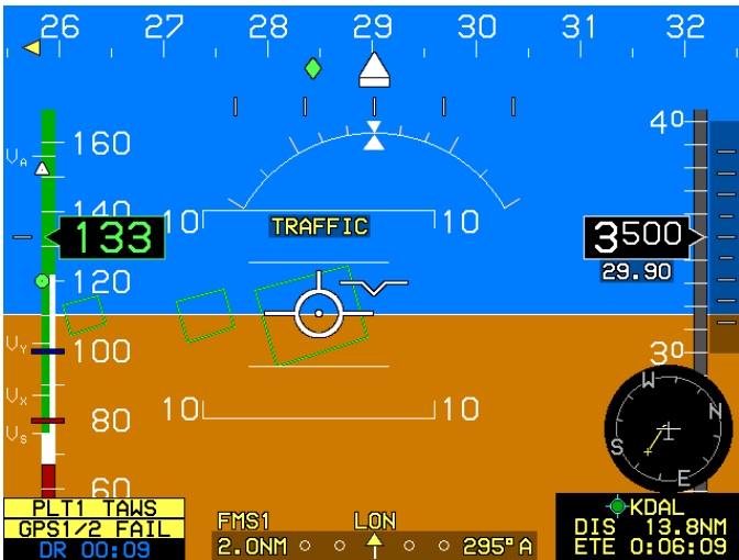
Figure 4-8: PFD Failure Mode 1 GPS/SBAS Failed, ADC and AHRS Normal
