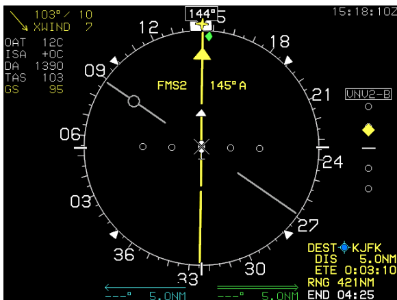
Figure 3-90: Conventional HSI with Loss of Navigation Condition
