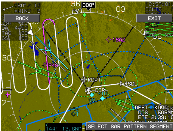
Figure SAR-8: Rising Ladder Pattern-Individual Leg Selected
