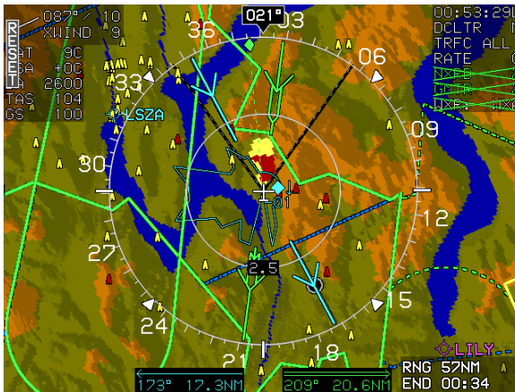
Figure 8-2: MFD Terrain Display
