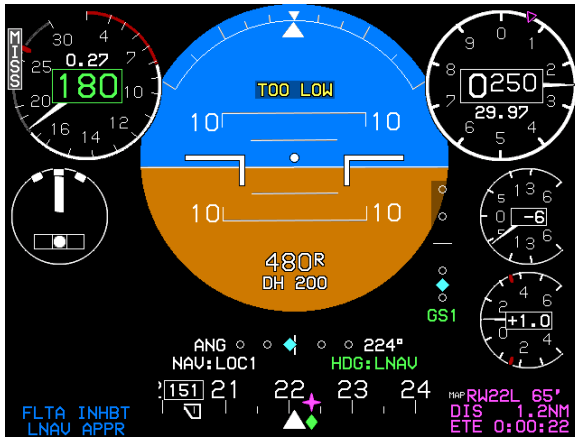
Figure RD-37: EFIS Coupled Vertically with Glide Slope Mode
