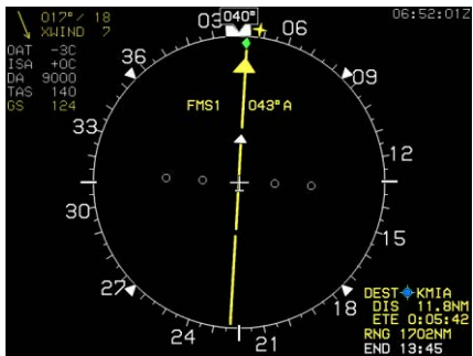
GPS LON Condition Amber (Yellow) Pointer
