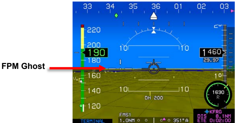
Figure 3-42: Flight Path Marker Ghost
