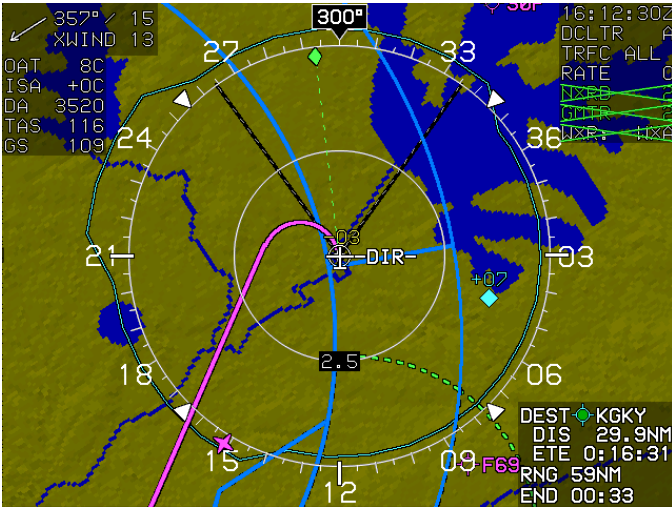
Figure 4-7: MFD Failure Mode 0 GPS, ADC and AHRS Normal
