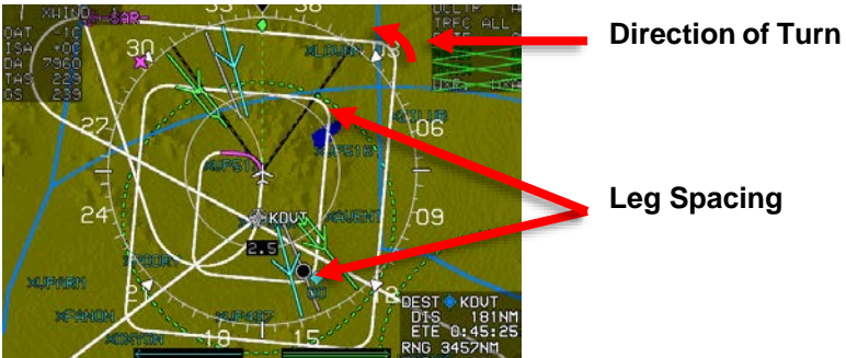
Figure SAR-3: Expanding Square Pattern-Turn and Leg
