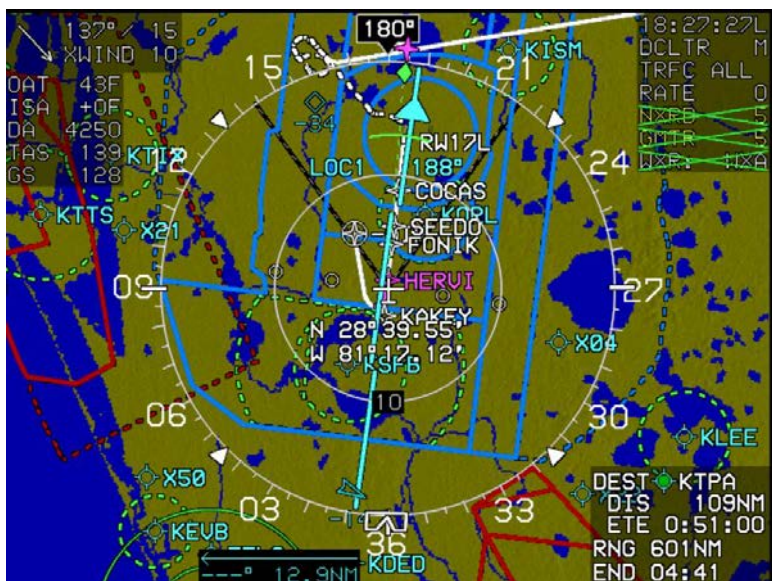
Figure 3-62: Moving Map with Instrument Approach with HSI Overlay Selected
