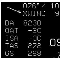
Figure 3-96: HSI Display Air Data and Ground Speed
