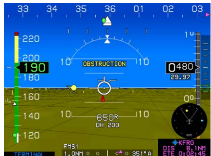
Obstructions creating an OBSTRUCTION caution
