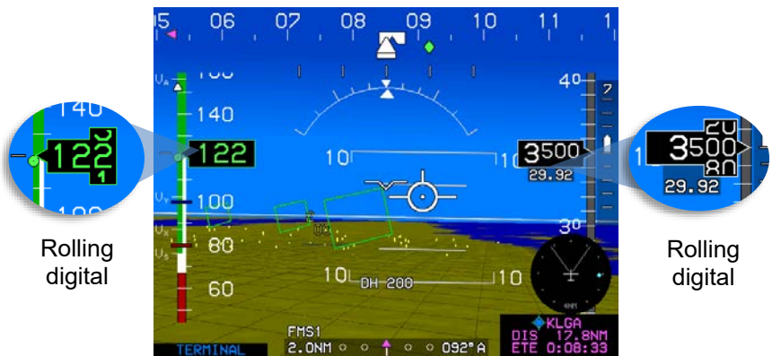
Figure 3-1: PFD Normal SVS Mode, Pure Digital and Rolling Configuration
