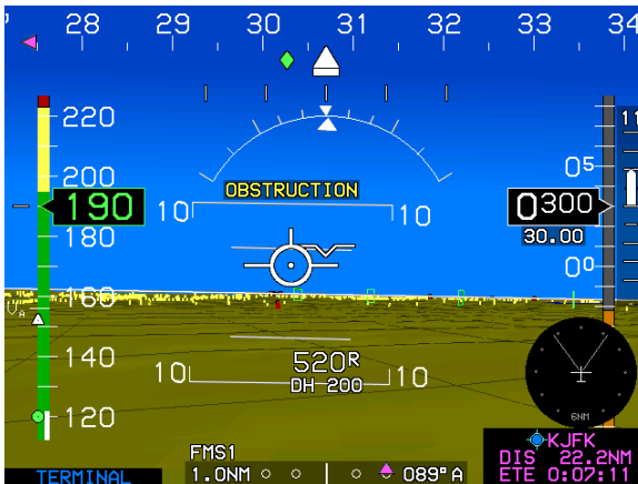
Figure 2-10: Time-Critical Caution Alert
