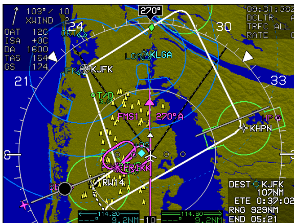
Figure 3-76: Navigation Data and Airspace Depiction
