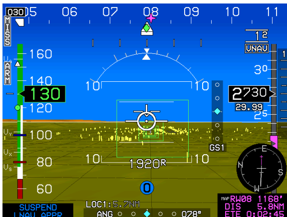
Figure 7-7: Highway in the Sky Final Approach Segments
