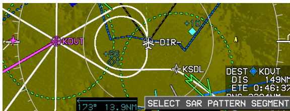
Figure SAR-19: Sector Search Pattern-Individual Leg Selected
