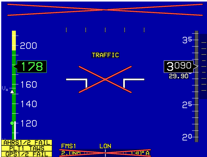
Figure 4-16: PFD Failure Mode 5 GPS/SBAS and AHRs Failed, ADC Normal
