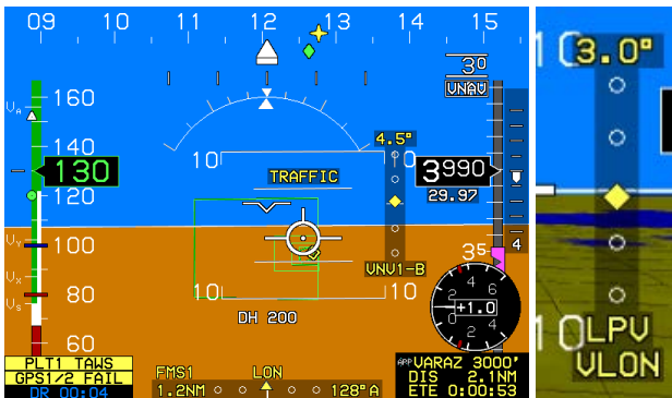
Figure 3-55: VDI Color during GPS/SBAS LON or VLON
