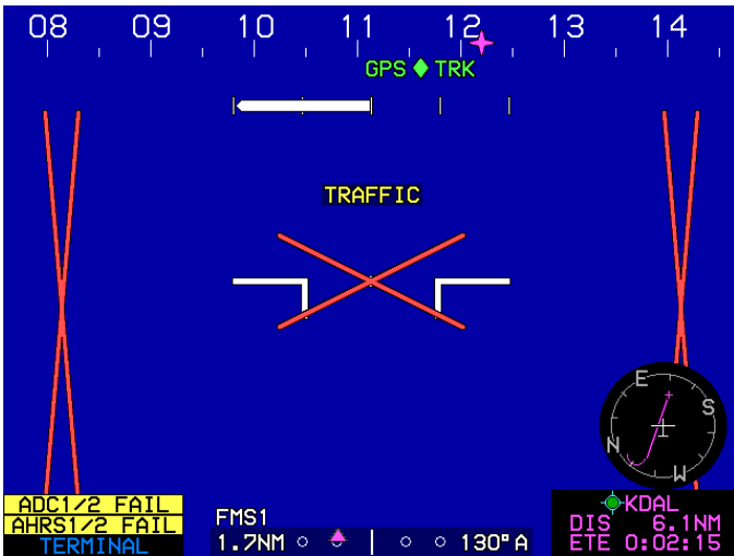
Figure 4-18: PFD Failure Mode 6 ADC and AHRS Failed, GPS/SBAS Normal
