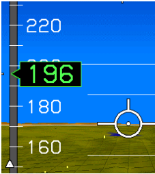
FPM nearing airspeed tape due to strong crosswind.
