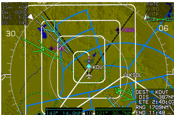
Figure SAR-1: Expanding Square Pattern
