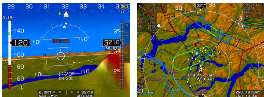
Figure 3-82: Terrain and Obstructions
