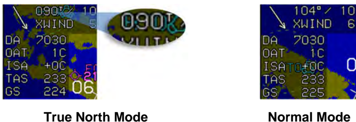
Figure 3-75: Air Data and Groundspeed
