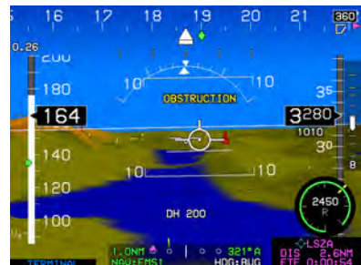
Obstructions creating an OBSTRUCTION caution
