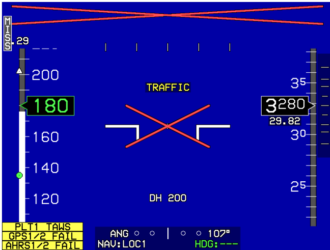
Figure 4-15: PFD Failure Mode 5 GPS/SBAS and AHRs Failed, ADC Normal
