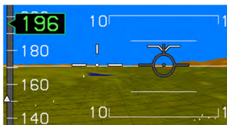
FPM caged in center due to excessive crosswinds from the right. Ghost FPM appears in proper lateral location.
