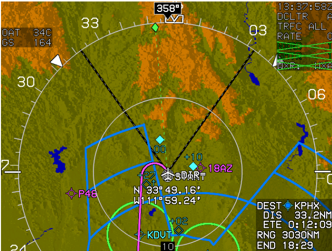
Figure 4-10: MFD Failure Mode 2, (Normal Mode) ADC Failed, GPS/SBAS and AHRS Normal
