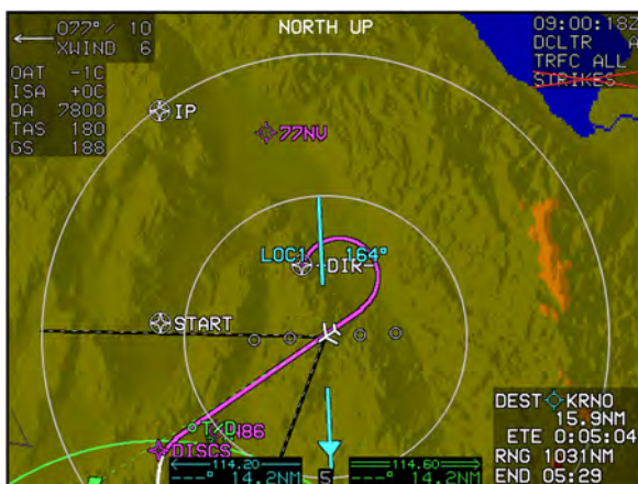
Figure 3-70: North-Up Arc Mode with HSI Enabled and VOR1 Selected
