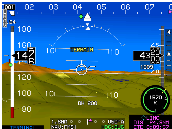
Figure 2-10: Time-Critical Caution Alert
