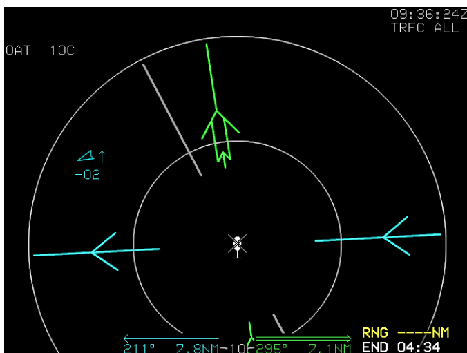
Figure 4-17: MFD Failure Mode 5 GPS/SBAS and AHRs Failed; ADC Normal
