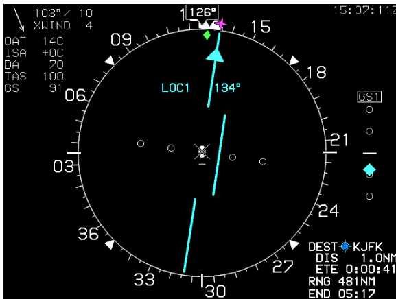
Figure 3-92: Conventional HSI/PTR Format: HSI with VDI and Glide Slope
