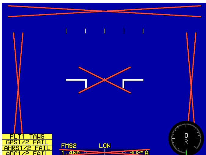
Figure 4-20: PFD Failure Mode 7 GPS/SBAS, ADC, and AHRS Failed
