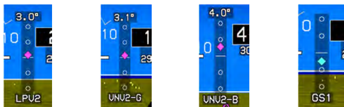
Figure 3-56: Vertical Deviation Indicator
