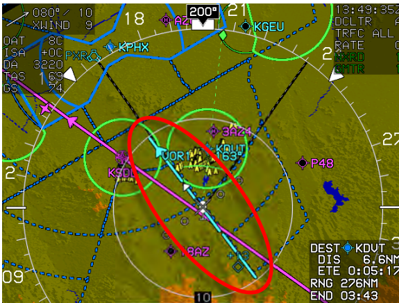
Figure 3-76: Analog Navigation Symbology HSI in ARC Mode
