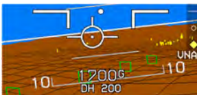
(SVS Basic) AGL Based on GPS Altitude
