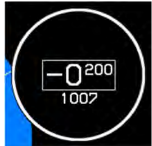
Altitude display when below sea level
