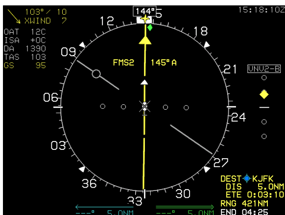
Figure 3-93: Conventional HSI/PTR Format with Loss of Navigation Condition
