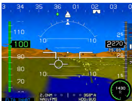
Obstructions without Hazardous Condition
