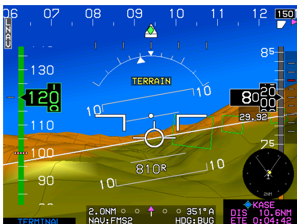
Figure 2-10: Time-Critical Caution Alert
