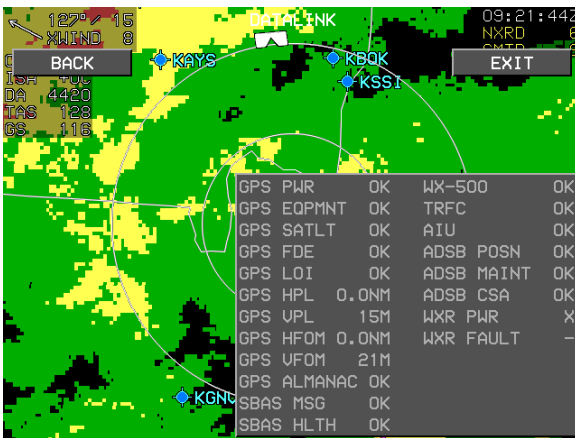
Figure D-16: MFD Fault Display Menu
