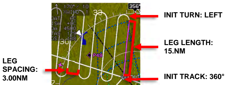
Figure SAR-7: Rising Ladder Pattern-Turn, Leg, and Track Parameters
