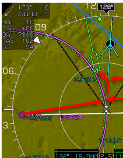
Figure SAR-11: Orbit Pattern-Turn and Radius Parameters
