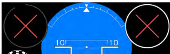
Figure RD-6: Airspeed and Altitude with Loss of ADC
