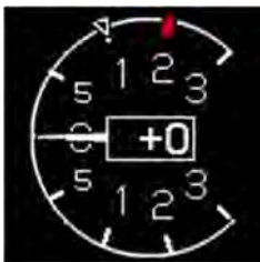
VSI bug set to +1,000 fpm with HelisAS enabled
