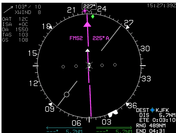
Figure 3-97: HSI Display Air Data and Ground Speed
