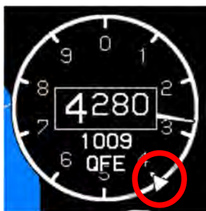
Figure RD-6: Airspeed and Altitude with Loss of ADC
