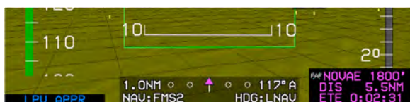
Figure 7-13: FSD Lateral Deviation Indicator Linear Deviation (not VTF Approach)
