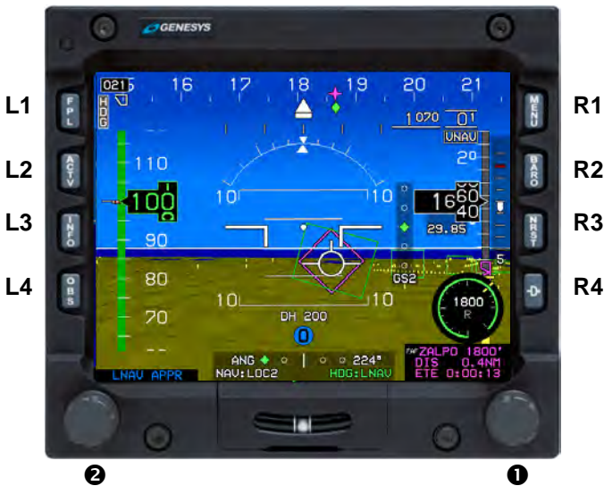
Figure 5-1: IDU-450 Input Controls
