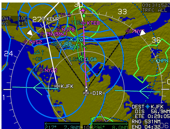
Figure 4-13: MFD Failure Mode 3 AHRs Failed; GPS/SBAS and ADC Normal
