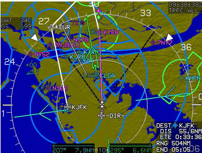
Figure 4-19: MFD Failure Mode 6 ADC and AHRS Failed; GPS/SBAS Normal
