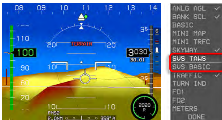
Figure 8-15: Automatic PFD Terrain Warning
