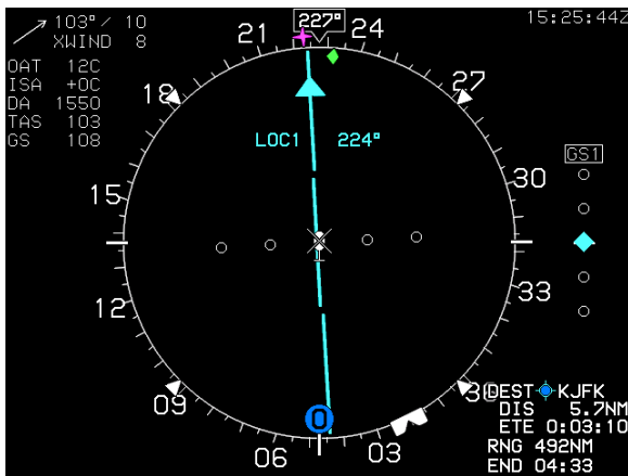
Figure 3-95: HSI with Marker Beacon Displayed
