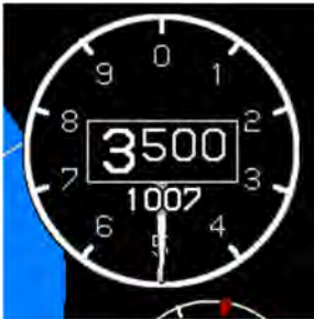
Altimeter display with labels and graduations
