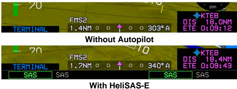
Figure 3-55: CDI No Autopilot or Fully-Integrated Autopilot
