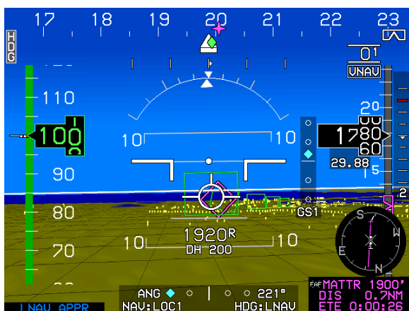
Figure 7-6: Highway in the Sky Final Approach Segments
