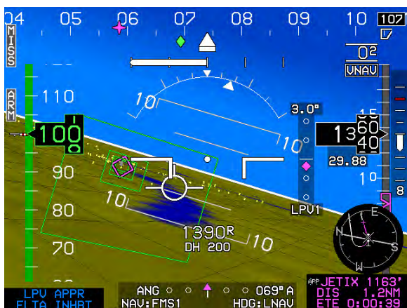
Figure 7-15: GPS Mode (LPV APPR)
