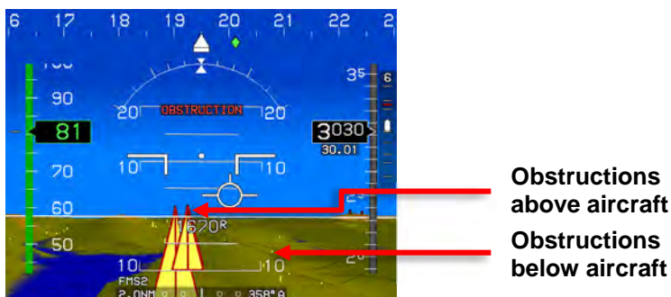
Figure 8-16: PFD SVS TAWS Option and Obstructions
