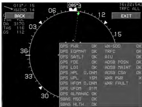
Figure T-20: MFD Faults Menu
