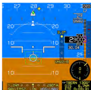
Figure 3-57: VDI Color during GPS/SBAS LON or VLON
