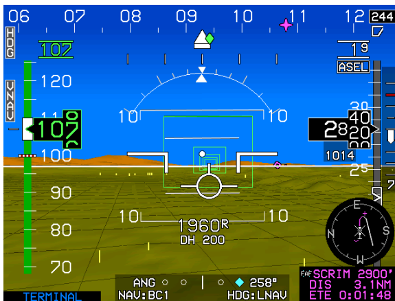
Figure 3-26: Airspeed Display (with EFIS-Coupled)
