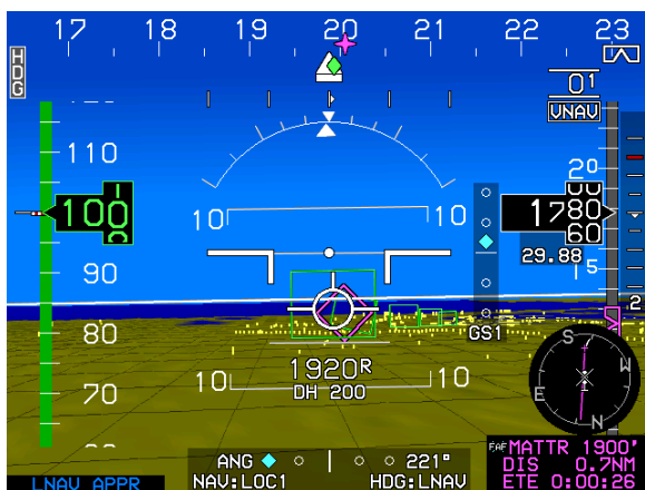
Figure 7-5: Highway in the Sky Final Approach Segments
