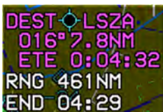
GPS in normal state and current active waypoint
