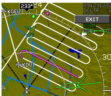
Figure SAR-8: Rising Ladder Pattern-Individual Leg Selected
