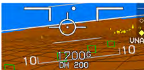
(SVS Basic) AGL Based on GPS Altitude
