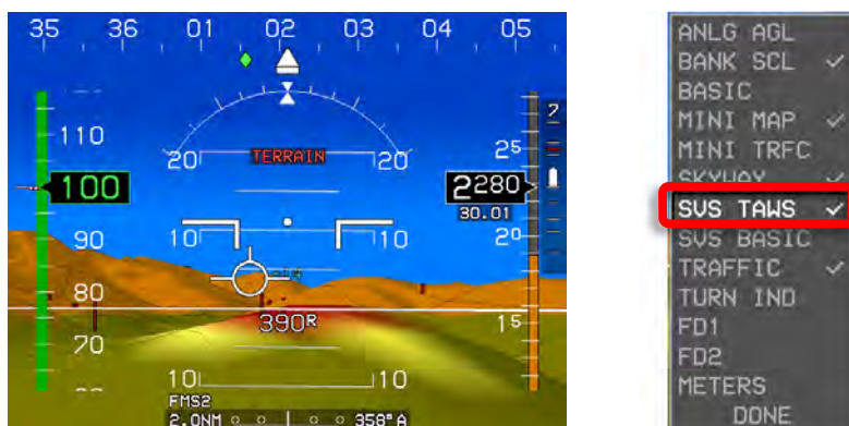
Figure 8-14: PFD SVS TAWS Option
