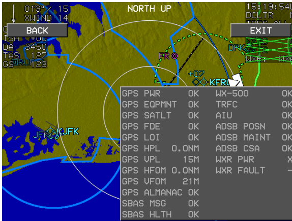
Figure 4-4: FAULTS Page on MFD
