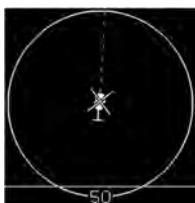
Figure D-5: Datalink Symbology Rotorcraft Ownship Symbol
