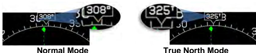
Figure T-8: Traffic Screen Range Compass Rose Symbols
