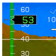
FPM removed due to excessive crosswinds from the right
