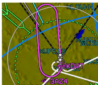
Figure SAR-12: Race Track Pattern
