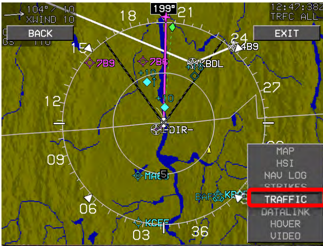
Figure T-1: MFD Traffic Page Access
