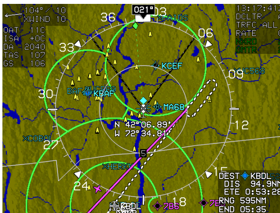
Figure 3-70: Heading-Up Centered Mode
