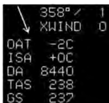
Figure S-3: Air Data and Groundspeed
