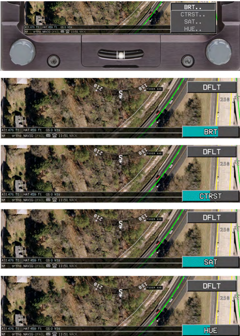
Figure V-2: Video Controls Settings
