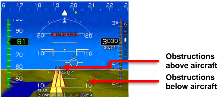
Figure 8-16: PFD SVS TAWS Option and Obstructions
