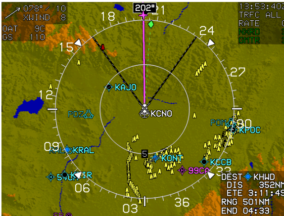
Figure 3-65: Basic Moving Map
