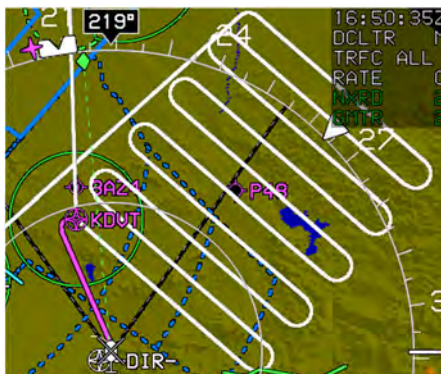
Figure SAR-5: Rising Ladder Pattern
