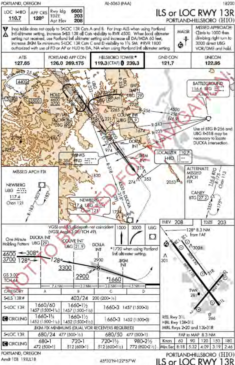
Figure 7-20: ILS Instrument Approach (KHIO)
