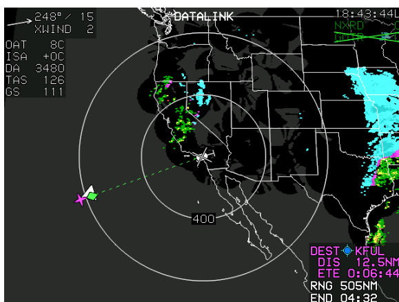
Figure D-8: Datalink Page Screen Range
