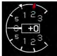
VSI bug set to +1,000 fpm without autopilot enabled.
