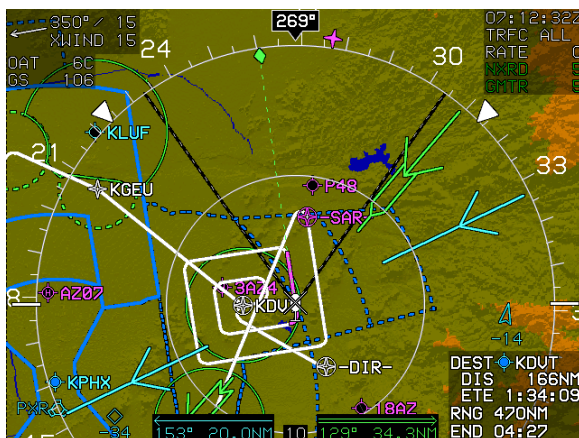
Figure SAR-1: Expanding Square Pattern
