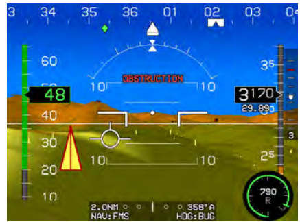
Obstructions Creating an OBSTRUCTION Warning
