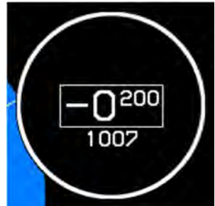
Altitude display when below sea level
