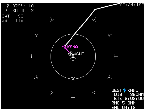
Figure S-5: Active Flight Plan Path/Manual Course/Runways
