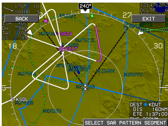
Figure SAR-18: Sector Search Pattern-Individual Leg Selected
