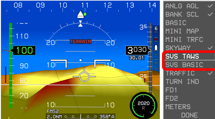
Figure 8-15: Automatic PFD Terrain Warning
