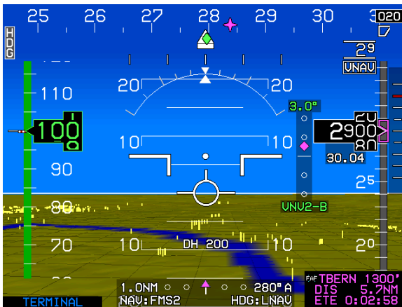
Figure 3-57: EFIS Coupled Vertically with Glideslope Mode Engaged
