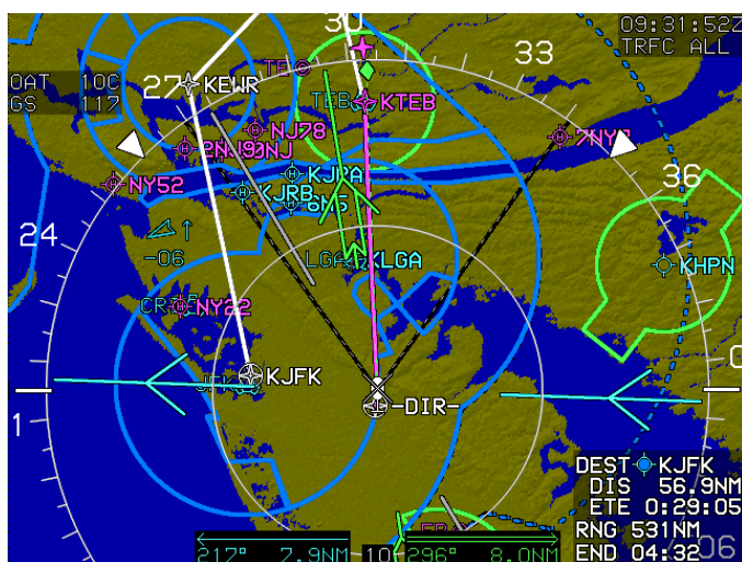
Figure 4-12: MFD Failure Mode 3 AHRs Failed; GPS/SBAS and ADC Normal
