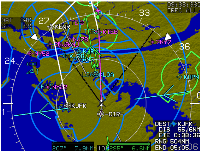
Figure 4-18: MFD Failure Mode 6 ADC and AHRS Failed; GPS/SBAS Normal
