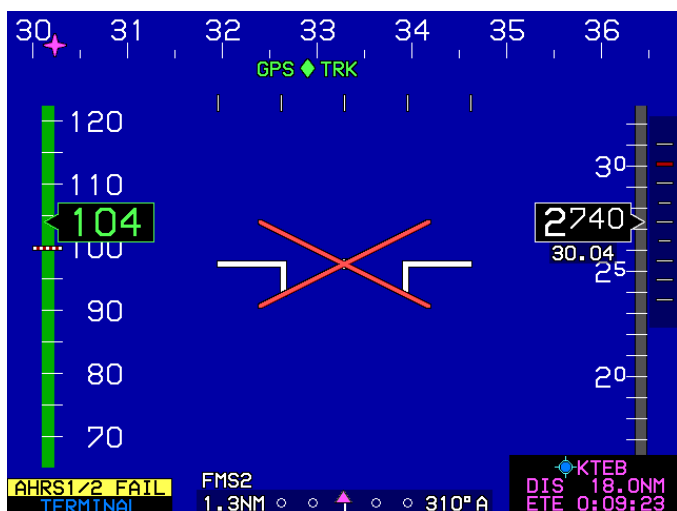
Figure 4-11: PFD Failure Mode 3 AHRs Failed; GPS/SBAS and ADC Normal
