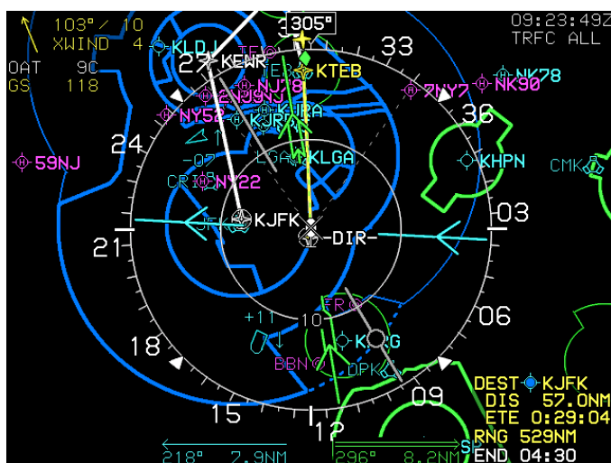
Figure 4-8: MFD Failure Mode 1 GPS/SBAS Failed; ADC and AHRS Normal
