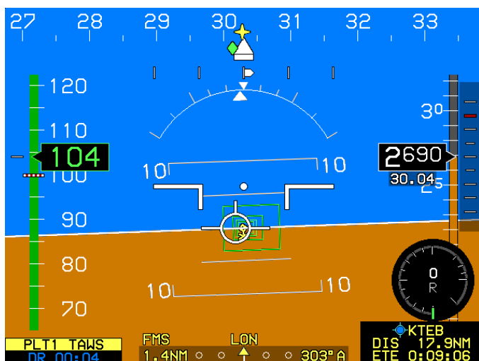
Figure 4-7: PFD Failure Mode 1 GPS/SBAS Failed; ADC and AHRS Normal
