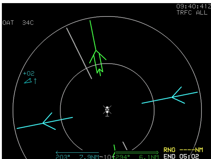
Figure 4-20: MFD Failure Mode 7 GPS/SBAS, ADC, and AHRS Failed
