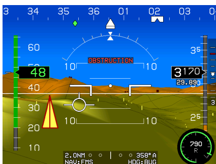
Obstructions Creating an OBSTRUCTION Warning
