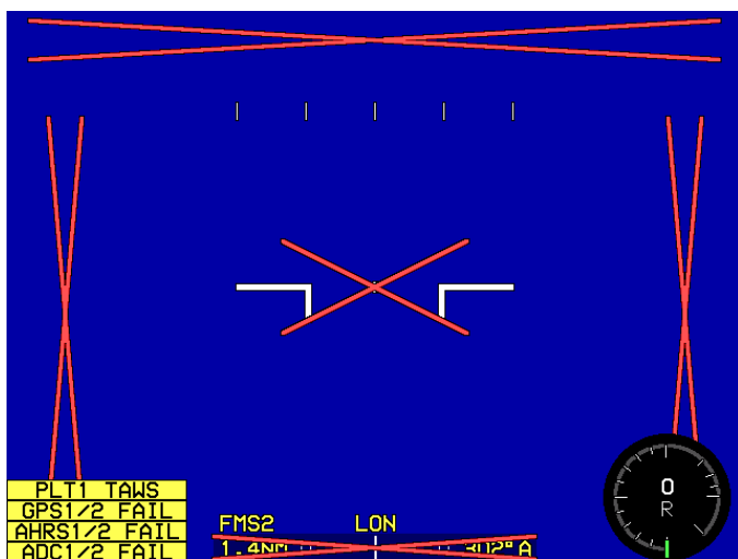
Figure 4-19: PFD Failure Mode 7 GPS/SBAS, ADC, and AHRS Failed
