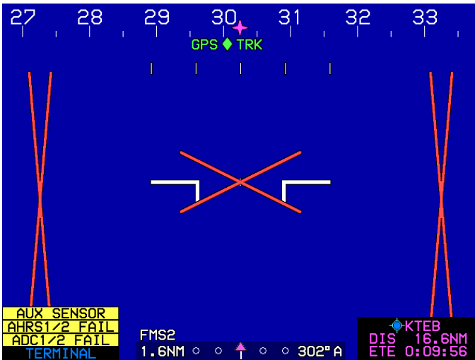
Figure 4-17: PFD Failure Mode 6 ADC and AHRS Failed; GPS/SBAS Normal
