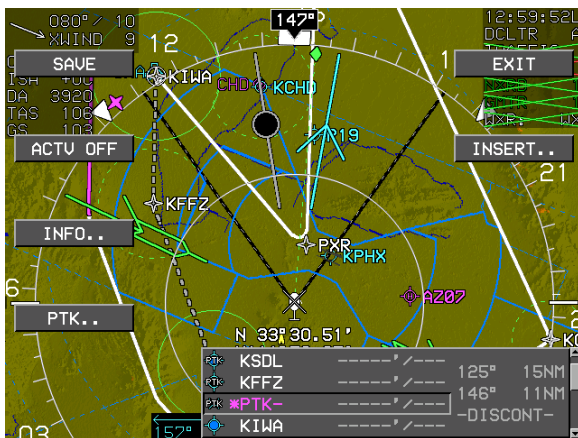
Figure 7-12: Parallel Offset PTK-/PTK ENDING
