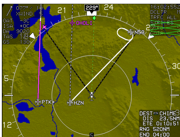
Figure 7-11: Parallel Offset PTK+/PTK ENTRY
