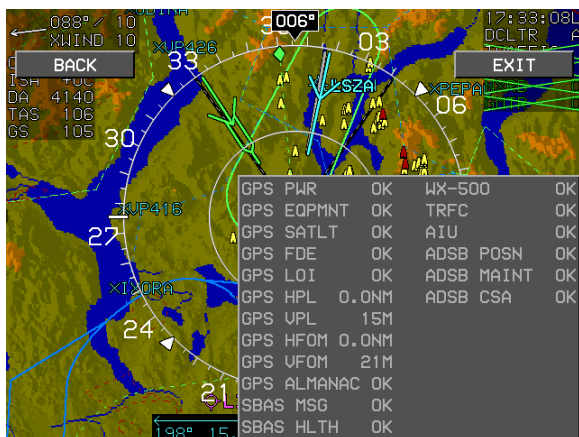
Figure 4-3: FAULTS Page on MFD
