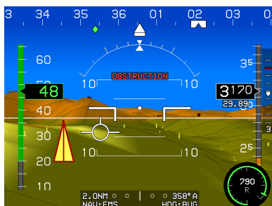
Obstructions Creating an OBSTRUCTION Warning
