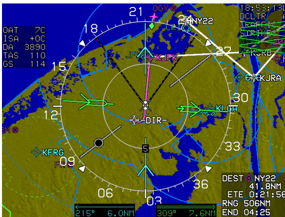
Figure 4-12: MFD Failure Mode 3 AHRs Failed; GPS/SBAS and ADC Normal
