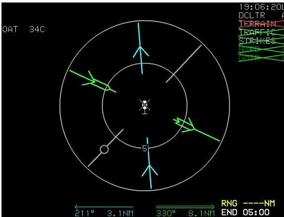
Figure 4-20: MFD Failure Mode 7 GPS/SBAS, ADC, and AHRS Failed
