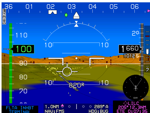
Figure 3-36: PFD Terrain and Obstructions
