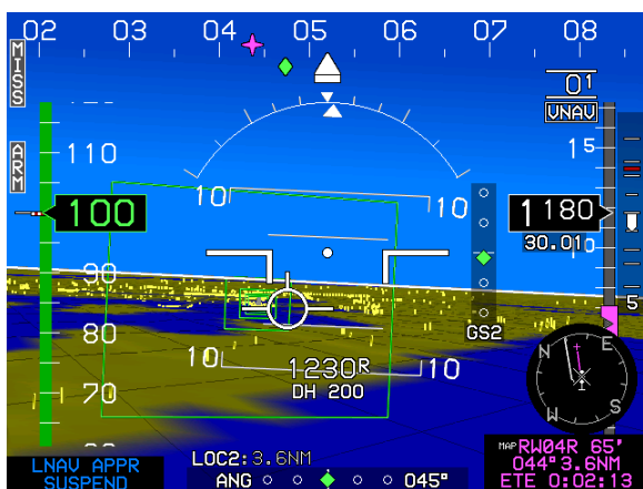
Figure 7-5: Highway in the Sky Final Approach Segments
