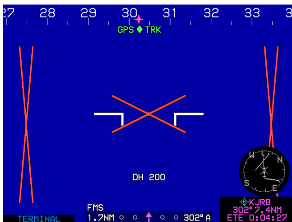
Figure 4-17: PFD Failure Mode 6 ADC and AHRS Failed; GPS/SBAS Normal
