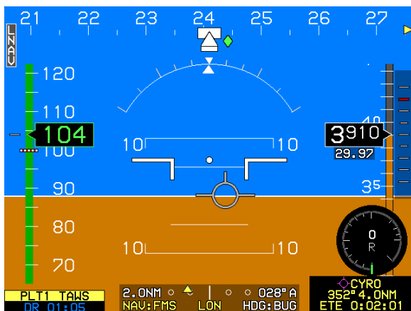
Figure 3-43: PFD with GPS Failure after 1 Minute
