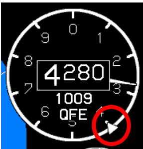
Figure RD-8: Airspeed and Altitude with Loss of ADC
