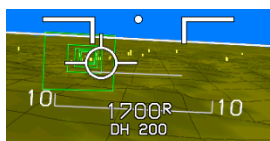
(SVS TAWS) AGL Based on Radar Altimeter
