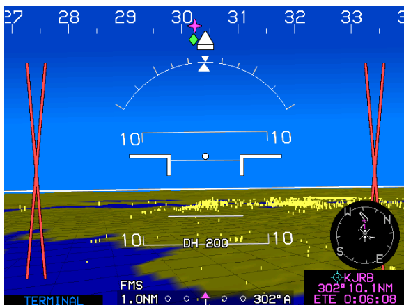
Figure 4-9: PFD Failure Mode 2 (Normal Mode) ADC Failed; GPS/SBAS and AHRS Normal
