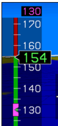
Figure 3-31: Airspeed Display (AW-109SP)
