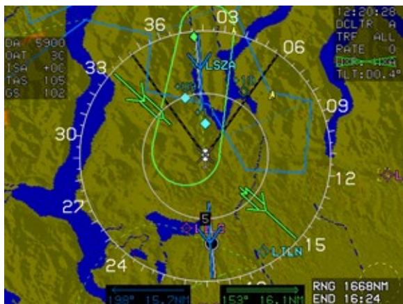
Figure 4-9: MFD Failure Mode 3 AHRS Failed; GPS/SBAS and ADC Normal
