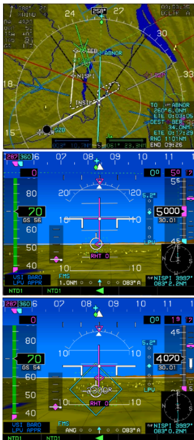
Figure 7-30: Copter RNAV (GNSS) Approach (Step-By-Step) (Continued)
