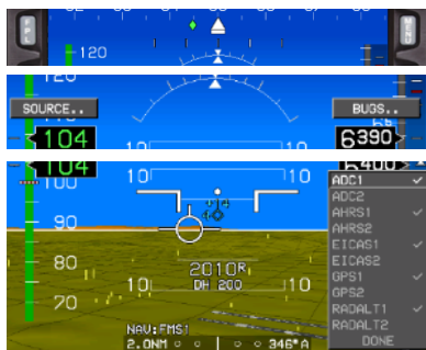
Figure 5-39: PFD Page First-Level Source Selection (Step-By-Step)
