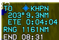
Figure 3-108: Identifier, Bearing, Distance, and Time to Active Waypoint (AW-109SP)
