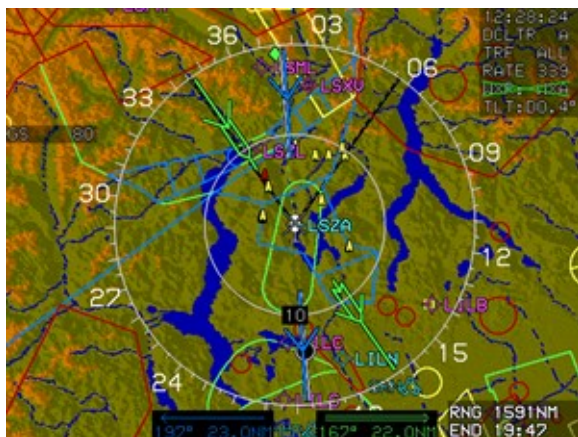
Figure 4-15: MFD Failure Mode 6 ADC and AHRS Failed; GPS/SBAS Normal
