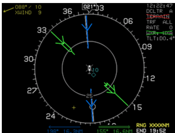
Figure 4-11: MFD Failure Mode 4 GPS/SBAS and ADC Failed; AHRS Normal
