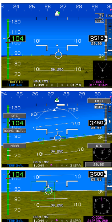
Figure 5-49: Altimeter Menu (Step-By-Step)
