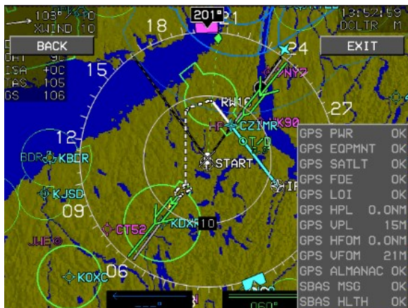
Figure 4-1: FAULTS Page on MFD
