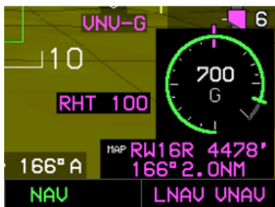
Figure 3-87: Decision Height and Radar Height Readout (AW-109SP)
