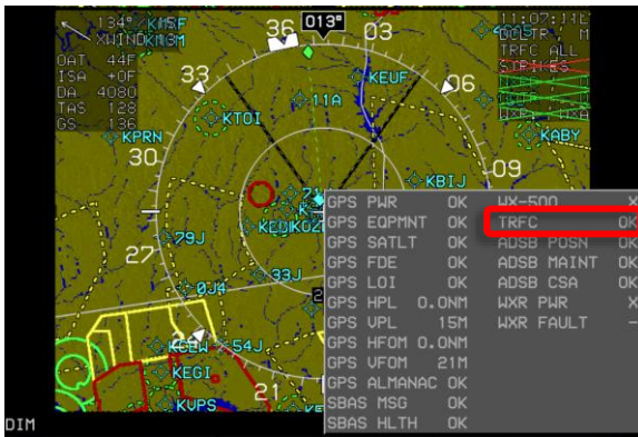
Figure T-17: Menu Faults Status
