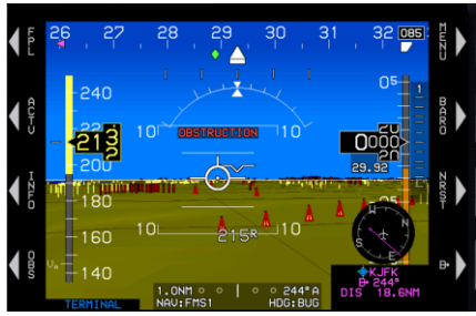
Obstructions creating an OBSTRUCTION warning
