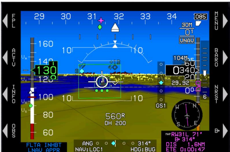
Figure 7-7: Highway in the Sky Final Approach Segments
