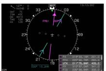
3) If a nav frequency is selected, press TO NAV1 (R2) or TO NAV2 (R3) to send frequency, or push • to change active waypoint to selected localizer.
