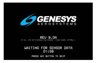
Figure 2-7: Two-Minute Countdown Screen (CPM5L)
