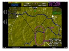
Once established in holding and ATC issues clearance for the KHIO ILS RW13R press CONT (L6) to continue the approach.
