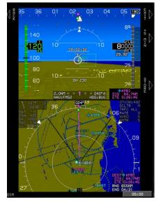
6) +5 MIN (R2) and STORE (R4) appear as shortcuts to quickly increase or decrease by 5 minute increments. Push ● to enter the default 05:00 countdown timer or press +5 MIN (R2) as many times as necessary to set the countdown timer. (Maximum time is 59 minutes and 59 seconds.)
