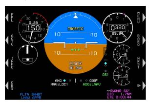
Figure RD-37: EFIS Coupled Vertically with Glide Slope Mode
