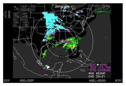
Figure D-2: Datalink Symbology with NEXRAD On
