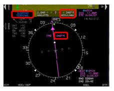
Indications of FMS being the source of navigation in manual OBS mode are shown in red rectangles.
