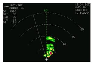
Figure WX-5: Radar Image in Arc Format
