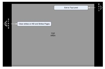
Figure S-8: MFD First-Level Menu in Normal Mode
