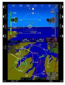
8) A magenta line leads from - DIR- current position to 3 OCSIP, which is now the active waypoint. 1500' is the VNAV altitude, and aircraft is flying in the HITS boxes.
