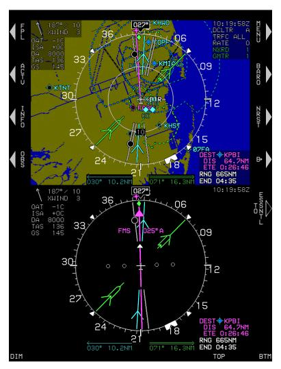
Figure 3-3: MFD in Normal Mode with MAP Page Displayed on Top and HSI on Bottom
