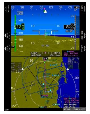
Figure 5-35: Fuel Totalizer Quantity Setting (SET FUEL) Menu
