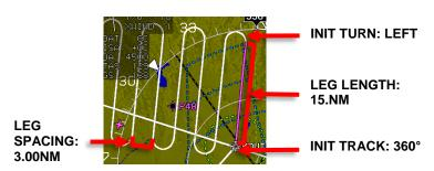
Figure SAR-7: Rising Ladder Pattern-Turn, Leg, and Track
