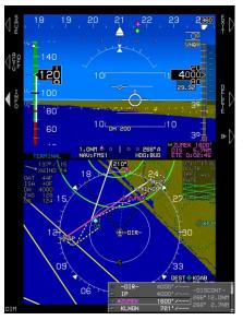
9) § Press ACTV (L2), rotate ● to ZUMEK, press → (R4), and then press EXIT.
