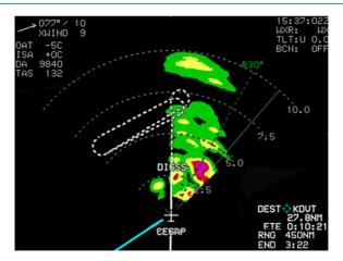
Figure WX-11: Radar Active Flight Plan
