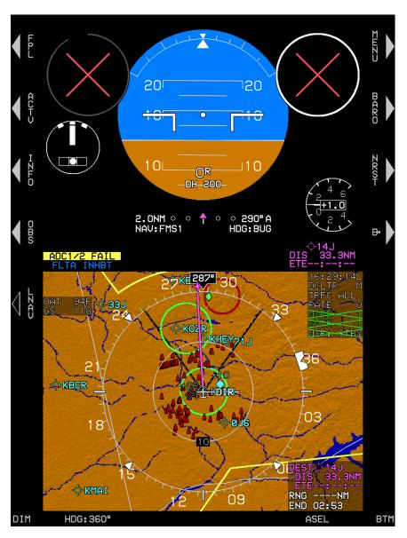
Figure RD-43: PFD Mode 2 ADC Failed, GPS/SBAS and AHRS Normal
