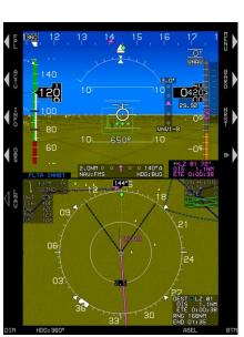
17) This view represents uncoupled maneuvering to the right base leg for the VFR approach. Vertical planning for turning final below the glide slope appears adequate for being level upon reaching the top of descent point.
