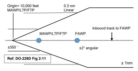
Figure 7-16: FSD Lateral Deviation Indicator Linear Deviation VTF
