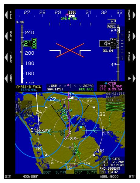
Figure 4-15: PFD Failure Mode 3 AHRS Failed, GPS/SBAS and ADC Normal
