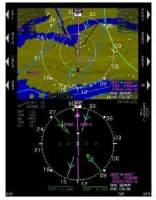
On MFD, press (R5) to display PFI on top and the last selected MFD mode on bottom.
