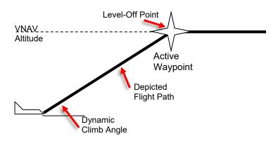
Figure 7-6: Highway in the Sky (Geo-Referenced Forward)
