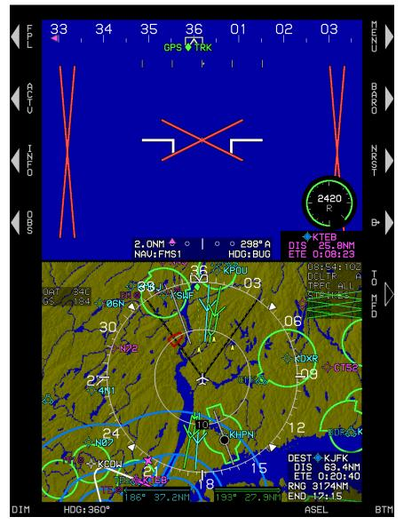
Figure 4-26: MFD Failure Mode 6 (Essential Mode) ADC and AHRS Failed, GPS/SBAS Normal
