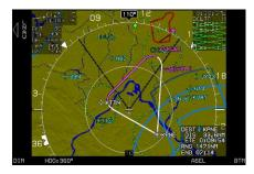
On this radar vector leg, no HITS boxes (guidance) are visible until intercepting the active leg.
