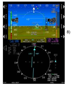
) Inside **2.0 NM** final with FLTA INHBT indicating no TAWS alerts are triggered and the default GPS LNAV APPR mode is active.
