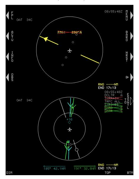
Figure 4-28: MFD Failure Mode 7 (Normal Mode) GPS/SBAS, ADC and AHRS Failed
