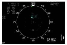
13) Press **MENU (R1)**, within 10 seconds press **FORMAT (R8)** to format the Traffic page on bottom.
