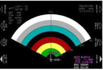
Press ACLTR ON (L2) to toggle anti-clutter option between ON and OFF.
