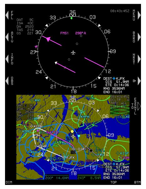
Figure 4-16: MFD Failure Mode 3 (Normal Mode) AHRS Failed, GPS/SBAS and ADC Normal
