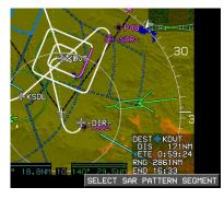
Rotate • to desired leg for navigation guidance.
