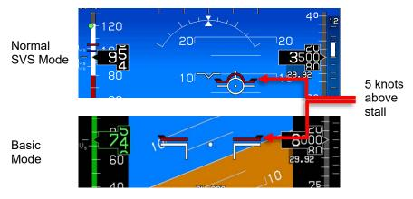
Figure 3-36: Pitch Limit Indicator (5 Knots above Stall)
