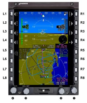
Figure 1-1: IDU-680 Input Identification
