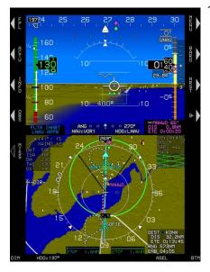
13) Established at 130 KIAS on short final with the runway in sight 0.8 NM ahead at the same horizontal angle as shown on the instrument approach chart.
