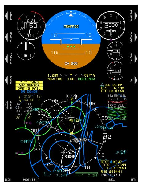
Figure RD-42: PFD Failure Mode GPS/SBAS Failed, ADC and AHRS Normal
