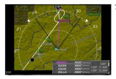
ATC issues clearance to "proceed to DUCKA 2 and hold as published maintain 4500' expect further clearance at (XXXX)." Rotate • to the first DUCKA and then push to enter.
