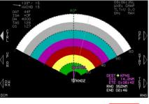
Press ON WX (L8) to resume normal weather radar mode of operation.
