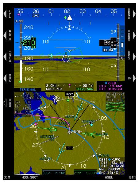
Figure 4-7: PFD Failure Mode 0 GPS, ADC and AHRS Normal
