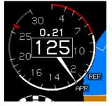
Figure RD-12: Takeoff and Landing Speed Bugs
