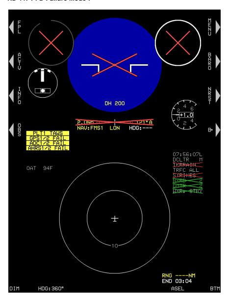
Figure RD-48: PFD Failure Mode 7 GPS/SBAS, ADC, and AHRS Failed
