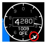
Altitude sub-mode user-selectable triangular target altitude bug shown here at 4,400'. The bug is limited to -1,000' up to 50,000' and is removed when more than 500' away from current altitude.
