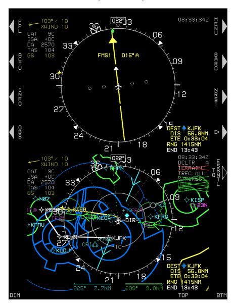
Figure 4-10: MFD Failure Mode 1 (Normal Mode) GPS/SBAS Failed, ADC and AHRS Normal
