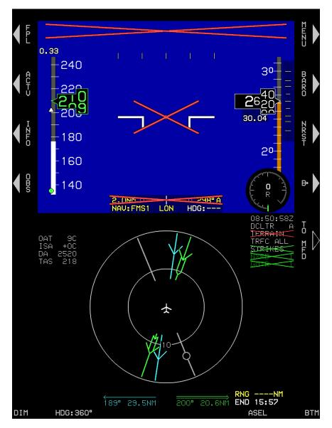
Figure 4-23: MFD Failure Mode 5 (Essential Mode) GPS/SBAS and AHRS Failed, ADC Normal
