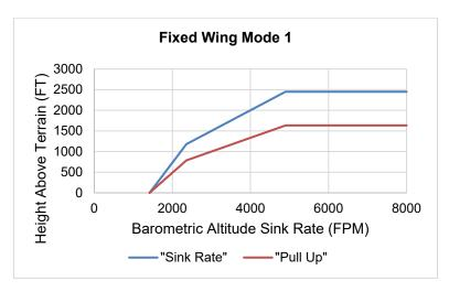
Figure 8-9: Fixed Wing GPWS Mode 1
