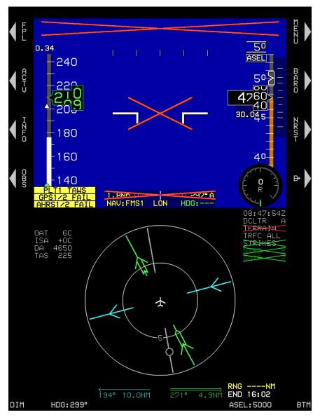
Figure 4-21: PFD Failure Mode 5
