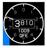
The altitude readout digitally displays barometric altitude to the nearest ten feet as adjusted by an altimeter setting and shows a 1000-foot range with labels and graduations every 100 feet. Clockwise rotation of the pointer corresponds to increasing altitude. All graduations are removed when below sea level.
