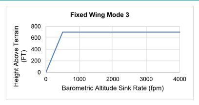
Figure 8-12: Fixed Wing GPWS Mode 3
