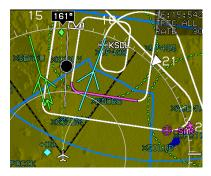
Figure SAR-4: Expanding Square Pattern-Individual Leg Selected
