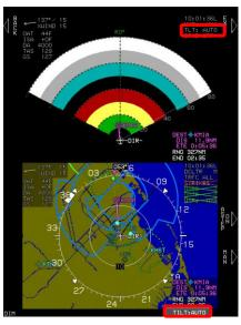
14) When in tilt auto mode, annunciation is above and in upper right corner of the top area.
