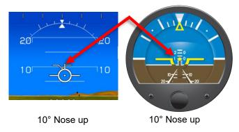
Figure 3-33: Pitch Scale
