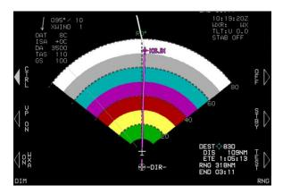
Figure WX-10: Radar Track Line with Menus
