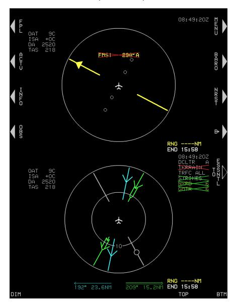
Figure 4-22: MFD Failure Mode 5 (Normal Mode) GPS/SBAS and AHRS Failed, ADC Normal
