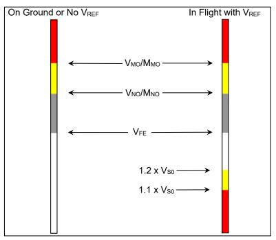
Figure 3-29: Airspeed Scale FAR Part 25
