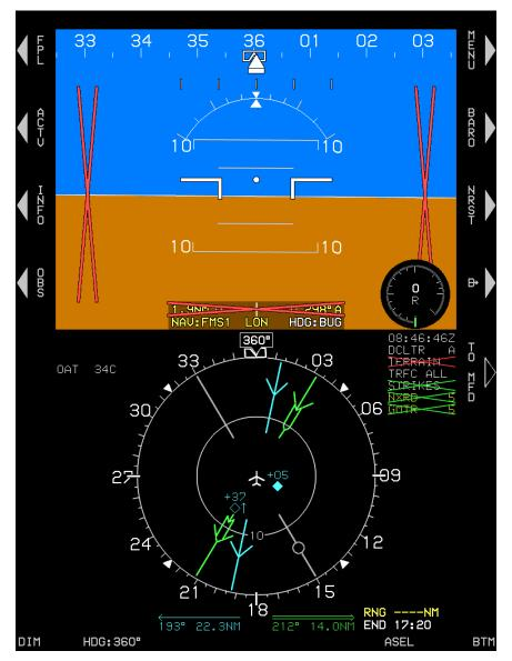
Figure 4-20: MFD Failure Mode 4 (Essential Mode) GPS/SBAS and ADC Failed, AHRS Normal
