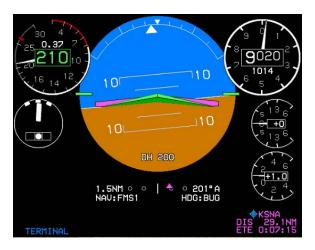
Figure RD-1: Pitch Scale
