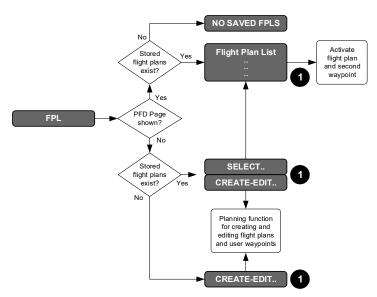
Figure 5-12: Flight Plan Menu (PFD or MFD)
