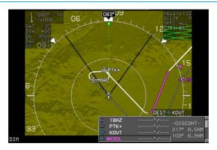
Figure 7-12: Parallel Offset PTK+/PTK ENTRY
