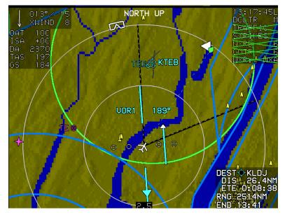
Figure 3-69: North-Up Arc Mode with HSI Enabled and VOR1 Selected
