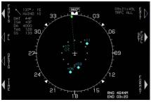
On the MFD, push ● and rotate to TRAFFIC and push to enter to display Traffic page on bottom.
