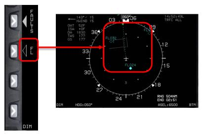
Figure T-14: Flight Level Option
