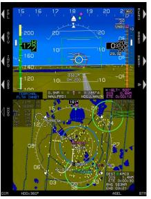
During the missed approach, the navigation source automatically switches to FMS1 with 0.3NM FSD. FLTA is still inhibited and terminal mode is active while within the terminal area.
