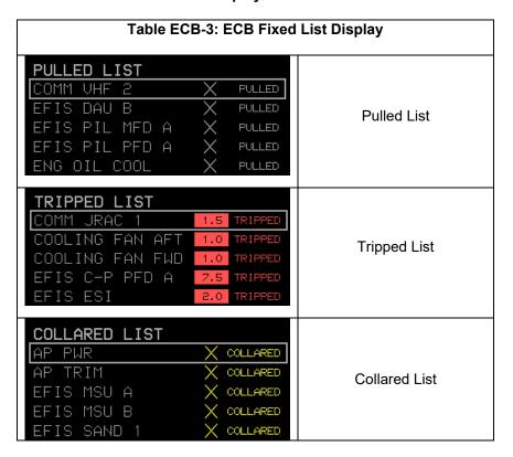
Electronic circuit breaker screen can show a fixed list based on its current breaker state using menu options. At least one ECB element is needed in the corresponding list for showing it on the screen.
