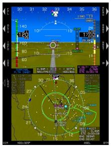
Past the MAWP, NAV source remains FMS and scale automatically changes to 0.3NM FSD.
