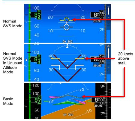
Figure 3-35: Pitch Limit Indicator (20 Knots above Stall)
