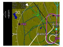
With no other menus displayed, **CONT** (L6) appears for continuing out of the racetrack and normal sequencing in the active flight plan.
