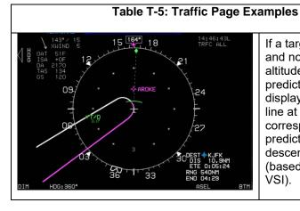
If a target altitude is set and not captured, an altitude capture predictor arc is displayed on the lubber line at a point corresponding with predicted climb or descent distance (based upon current VSI).
