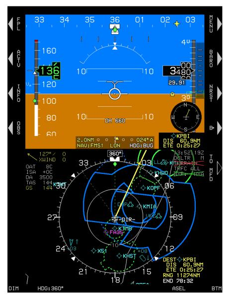
Figure 4-11: MFD Failure Mode 1 (Essential Mode) GPS/SBAS Failed, ADC and AHRS Normal
