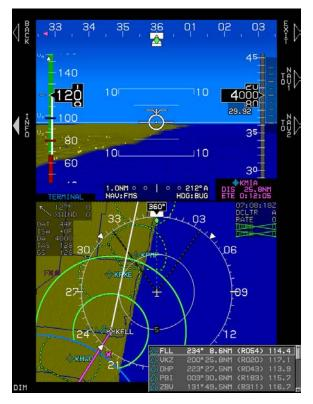
Figure 5-17: Remote Tuning NAV Radios
