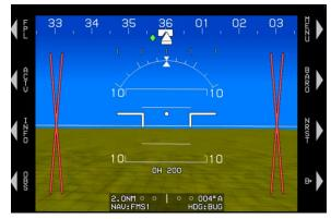
Single System ADC Failure (Red X's Only)
