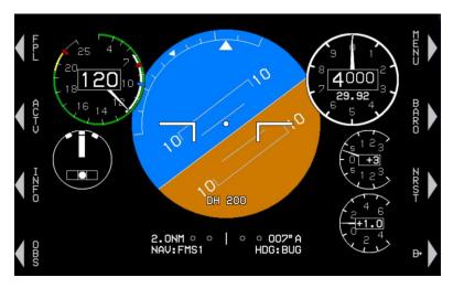
Figure RD-5: Bank Angle Scale Roll Pointer Type
