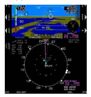
Figure T-8: Traffic Display Format
