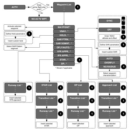
Figure 5-14: Active Flight Plan Main Menu
