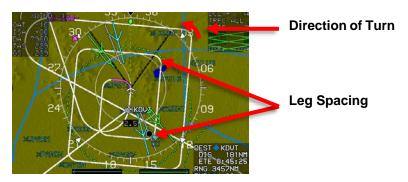
Figure SAR-3: Expanding Square Pattern-Turn and Leg
