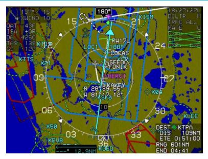
Figure 3-68: Moving Map with Instrument Approach with HSI Enabled
