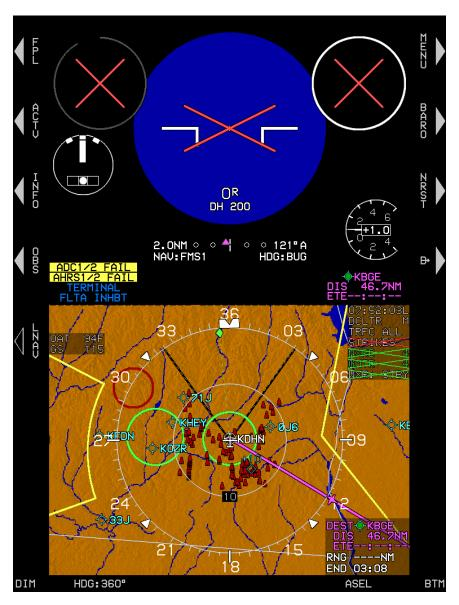
Figure RD-47: PFD Failure Mode 6 ADC and AHRS Failed, GPS/SBAS Normal
