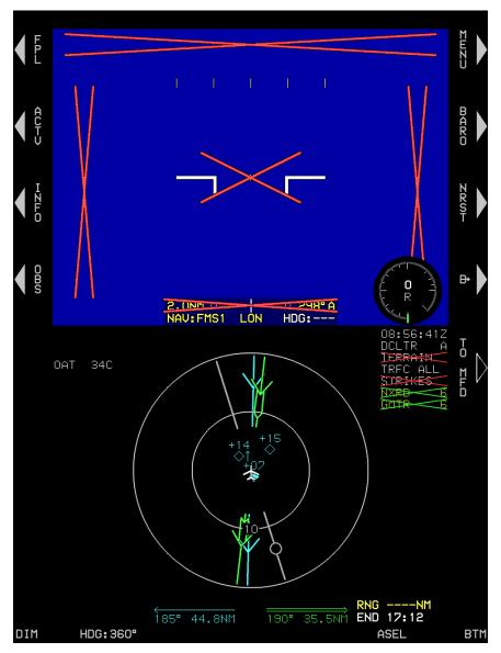
Figure 4-29: MFD Failure Mode 7 (Essential Mode) GPS/SBAS, ADC and AHRS Failed
