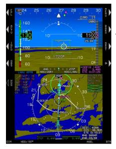
11) Established inbound on the final approach course to the FAF (SOFIE) 5 crossing top of descent symbol ahead indicating when descent can be commenced to cross the FAF at 1400'. Nav source is VOR1 and HITS source is GPS. The primary lateral source is the VOR and DME for this instrument approach.
