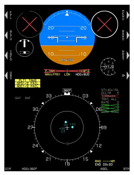
Figure RD-45: PFD Failure Mode 4 GPS/SBAS and ADC Failed, AHRS Normal
