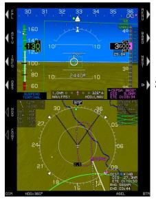
23) Sestablished in hold at CEPGA. Press CONT (L6) to continue waypoint sequencing to next leg in active flight plan.
