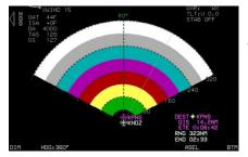
16) Rotate • to alter range of weather radar from 5.00 NM to 320.00 NM. Rotation direction dependent upon EFIS limits setting.
