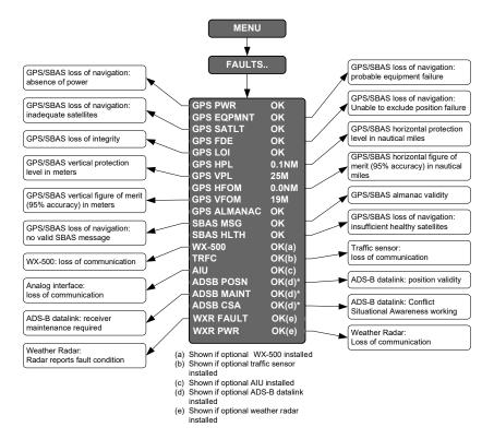
Figure 5-32: MFD Fault Display Menu
