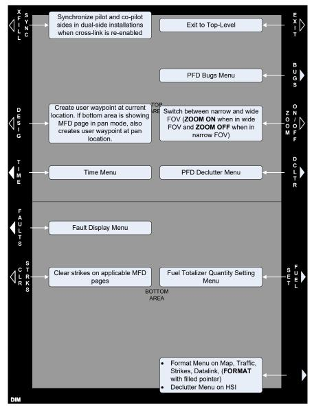
Figure 5-9: First-Level (PFD IDU #1) (PFI in Top Area and MFD in Bottom Area) (Normal Mode)
