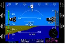
2) Press one of the following options: NRST APT (L2), NRST VOR (L3), NRST NDB (L4), NRST FIX (R2), NRST USR (R3), to view applicable list or create new waypoint with entering process for all five spaces and push to enter.
