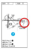
14) After passing the MAWPT and the missed approach procedure automatically sequenced, aircraft begins following the dashed magenta missed approach course lines on the MAP. NAV source automatically switched to FMS1 and 1.0 NM FSD.
