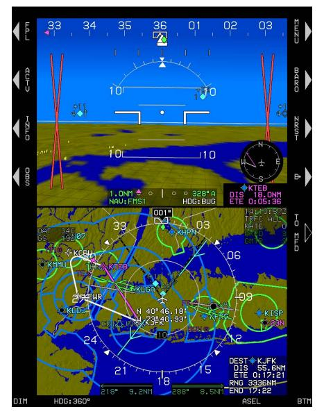
Figure 4-14: MFD Failure Mode 2 (Essential Mode) ADC Failed, GPS/SBAS and AHRS Normal
