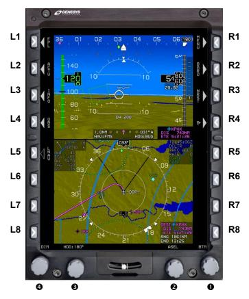
Figure 5-1: IDU-680 Input Controls
