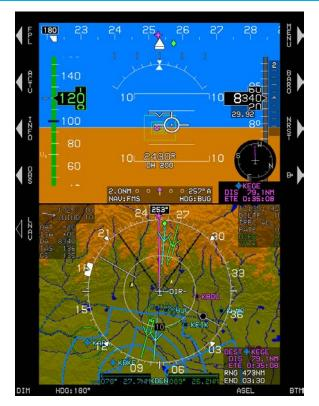
Figure 3-45: PFD with Terrain Deselected but Retained on Map
