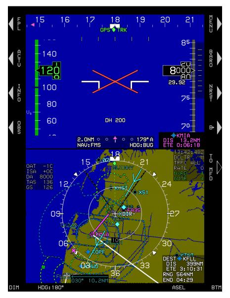
Figure 4-17: MFD Failure Mode 3 (Essential Mode) AHRS Failed, GPS/SBAS and ADC Normal
