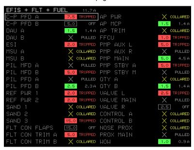
Figure ECB-1: ECBU Circuit Breaker Screen
