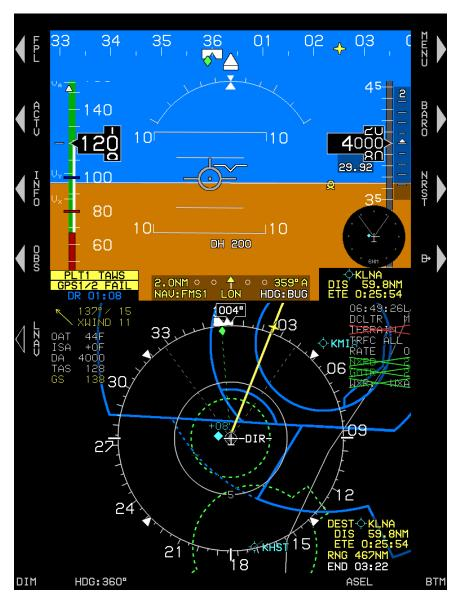
Figure 4-9: PFD Failure Mode 1 GPS/SBAS Failed, ADC and AHRS Normal
