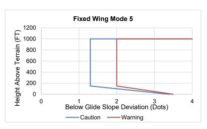
Figure 8-14: Fixed Wing GPWS Mode 5
