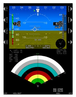
Figure WX-2: PFD Weather Radar Image on Bottom
