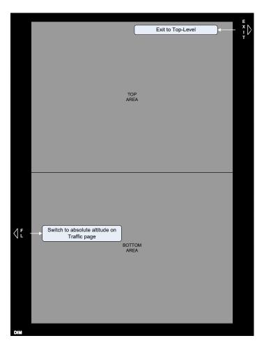
Figure T-6: PFD First-Level Menu in Normal Mode
