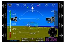
Active waypoint information, including waypoint type and identifier; elevation or crossing altitude; and along-track distance are displayed below the ANLG AGL, ANLG G, MINI MAP, or MINI TRFC indicator, as configured.
