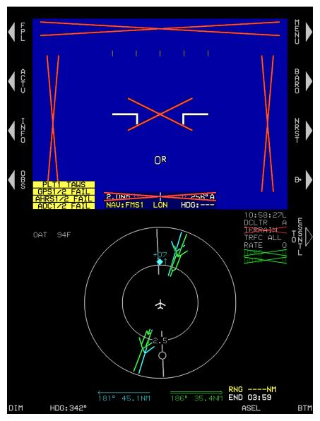
Figure 4-27: PFD Failure Mode 7 GPS/SBAS, ADC and AHRS Failed
