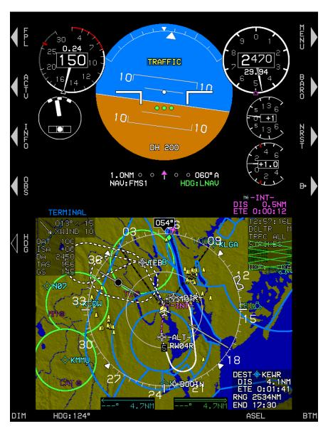
Figure RD-41: PFD Failure Mode 0 GPS, ADC and AHRS Normal
