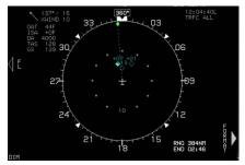
6) Press **MENU (R1)**, within 10 seconds press **FORMAT (R8)** to format the Traffic page on bottom.
