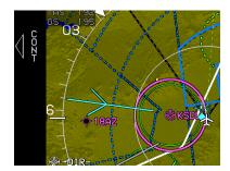
The SAR exit waypoint is a duplicate of the previous waypoint. This SAR pattern is unique in that the navigation path never goes through the waypoint. The path is a circle around the waypoint intercepted along tangents. With no other menus displayed on the PFD, CONT (L6) appears to allow for continuing out of the orbit and normal sequencing in the active flight plan.
