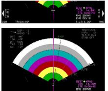
32) Press **GAIN** (R8) to open gain menu and rotate **①** to change gain in 1 dB increments. Push to set selected gain value.
