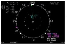
Traffic page scale is adjustable by rotating ● to select 3NM radius in 5NM and 10NM ranges.
