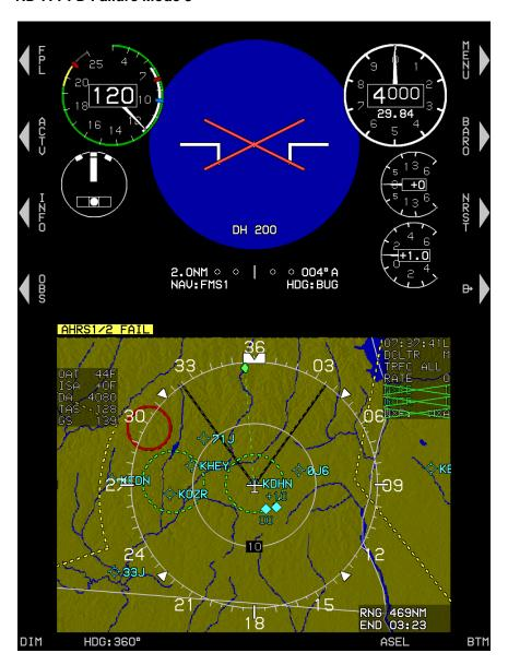
Figure RD-44: PFD Failure Mode 3 AHRS Failed, GPS/SBAS and ADC Normal
