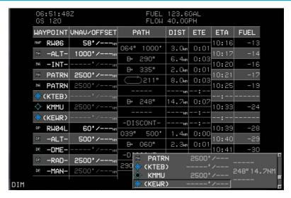
Figure 7-2: Active Flight Plan with Two Suppressed Waypoints
