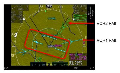
Figure 3-80: Analog Navigation Symbology, HSI in ARC Mode
