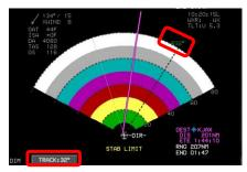
15) In the CTRL menu, push ❸ and rotate or begin by rotating to set new track angle in 1° increments between limits set in EFIS limits. Read new track in two places. Push ❷ to enter or press BACK (L1) to exit from track sub-mode.
