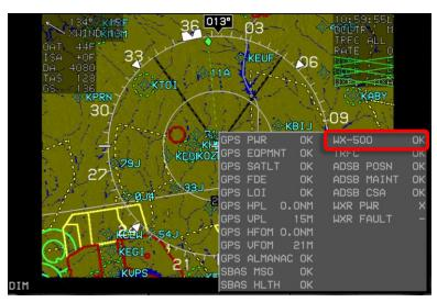
Figure S-10: MFD Fault Display Menu
