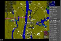
3) Rotate ● to LAT/LON and push to select. Either press EXIT (R1) or rotate ● to DONE and push to enter. If traffic is enabled, latitude/longitude display is removed when a traffic alert is present.
