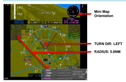
Figure SAR-11: Orbit Pattern-Turn and Radius
