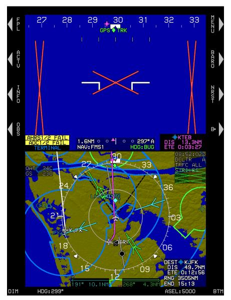
Figure 4-24: PFD Failure Mode 6
