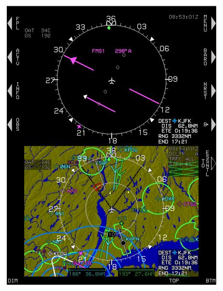
Figure 4-25: MFD Failure Mode 6 (Normal Mode) ADC and AHRS Failed, GPS/SBAS Normal
