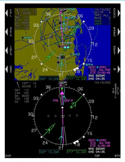
Figure 2-2: IDU-680 Multifunction Display (MFD)
