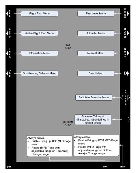
Figure 5-4: MFD Top-Level Menu (Normal Mode)
