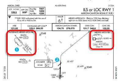
Figure 7-29: ILS or LOC RWY 1 Instrument Approach with Missed Approach Flown to Alternate fix (Step-By-Step)
