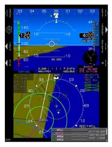
With active flight plan displayed, press INSERT (R2) to insert new waypoint above the highlighted line.
