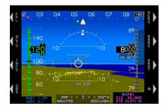
Rotate • to desired FSD and push to enter to view estimate of position uncertainty required in RNP airspace.
