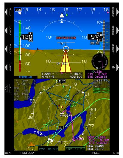
Obstruction within TAWS FLTA warning envelope with audible alert, "Warning Obstruction, Warning Obstruction."
