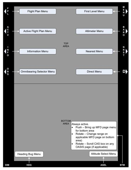
Figure 5-3: PFD Top-Level Menu (Normal Mode)
