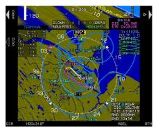
To change the HDG submode to HDG, press HDG
