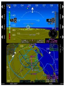
On MFD, press (R5) to display Map on top and HSI on bottom.
