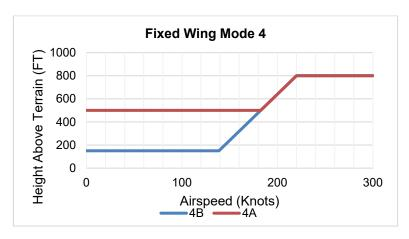
Figure 8-13: Fixed Wing GPWS Mode 4
