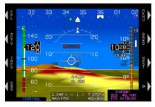
Indicated airspeed is on the left, altitude is on the right, and heading is across the top. FMS/VLOC CDI is located on the bottom. VSI appears on the right side of the altitude tape. Time-critical caution is displayed in the primary field of view.
