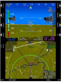
12) Navigation source automatically switches to FMS and FSD 0.3NM with HITS guidance clearly revealing anticipatory right turn ahead.
