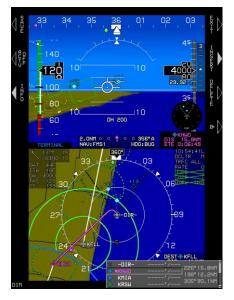
4) Press SAVE (L1), this action saves this active flight plan as one of the 100 saved flight plans in the system. This action is the same as creating a flight plan in the CREATE FLIGHT PLAN menu and pressing SAVE (R8). This action exits the Active Flight Plan menu.
