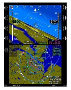
5) HDG bug sub-mode is now HDG BUG and LNAV (L5) appears for one touch changing back to LNAV submode. Partial HDG Bug is displaced beyond heading scale boundaries and shown at the heading scale limits.
