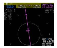
When there is an active waypoint and the GPS/SBAS OBS setting is manual, the course through the waypoint is shown as a pointer centered on the waypoint. The pointer matches the lateral navigation guidance on the PFD (GPS/SBAS CDI in manual OBS mode, skyway boxes, and mini map).
