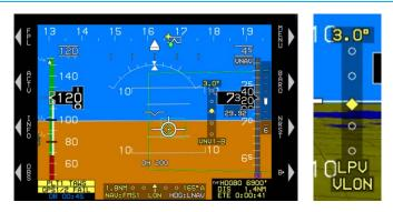
Figure 3-61: VDI Color during GPS/SBAS LON or VLON
