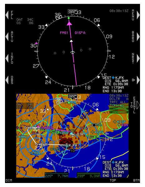
Figure 4-13: MFD Failure Mode 2 (Normal Mode) ADC Failed, GPS/SBAS and AHRS Normal
