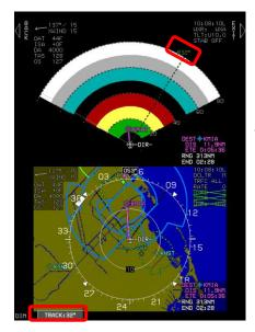
19) Push • and rotate or begin by rotating to set new track angle in 1° increments between limits set in EFIS limits. Read new track in two places.
