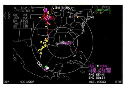
Figure D-1: Datalink Symbology with G METAR On
