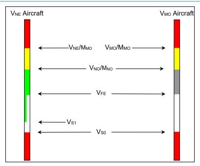
Figure 3-28: Airspeed Scale FAR Part 23
