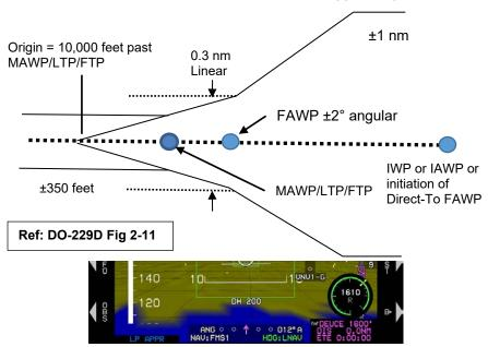
Figure 7-15: FSD Lateral Deviation Indicator Linear Deviation (not VTF Approach)
