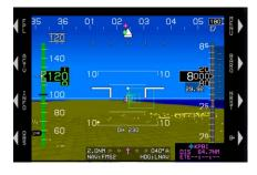
SVS TAWS terrain is now present. This setting is saved and retained during the next power cycle during initialization.
