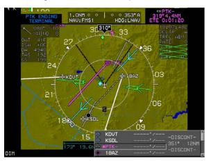
Figure 7-13: Parallel Offset PTK-/PTK ENDING
