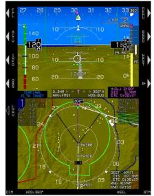
11) Passing the MAWP, navigation source automatically switches to FMS and **FSD 0.3NM**.
