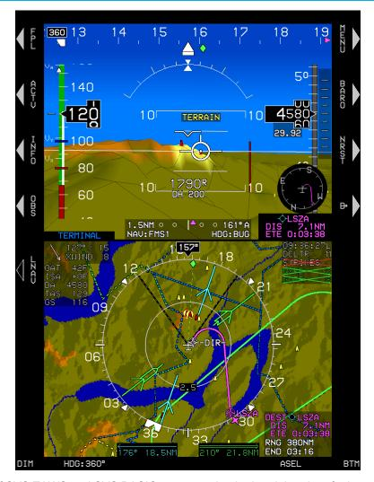
If SVS TAWS and SVS BASIC were not checked and the aircraft pierced the TAWS FLTA Terrain envelope, the EFIS automatically enables SVS TAWS. TERRAIN takes precedence over OBSTRUCTION.
