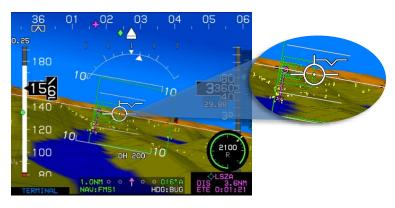
Figure 3-47: Flight Path Marker
