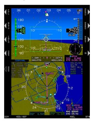
Figure 2-9: PFD PFI on Top and Map on Bottom
