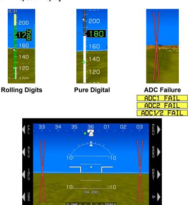
Single System ADC Failure (Red X's Only)
