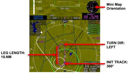
Figure SAR-14: Race Track Pattern-Turn, Leg, and Track
