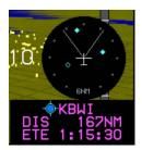
When selected from declutter options, thumbnail is displayed in the lower right corner of the PFI area of the PFD above the active waypoint identifier and has clock face markings fixed at the 6 NM scale.
