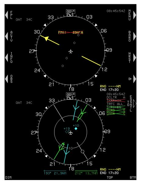
Figure 4-19: MFD Failure Mode 4 (Normal Mode) GPS/SBAS and ADC Failed, AHRS Normal
