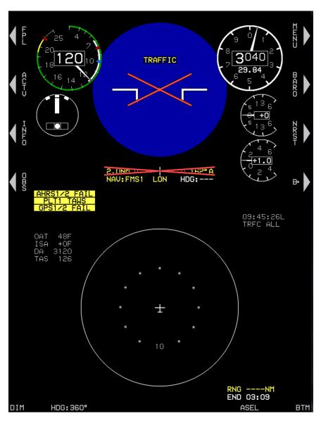
Figure RD-46: PFD Failure Mode 5 GPS/SBAS and AHRS Failed, ADC Normal
