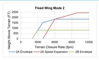
Figure 8-10: Fixed Wing GPWS Mode 2
