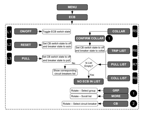
Figure ECB-6: Second Level ECB Control Menu
