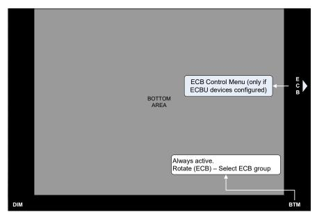
Figure ECB-5: Top-Level Menu (PFD/MFD Essential Mode/MFD Normal Mode)
