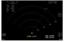
While in STBY mode, press ON WX (L8) to return radar to ON mode.
