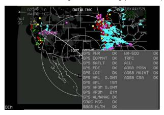
Figure D-11: FAULTS Menu with ADS-B Status
