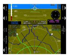
A manual termination leg has been created within a procedure and waypoint sequencing is suspended.
