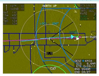
Figure 3-70: North-Up Centered Mode with HSI Enabled and VLOC1 Selected
