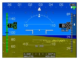
Figure 3-50: Flight Path Marker Absence
