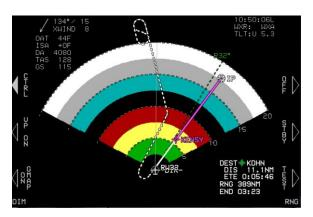
Figure WX-12: Radar Active Flight Plan with Menus
