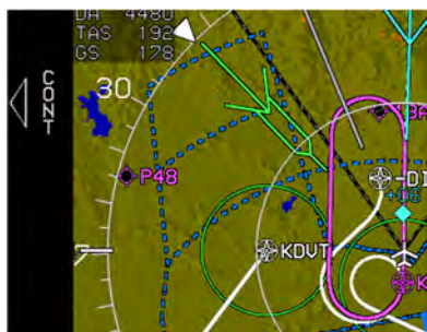
Figure SAR-12: Race Track Pattern
