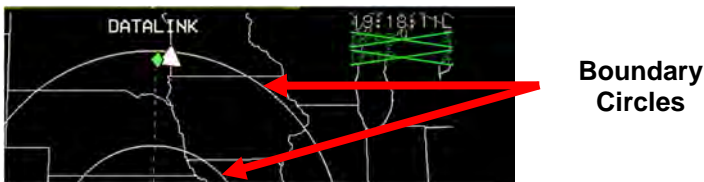
Figure D-9: Boundary Circle Symbol
