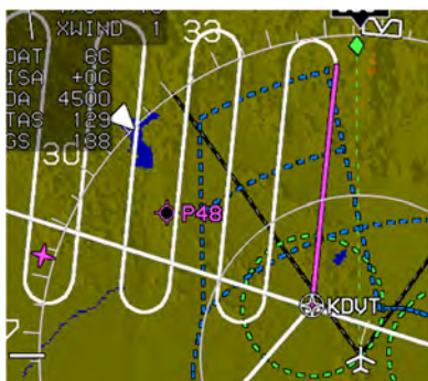
Figure SAR-5: Rising Ladder Pattern
