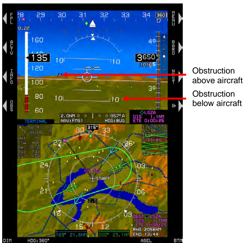
Figure 8-14: PFD SVS TAWS Option and Obstructions
