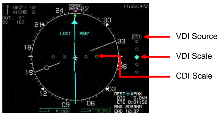
Figure 3-103: CDI Scale with VDI
