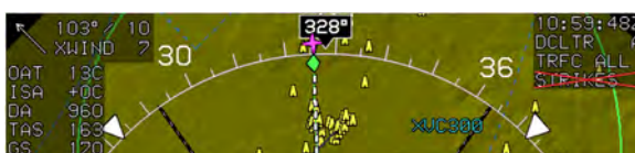
Figure 3-78: Compass Rose/ND Boundary Circle Symbol
