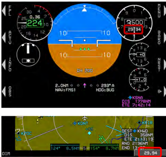
Figure RD-13: Altimeter Setting
