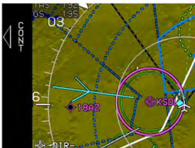
Figure SAR-9: Orbit Pattern
