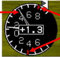
Figure 3-45: Analog G-Force Indicator
