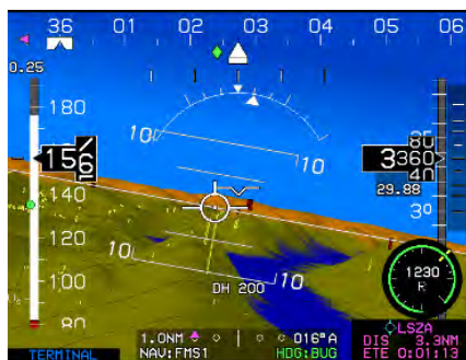
Obstructions without hazardous condition
