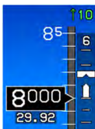
Figure 3-23: VSI Bug without Genesys/S-TEC DFCS
