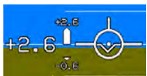
Figure 3-44: G-Force Indicator Telltale Indications
