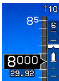
Figure 3-23: VSI Bug without Genesys/S-TEC DFCS
