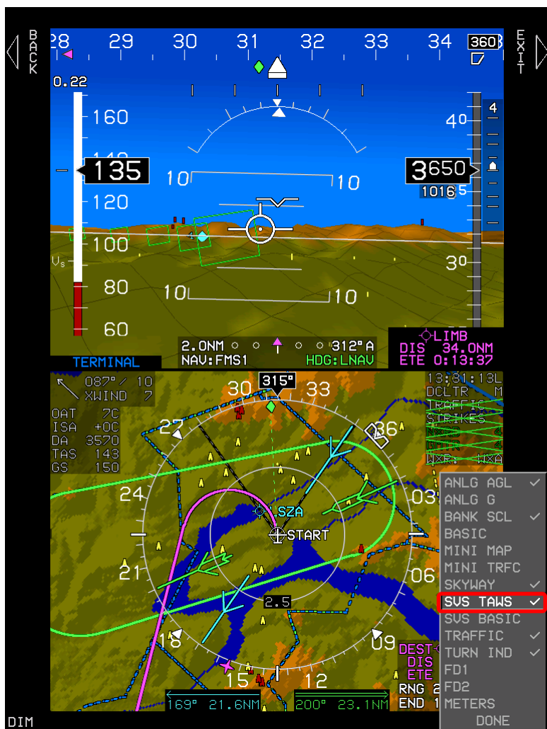
Figure 8-16: PFD SVS TAWS Option
