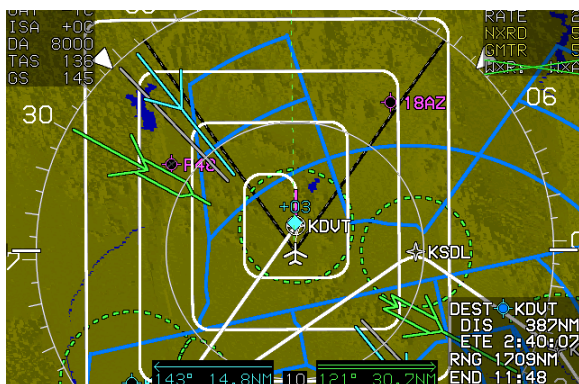
Figure SAR-1: Expanding Square Pattern
