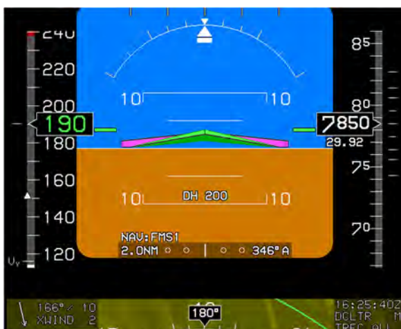
Figure 3-60: Flight Director FD1 (Basic Mode with Compass Rose Detected on MFD Page)
