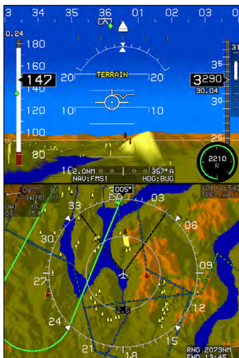
Figure 3-87: Terrain and Obstructions
