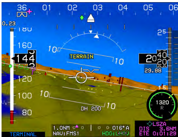
Figure 3-49: PFD Terrain and Obstructions
