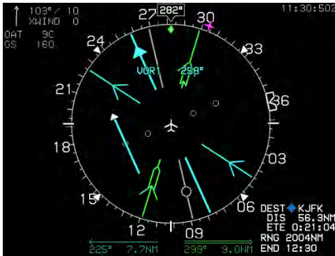
Figure 3-104: Analog Navigation Display VOR1 and VOR2
