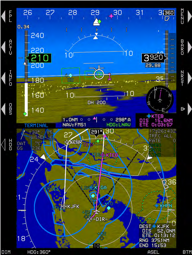
Figure 3-1: PFD Normal SVS Mode
