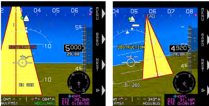
Figure 2-12: Time-Critical Warning and Caution Alerts
