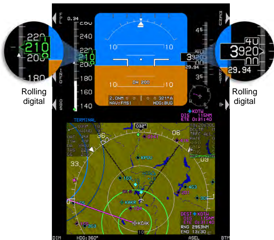
Figure 3-2: PFD in Basic Mode
