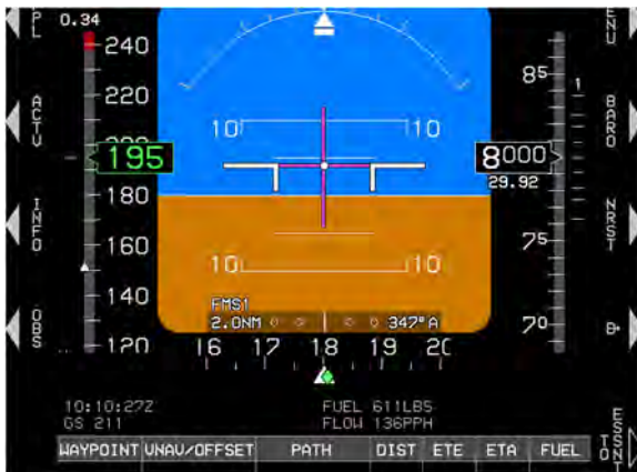
Figure 3-62: Flight Director FD2 (Basic Mode without Compass Rose Detected on MFD Page)
