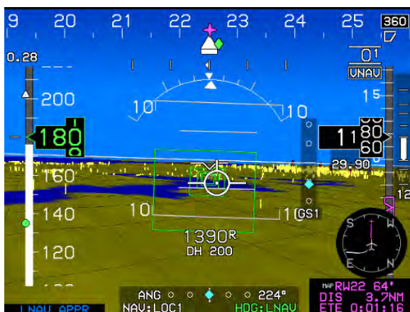
Figure 7-6: Highway in the Sky Final Approach Segments
