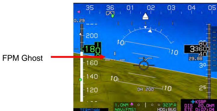
Figure 3-54: Flight Path Marker Ghost
