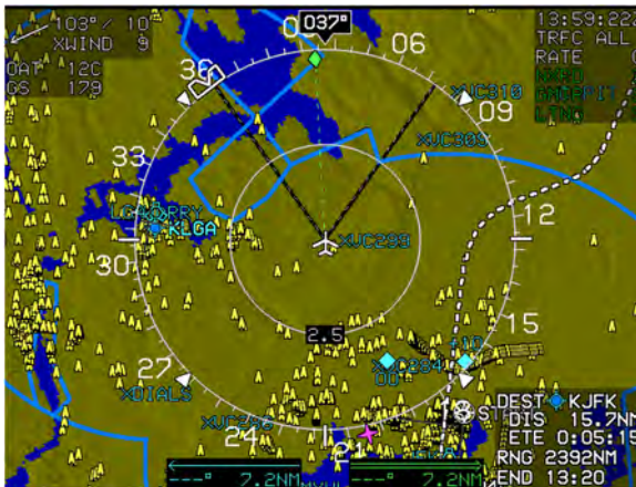
Figure 3-73: Basic Moving Map
