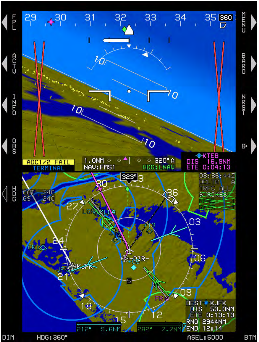
Figure 4-11: PFD Mode 2 ADC Failed, GPS/SBAS and AHRS Normal
