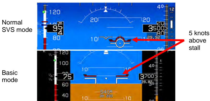
Figure 3-41: Pitch Limit Indicator (5 Knots above Stall)
