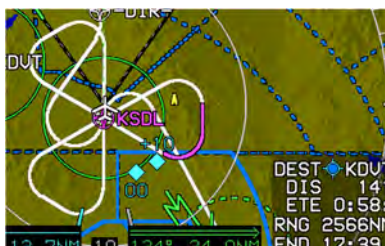
Figure SAR-18: Sector Search Pattern-Individual Leg Selected
