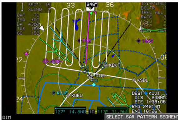
Figure SAR-8: Rising Ladder Pattern-Individual Leg Selected
