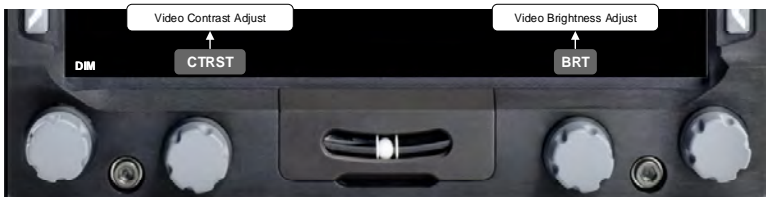
Figure V-1: First Page PFD Video Control
