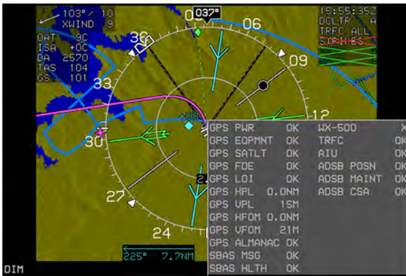
Figure 4-4: FAULTS Page on MFD
