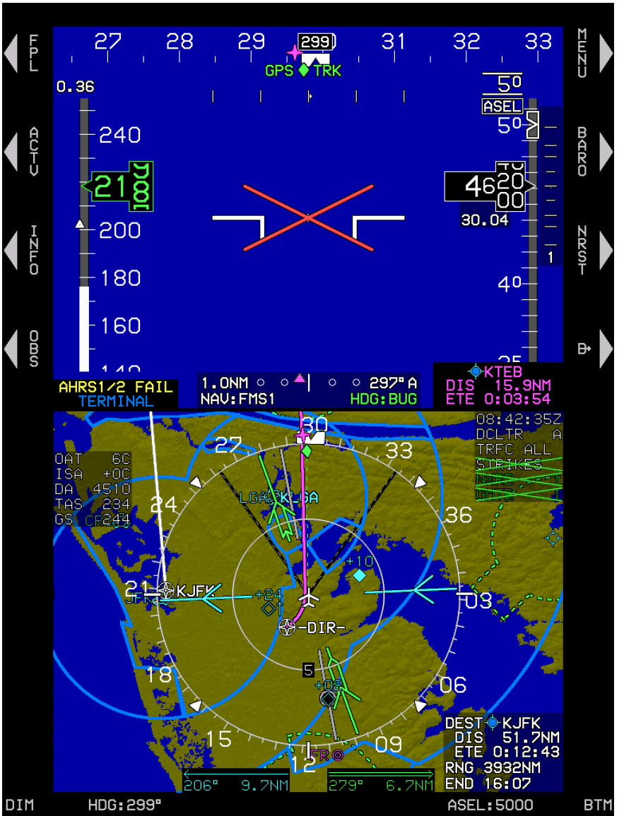
Figure 4-14: PFD Failure Mode 3 AHRS Failed, GPS/SBAS and ADC Normal
