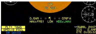
Figure RD-36: Course Deviation Indicator
