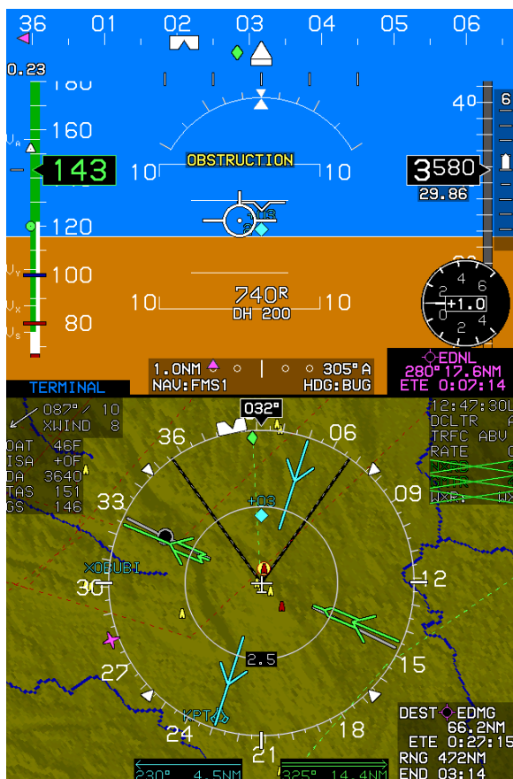
Figure 3-51: PFD with Terrain Deselected on PFD and Retained on the ND MAP
