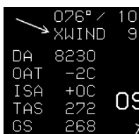
Figure 3-109: HSI Display Air Data and Groundspeed
