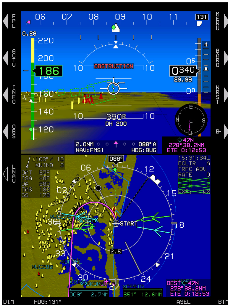
Obstruction within TAWS FLTA warning envelope with aural annunciation “Warning Obstruction, Warning Obstruction.” Obstruction symbols flash.
