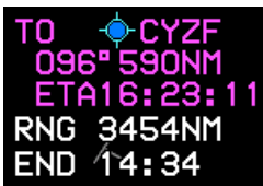
Figure S-5: Fuel Totalizer/Waypoint Bearing and Distance Functions
