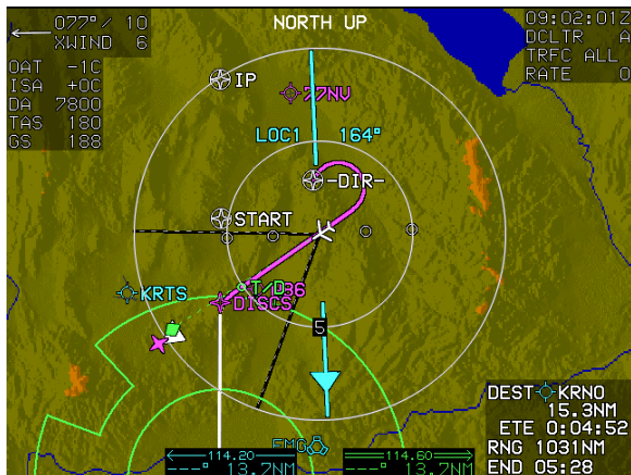
Figure 3-79: North-Up Centered Mode with HSI Enabled and VLOC1 Selected
