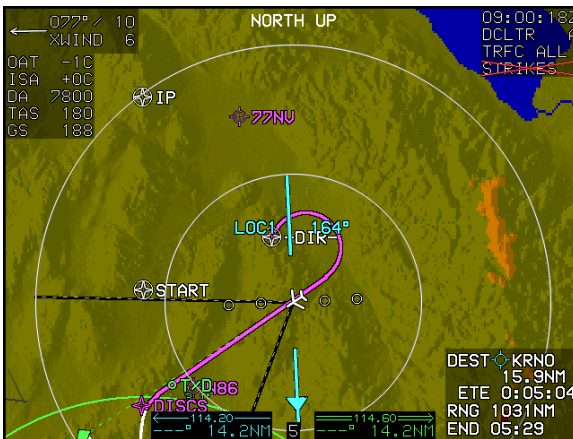
Figure 3-78: North-Up Arc Mode with HSI Enabled and VOR1 Selected
