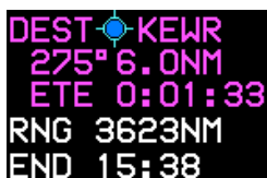
Figure T-7: Fuel Totalizer/Waypoint Bearing and Distance Functions
