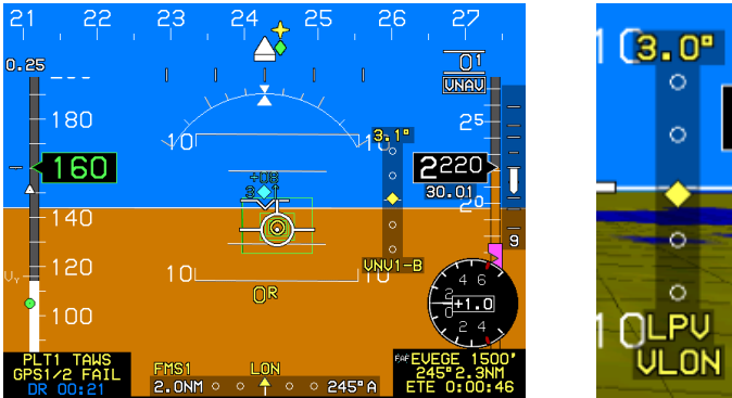
Figure 3-67: VDI Color during GPS/SBAS LON or VLN
