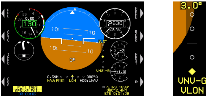
Figure RD-35: VDI Color during GPS/SBAS LON or VLON
