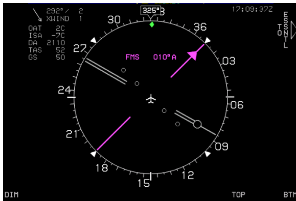
Figure 3-105: Analog Navigation Display FMS and ADF2
