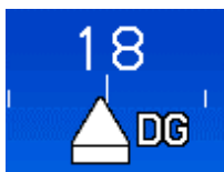
Figure 3-37: DG Indicated when AHRS in DG Mode
