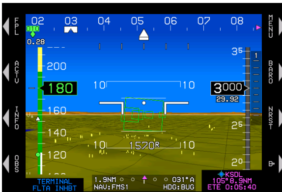
Figure 3-56: Flight Path Marker Absence
