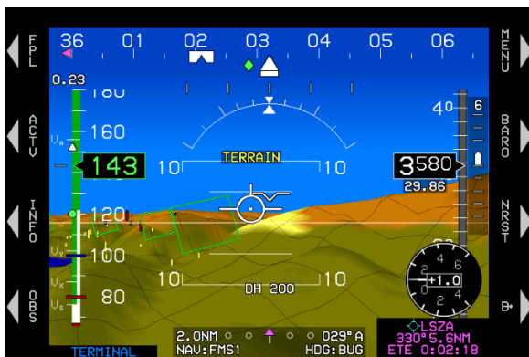
Figure 3-50: PFD Terrain and Obstructions
