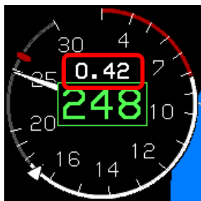
Figure RD-11: Airspeed Readout with Mach Number
