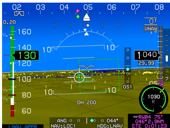
Figure 7-5: Highway in the Sky Final Approach Segments
