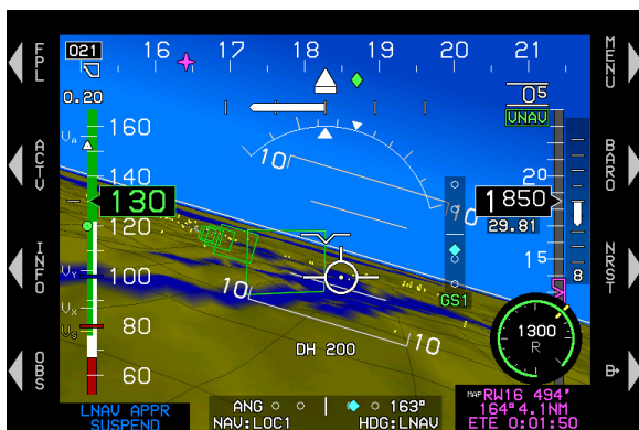
Figure 3-68: EFIS Coupled Vertically with Glideslope Mode
