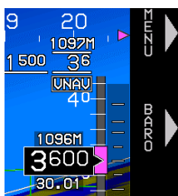
Figure 3-19: Altitude Display (Metric Units)
