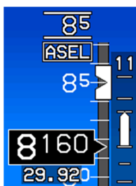
Figure 3-15: Target Altitude Bug (Without Autopilot)
