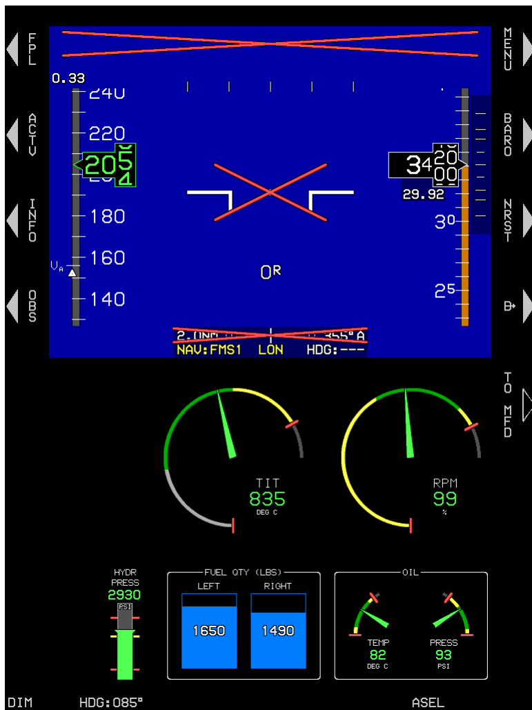
Figure 4-20: MFD Failure Mode 5 (Essential Mode) GPS/SBAS and AHRs Failed, ADC Normal
