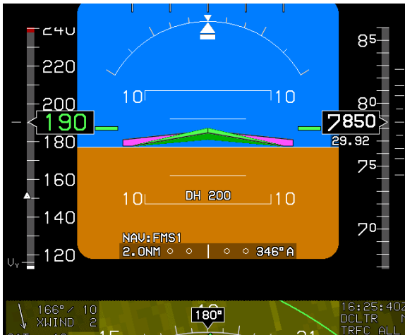
Figure 3-61: Flight Director FD1 (Basic Mode with Compass Rose Detected on ND)
