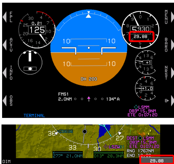
Figure RD-13: Altimeter Setting
