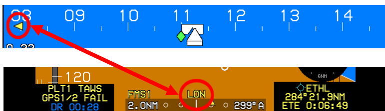
Figure 3-38: GPS Loss of Navigation (LON)
