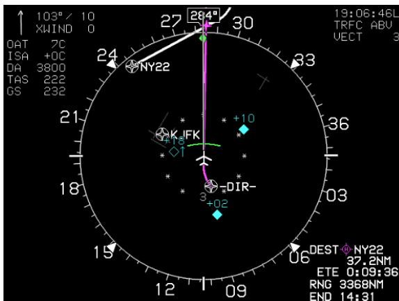
Figure T-4: Traffic Display Format
