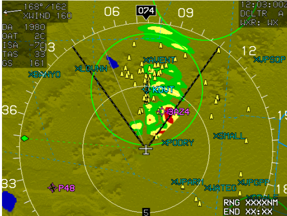
Figure WX-1: Weather Radar Image on ND
