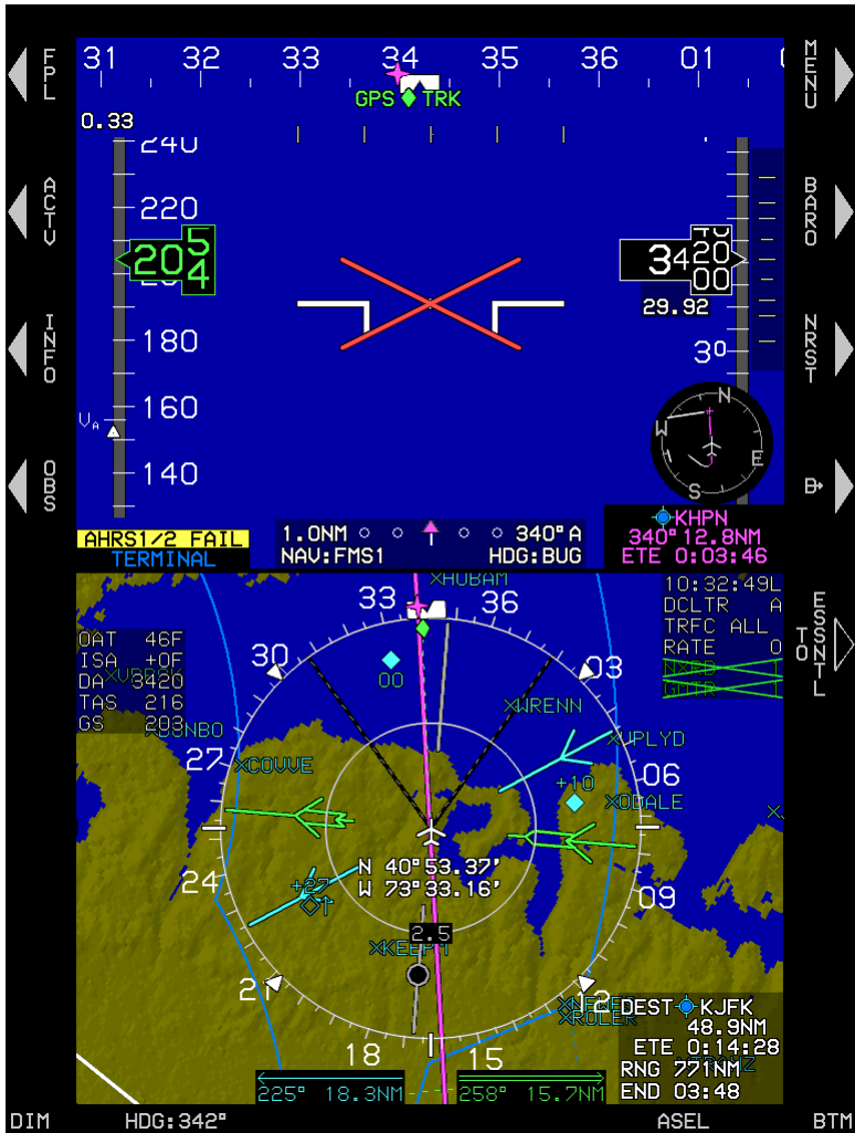
Figure 4-13: PFD Failure Mode 3 (Normal Mode) AHRS Failed, GPS/SBAS and ADC Normal
