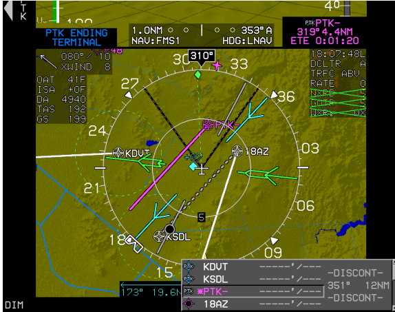
Figure 7-9: Parallel Offset PTK-/PTK ENDING
