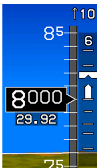
Figure 3-24: VSI Bug without Genesys/S-TEC DFCS
