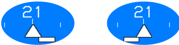
Figure 3-36: Dampened Integral Slip Indicator
