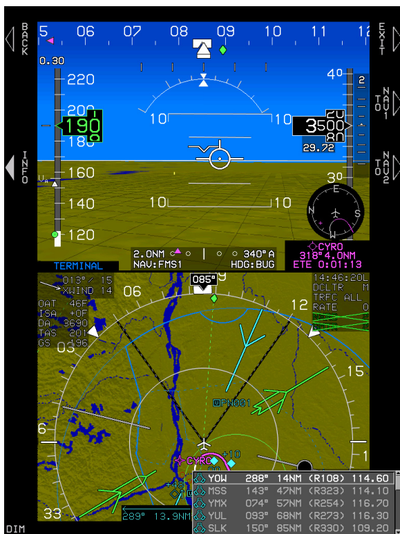
Figure 5-17: Remote Tuning NAV Radios
