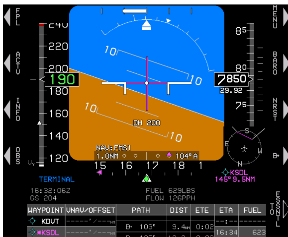
Figure 3-66: Flight Director FD2 (Basic Mode without Compass Rose Detected on ND) (Tapes)
