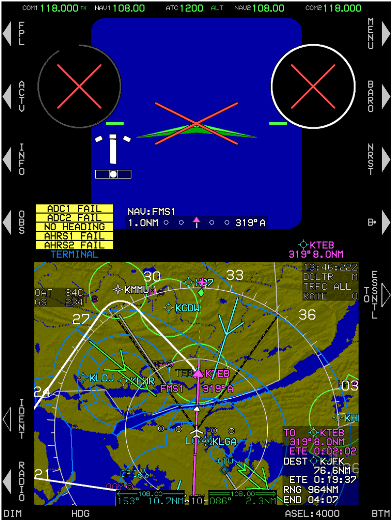
Figure 4-25: PFD Failure Mode 6 (Normal Mode) ADC and AHRs Failed, GPS/SBAS Normal (Round Dials)
