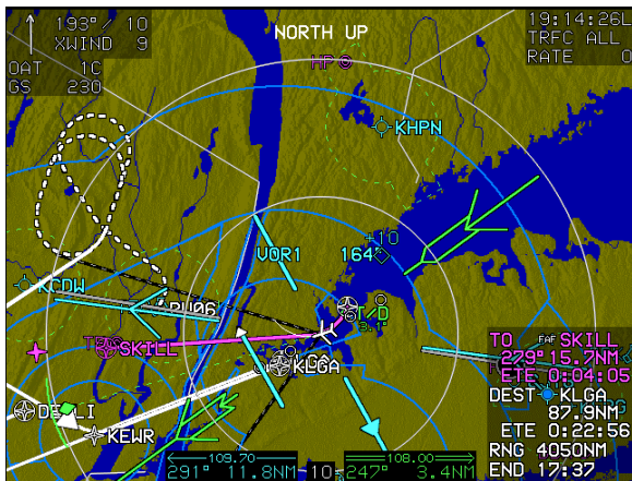
Figure 3-81: North-Up Arc Mode
