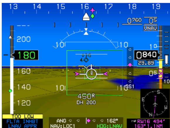
Figure 3-20: Minimum Altitude (Tapes)
