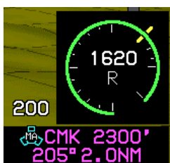
Figure 3-28: Analog AGL Indication
