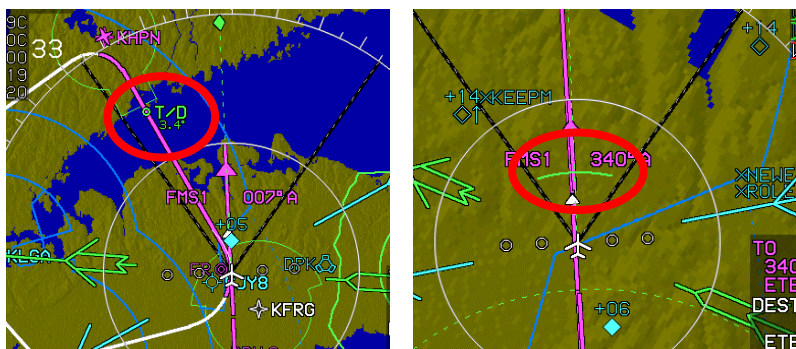
Figure 3-90: Top-of-Descent or Top-of-Climb
