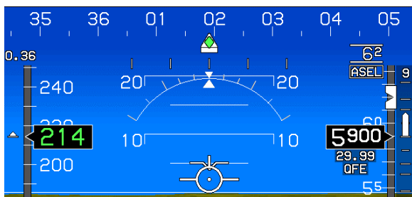
Figure 3-12: Altimeter QFE (Tapes)
