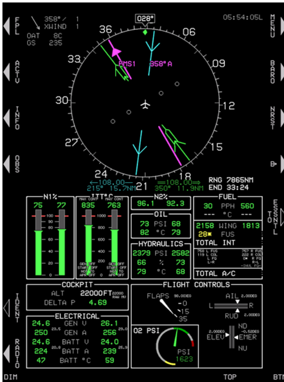
Figure 2-8: MFD with HSI and EICAS
