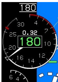
Figure 3-35: Airspeed Display (Round Dials)
