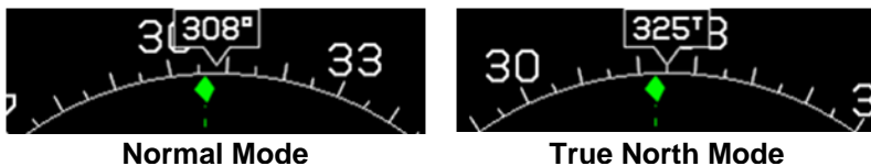
Figure T-4: Traffic Screen Range Compass Rose Symbols
