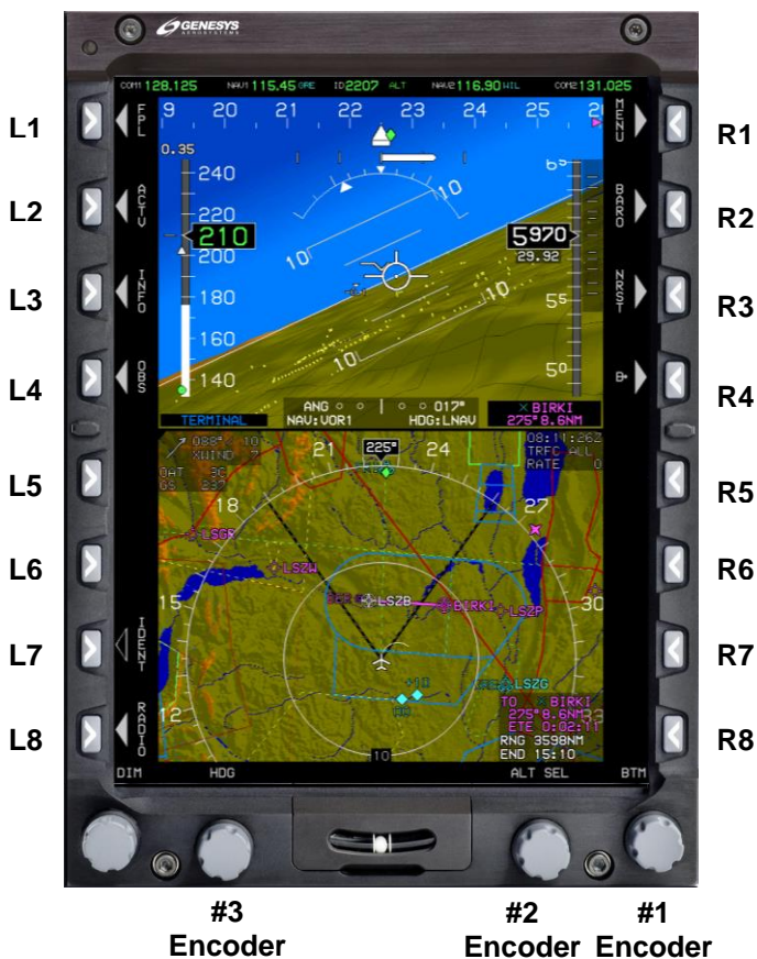
Figure 1-1: IDU-680 Input Identification
