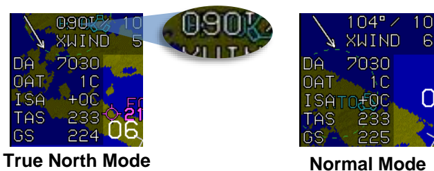
Figure 3-95: Air Data and Groundspeed
