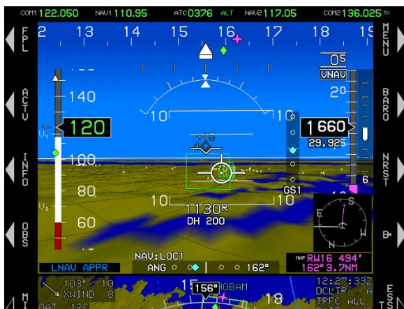
Figure 7-5: Highway in the Sky Final Approach Segments
