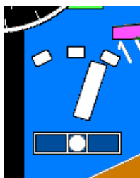
Figure 3-60: Turn Rate Indicator (Round Dials)
