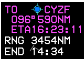
Figure S-5: Fuel Totalizer, Waypoint Bearing/Distance in Lower Right Corner
