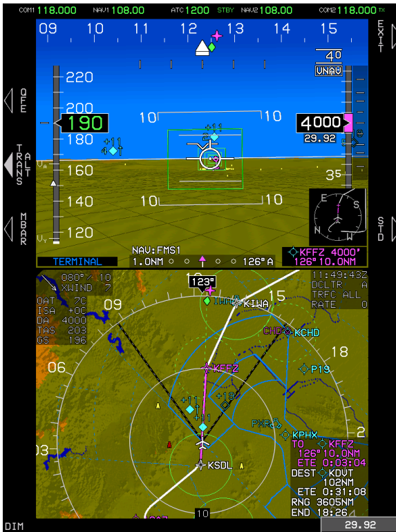
Figure 3-11: Altimeter Setting (Tapes)
