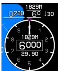
Figure 3-22: Metric Altitude (Round Dials)
