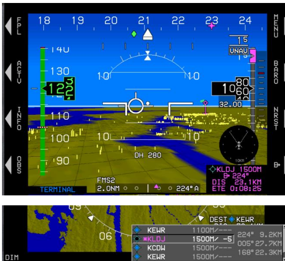
Figure 3-15: VNAV Sub-Mode (Not Vertically Integrated) (Meters for Altitude and KM for Distance)
