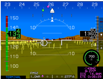
Obstructions without hazardous condition
