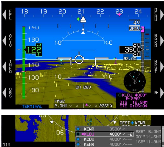
Figure 3-14: VNAV Sub-Mode (Not Vertically Integrated) (Feet for Altitude and NM for Distance)
