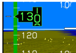
FPM removed due to excessive crosswinds from the right
