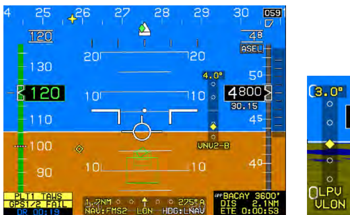
Figure 3-60: VDI Color during GPS/SBAS LON or VLON
