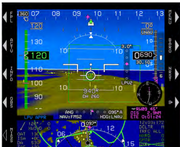
Figure 7-16: GPS Mode (LPV APPR)
