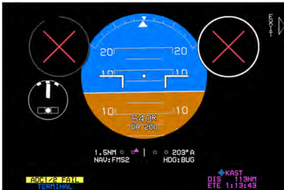
Figure RD-12: Airspeed and Altitude with Loss of ADC
