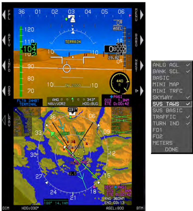
Figure 8-13: Terrain Display Functionality SVS TAWS
