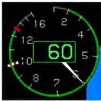
Figure RD-7: Airspeed Display with ADC Failure
