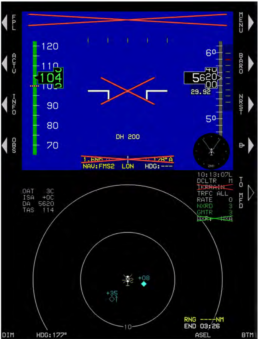
Figure 4-24: MFD Failure Mode 5 (Essential Mode) GPS/SBAS and AHRs Failed, ADC Normal
