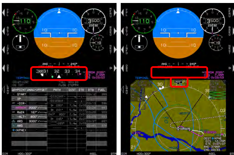
Figure RD-18: Heading Display
