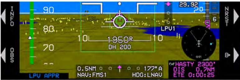
Figure 7-14: FSD Lateral Deviation Indicator Linear Deviation (not VTF Approach)
