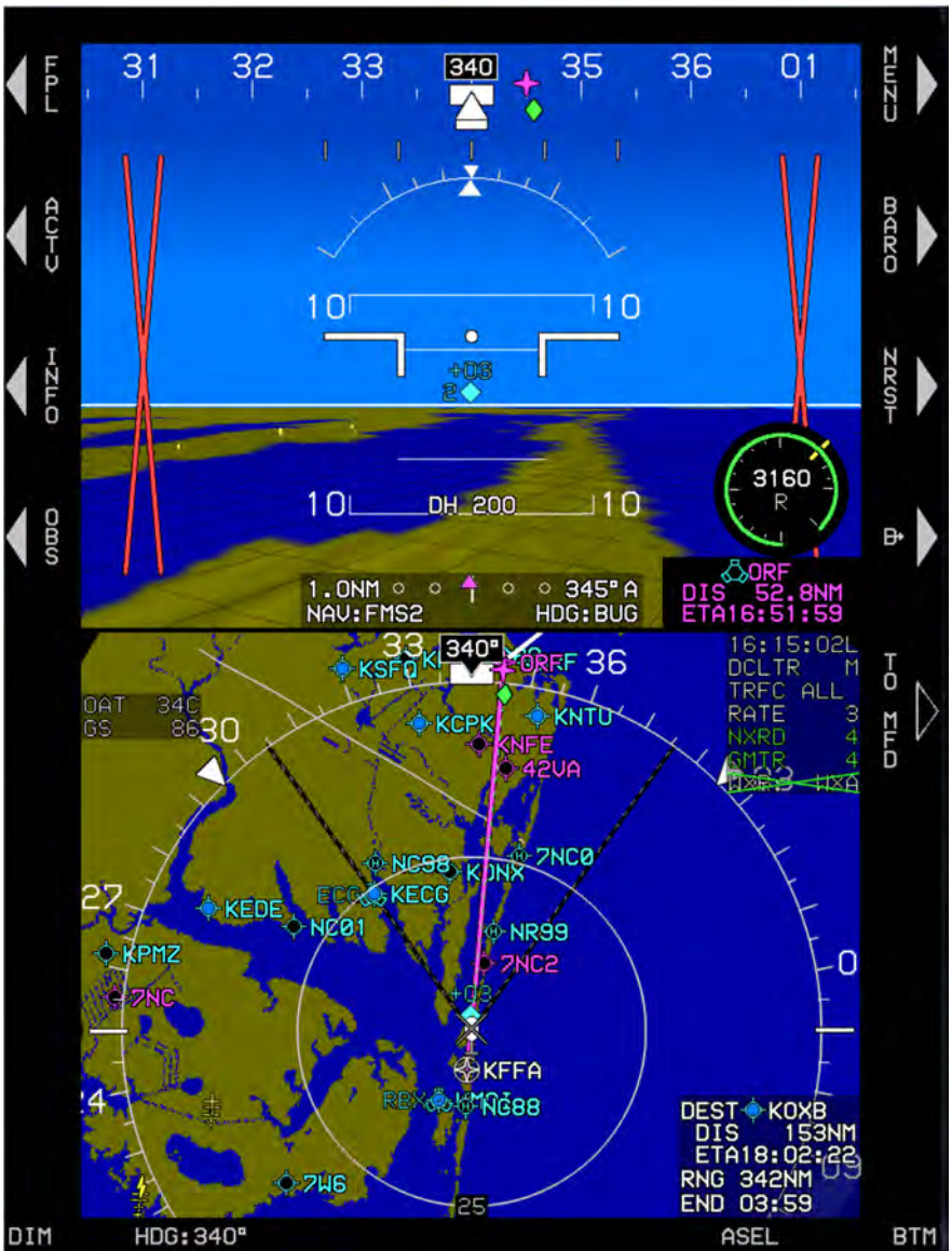
Figure 4-15: MFD Failure Mode 2 (Essential Mode) ADC Failed, GPS/SBAS and AHRS Normal
