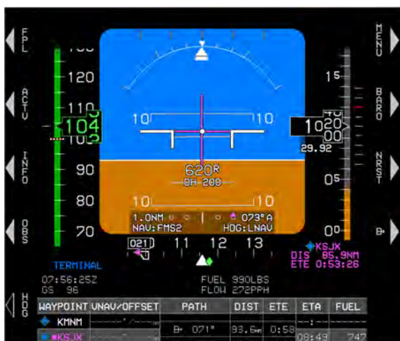
Figure 3-55: Flight Director FD2 Dual Cue (Basic Mode without Compass Rose Detected on Bottom Area)
