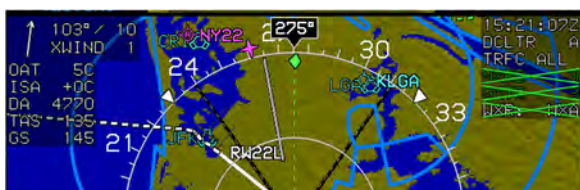
Figure 3-74: Compass Rose/ Boundary Circle Symbol
