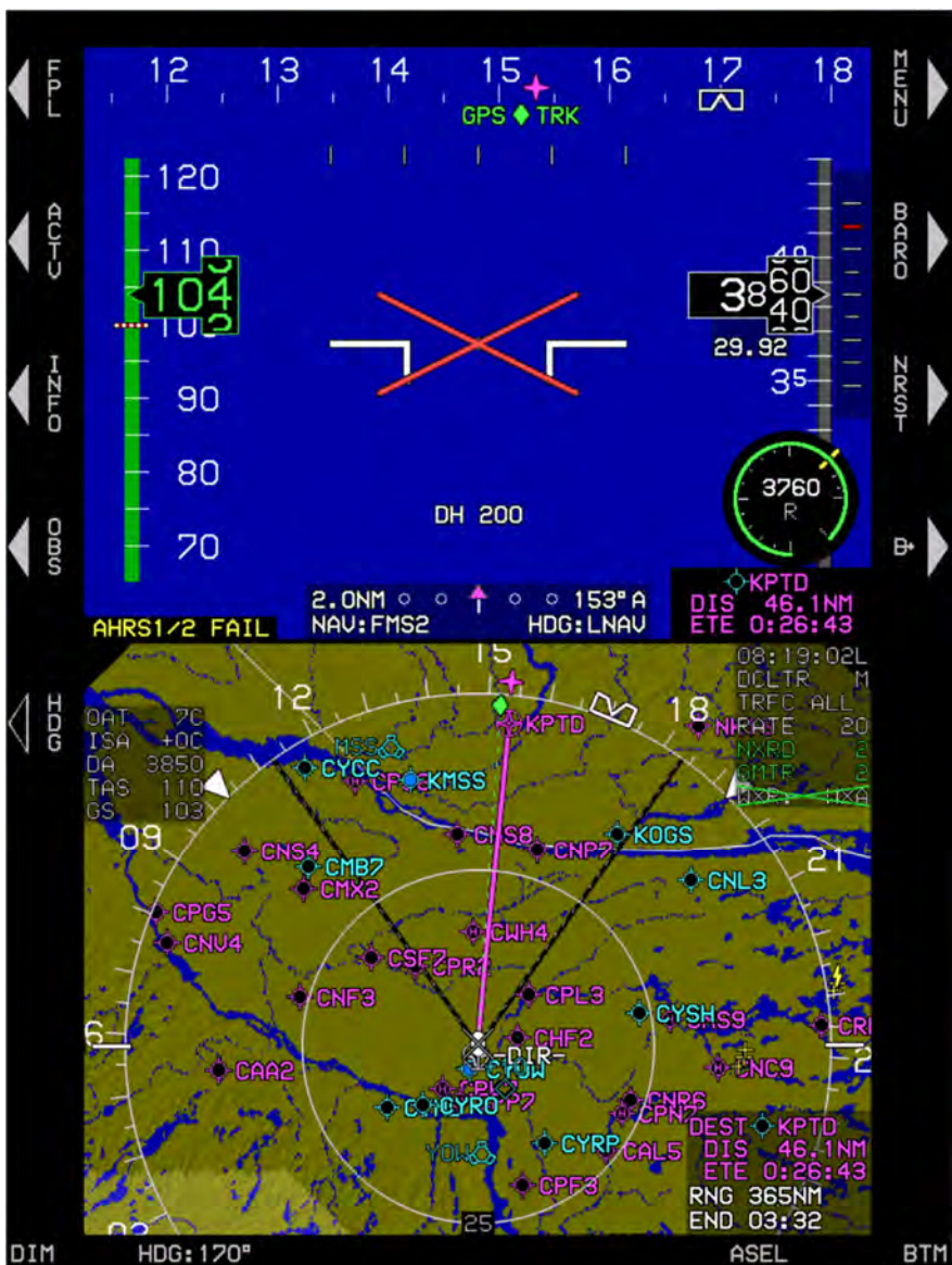
Figure 4-16: PFD Failure Mode 3 (Normal Mode) AHRs Failed, GPS/SBAS and ADC Normal
