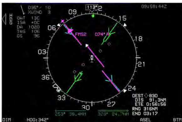
Figure 3-99: HSI Display Air Data and Ground Speed
