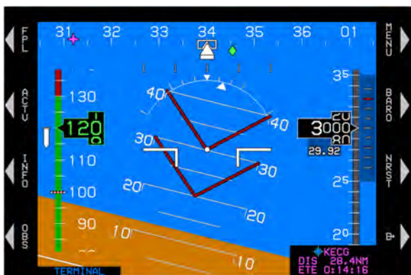
Figure 3-44: Flight Path Marker absent (Unusual Attitude Mode)
