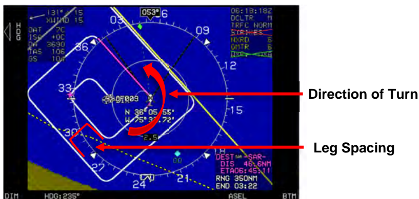
Figure SAR-1: Expanding Square Pattern Turn and Leg Spacing
