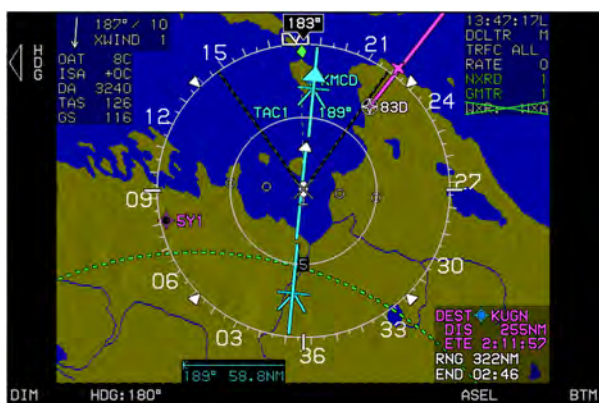
Figure 3-79: Analog Navigation Symbology, HSI overlay with Map in Centered Mode
