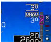
Figure 3-19: VNAV Sub-Mode (Vertically Integrated)
