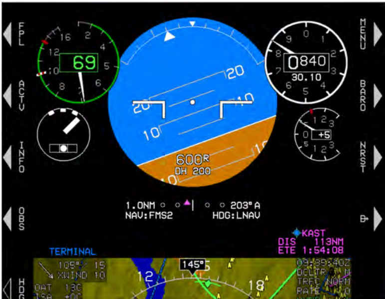
Figure RD-1: Pitch Scale
