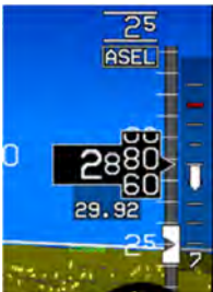
Figure 3-15: Target Altitude Bug (Not Vertically Integrated)
