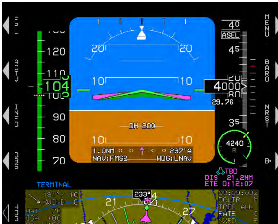
Figure 3-53: Flight Director FD1 Single Cue (Basic Mode with Compass Rose Detected on Bottom Area)
