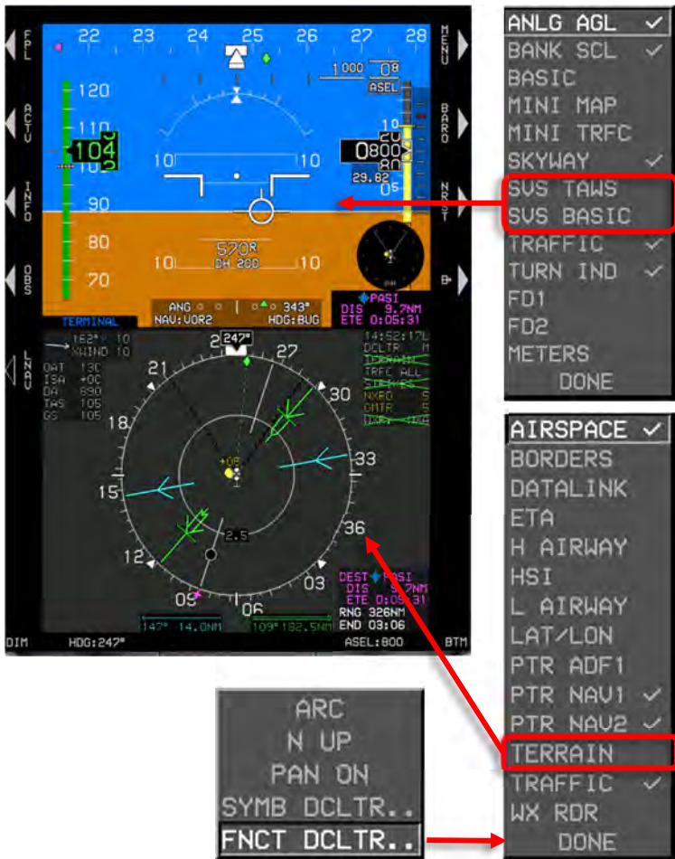
Figure 8-14: Terrain Display Functionality TAWS Disabled
