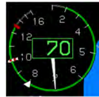
Figure RD-7: Airspeed Display with ADC Failure
