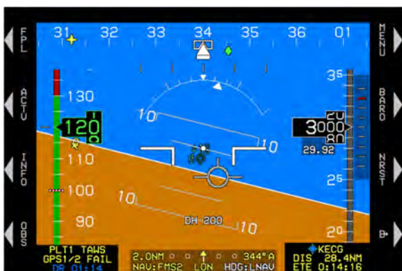
Figure 3-43: Flight Path Marker Grayed to Indicate Degraded Condition with GPS Failure
