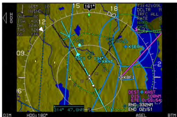
Figure 3-78: Analog Navigation Symbology, HSI overlay with Map in ARC Mode
