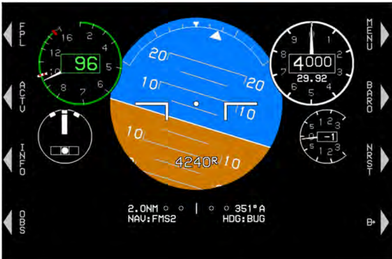
Figure RD-5: Bank Angle Scale Sky Pointer Type
