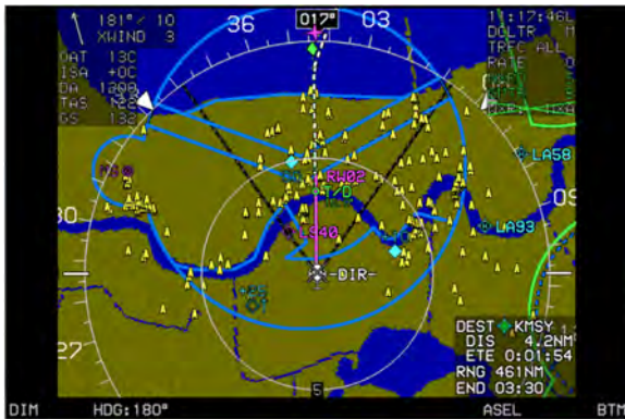
Figure 3-70: Moving Map with Instrument Approach
