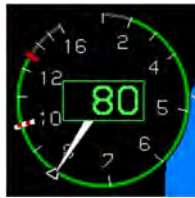
Figure RD-7: Airspeed Display with ADC Failure
