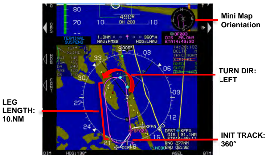
Figure SAR-11: Race Track Pattern-Turn, Leg, and Track
