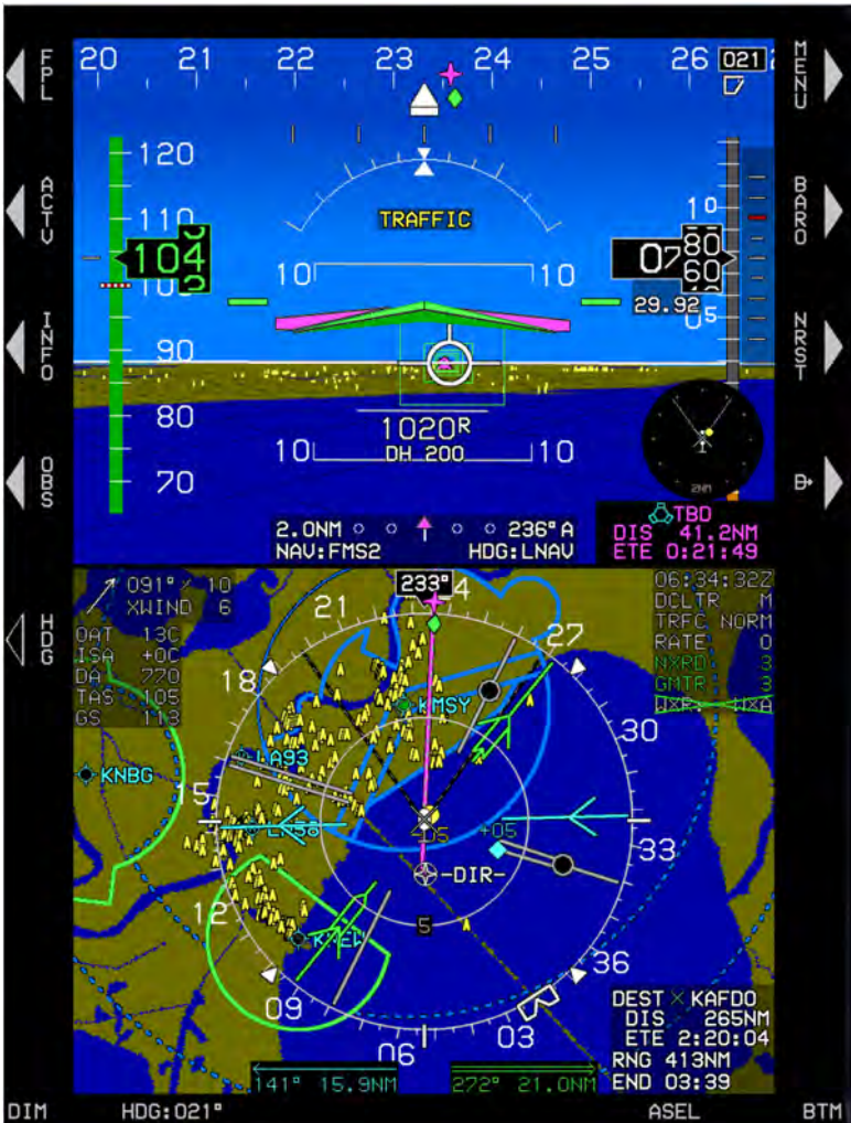
Figure 2-1: IDU-680 Primary Flight Display (PFD) and Map Page
