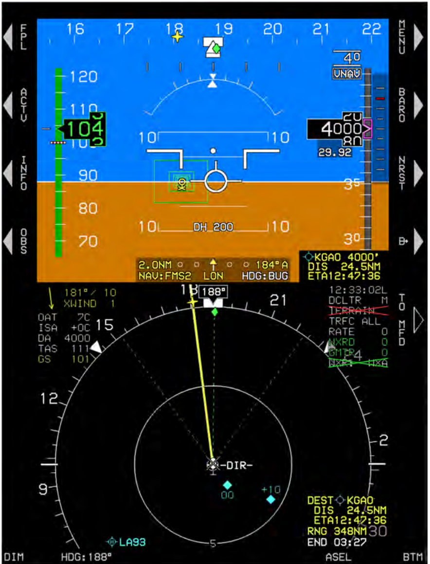
Figure 4-12: MFD Failure Mode 1 (Essential Mode) GPS/SBAS Failed, ADC and AHRs Normal
