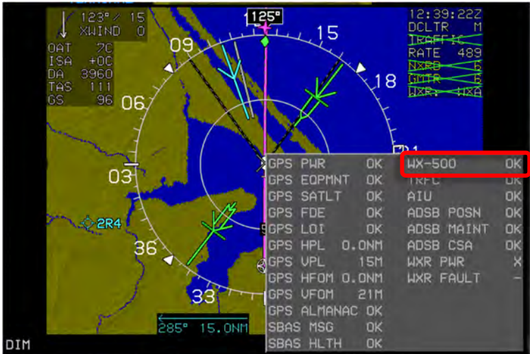
Figure S-10: MFD Fault Display Menu
