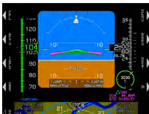
Figure 3-2: PFD in Basic Mode (with Compass Rose Detected on Bottom Area)
