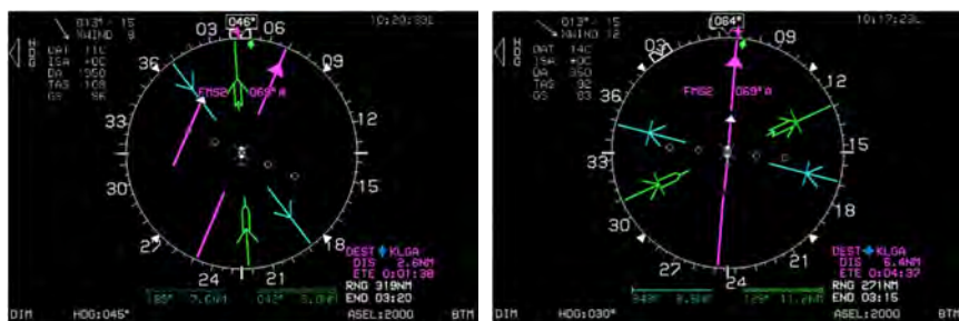
Figure 3-96: Analog Navigation Display VOR1/TAC1 and VOR2/TAC2
