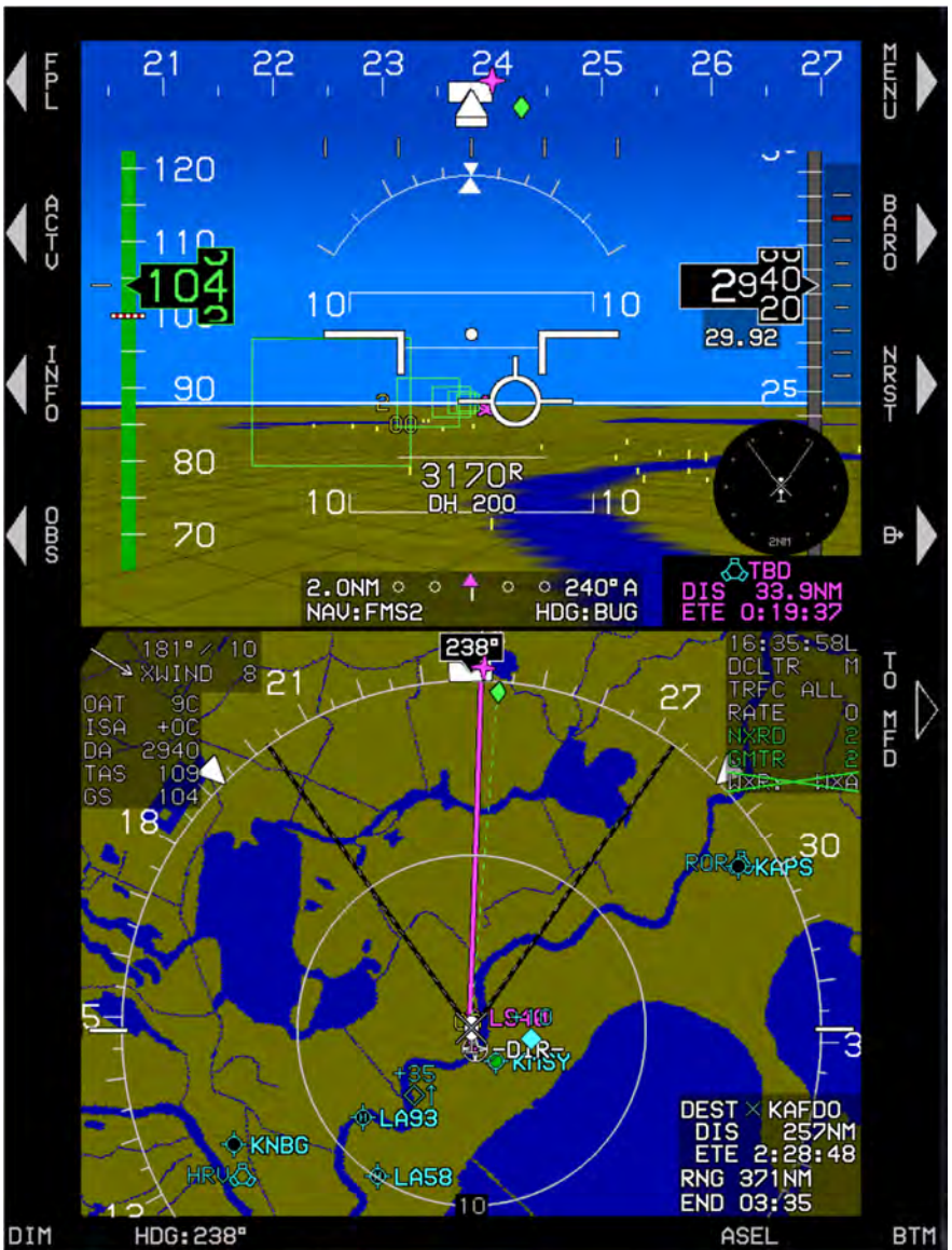
Figure 4-9: MFD Failure Mode 0 (Essential Mode) GPS, ADC and AHRS Normal
