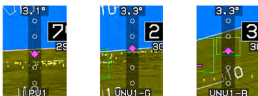
Figure 7-13: Vertical Deviation Indicator Linear Deviation
