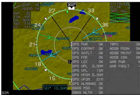
Figure 4-4: FAULTS Page on PFD or MFD
