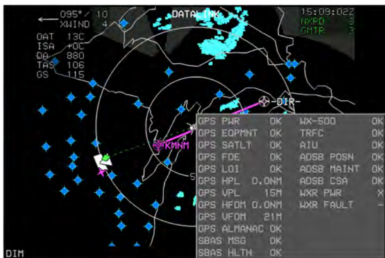
Figure D-12: FAULTS Menu with ADS-B Status
