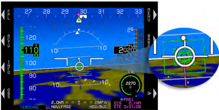
Figure 3-41: Flight Path Marker
