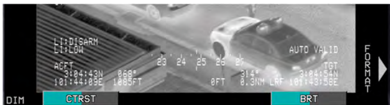
Figure V-1: PFD Page First-Level Video Control
