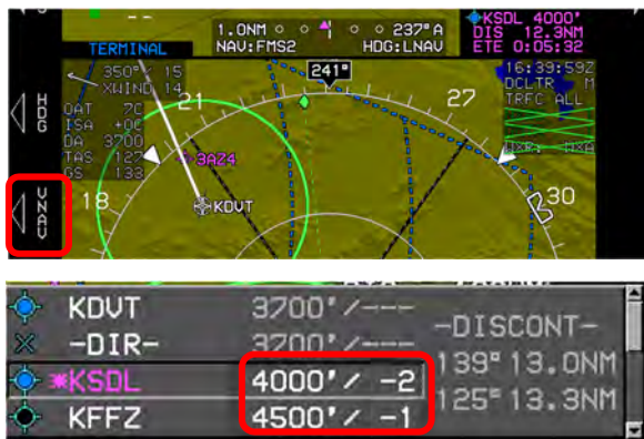
Figure 3-16: Altitude Display (VNAV Tile)
