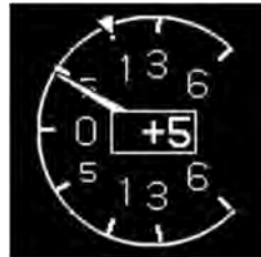
Figure RD-16: Vertical Speed Indicator
