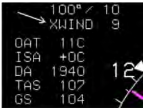
Figure T-12: Air data and Ground Speed
