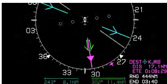
Figure 3-77: HSI Bearing Distance Readout
