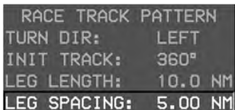
Figure SAR-10: Race Track Pattern Parameters
