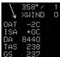
Figure S-2: Air Data and Groundspeed in Upper Left Corner
