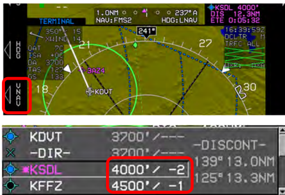
Figure 3-15: Altitude Display (VNAV Tile)
