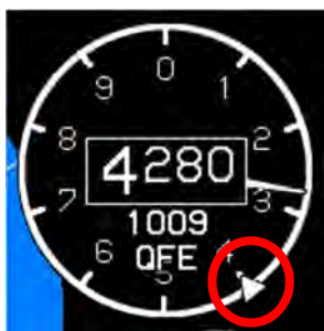
Figure RD-8: Airspeed and Altitude with Loss of ADC
