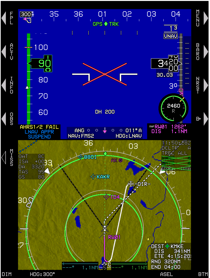
Figure 4-15: PFD Failure Mode 3 (Normal Mode) AHRs Failed, GPS/SBAS and ADC Normal
