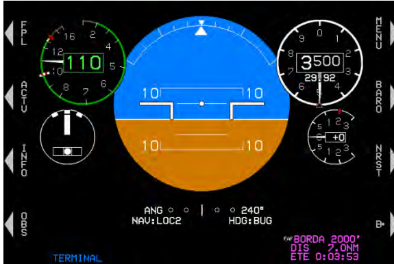
Figure RD-1: Round Dials Airspeed Display
