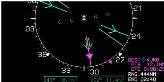
Figure 3-72: HSI Bearing Distance Readout
