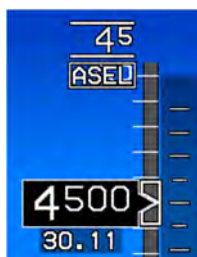
Figure 3-14: Selected Altitude Sub-Mode (Target Altitude)
