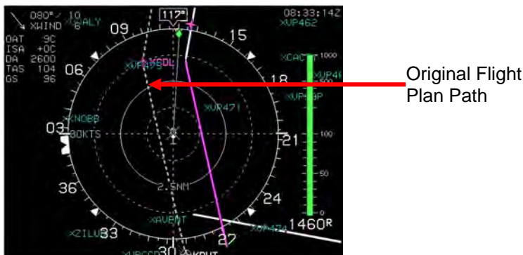
Figure 3-104: Hover Vector Active Flight Plan Path/Parallel Course
