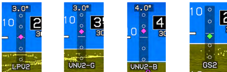
Figure 3-54: Vertical Deviation Indicator
