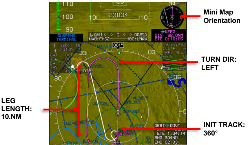
Figure SAR-14: Race Track Pattern-Turn, Leg, and Track
