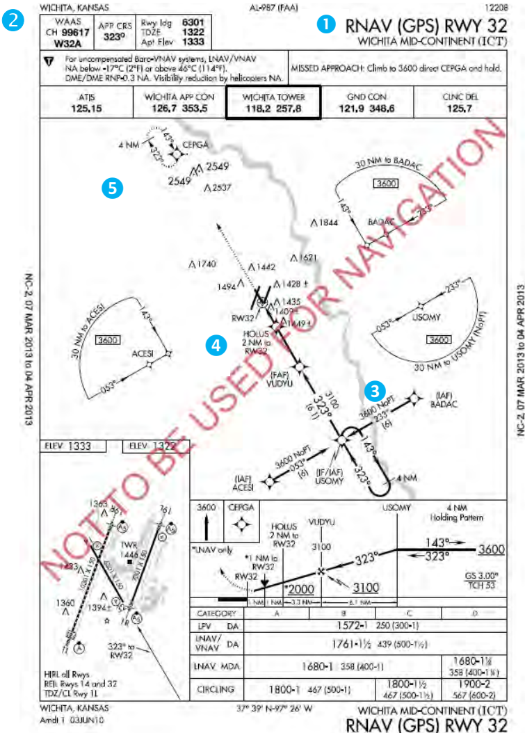
Figure 7-16: RNAV (GPS) Instrument Approach to LPV Minima
