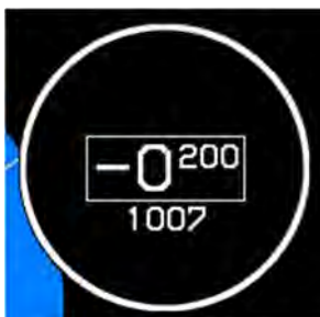
Figure RD-7: Altitude Display (When Below Sea Level)
