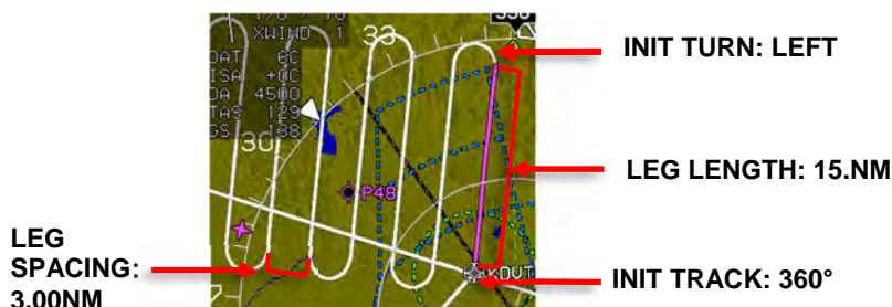
Figure SAR-7: Rising Ladder Pattern-Turn, Leg, and Track
