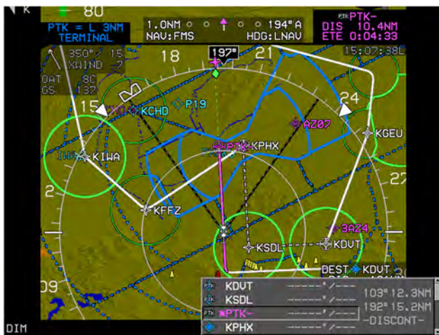
Figure 7-9: Parallel Offset PTK-/PTK ENDING
