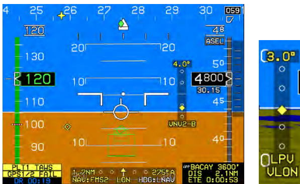
Figure 3-55: VDI Color during GPS/SBAS LON or VLON
