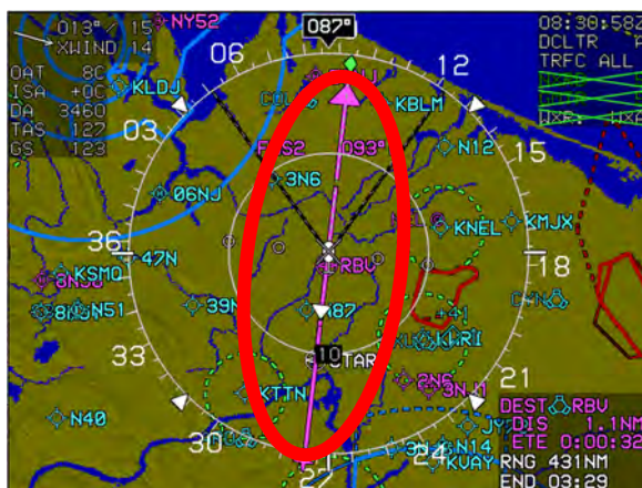
Figure 3-74: Analog Navigation Symbology, HSI in Centered Mode
