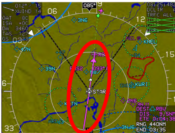
Figure 3-73: Analog Navigation Symbology, HSI in ARC Mode
