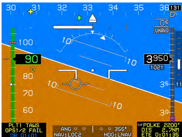
Figure 3-39: Flight Path Marker Grayed to Indicate Degraded Condition with GPS Failure
