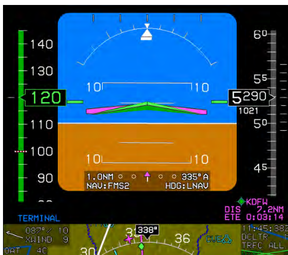
Figure 3-49: Flight Director FD1 (Basic Mode with Compass Rose Detected on Bottom Area)
