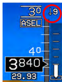
Current rate of descent is 900 fpm and VSI bug set to -900 fpm.
