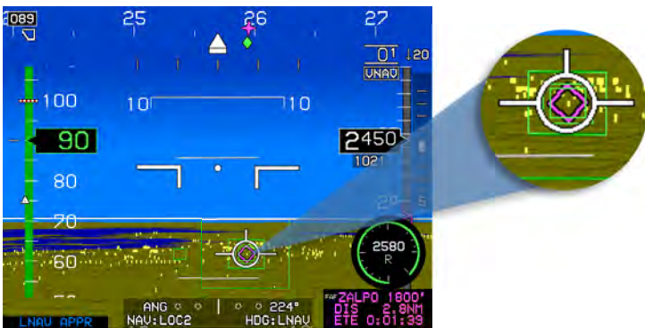
Figure 3-37: Flight Path Marker
