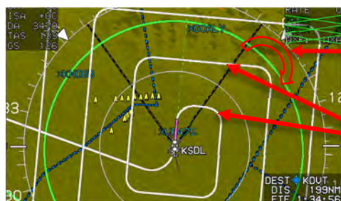
Figure SAR-3: Expanding Square Pattern-Turn and Leg
