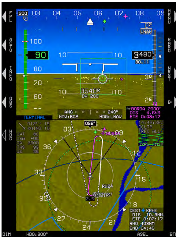
Figure 2-9: IDU #1 PFI on Top and Map on Bottom
