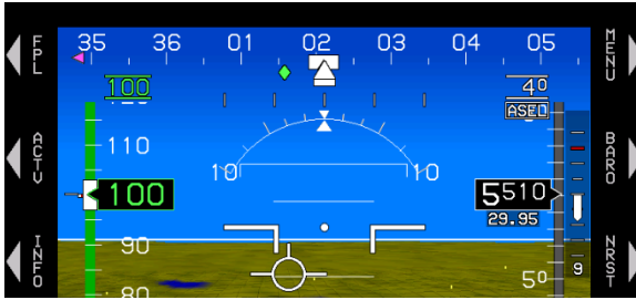
Figure 3-30: Airspeed Display (with EFIS-Coupled)
