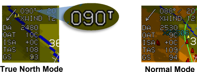
Figure 3-75: Air Data and Groundspeed
