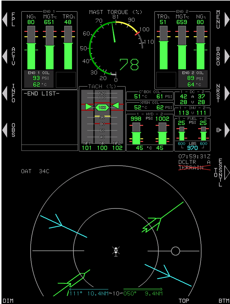
Figure 4-26: MFD Failure Mode 7 (Normal Mode) GPS/SBAS, ADC and AHRs Failed
