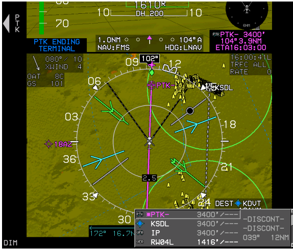
Figure 7-9: Parallel Offset PTK-/PTK ENDING
