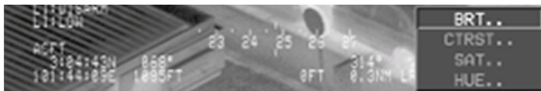
Figure V-1: Encoder Functions for MFD Video Page
