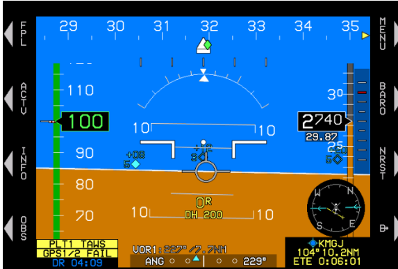
Figure 3-45: Flight Path Marker Grayed to Indicate Degraded Condition with GPS Failure
