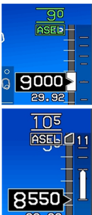
Figure 3-12: Target Altitude Bug (Vertically Integrated)
