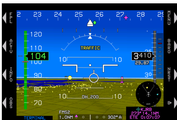
Figure 2-17: Time-Critical Caution Alert
