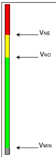
Figure 3-29: Airspeed Scale FAR Part 27/29
