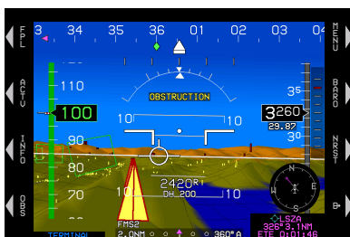
Obstructions creating an OBSTRUCTION caution
