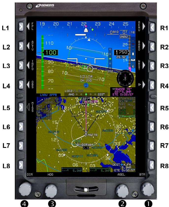
Figure 5-1: IDU-680 Input Controls
