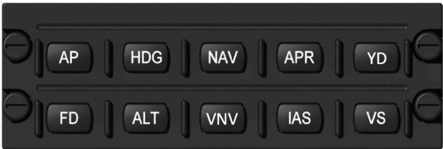
Fig. 1-1. DFCS-2G Control Panel
