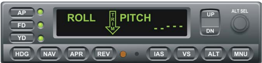
Fig. 3-16. AP Display, AUTO TRIM DN in Progress
