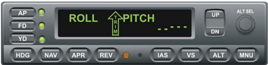
Fig. 3-15. AP Display, AUTO TRIM UP in Progress
