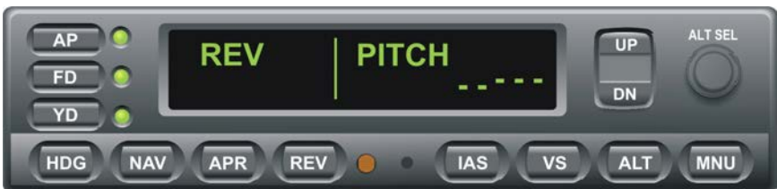
Fig. 3-38. AP Display, REV Mode Engaged, Track VOR Front Course Outbound
