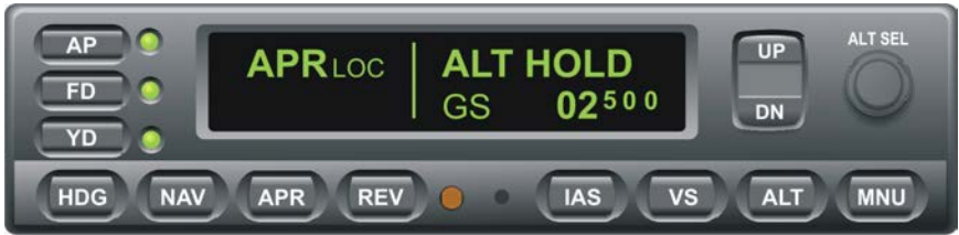
Fig. 3-18. AP Display, APR LOC and ALT HOLD Modes Engaged, GS Mode Armed
