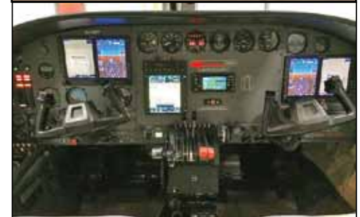
Patrick Dougherty’s 414. The 2100 is a 21st century autopilot that matches the quality and capability of modern glass panels.
