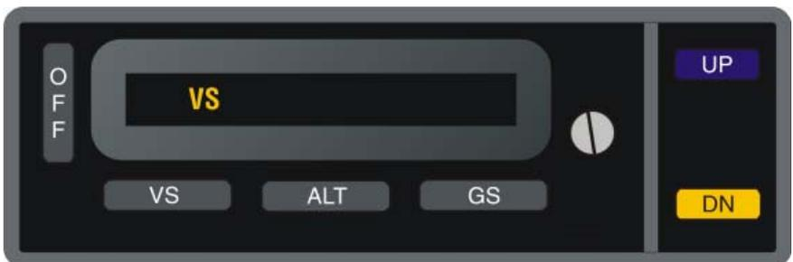
**Fig. 2-3. AP Display, VS Mode Engaged**
