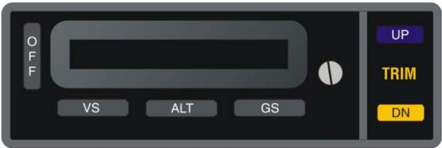
Fig. 3-4. AP Display, Manual Electric Trim in Progress
