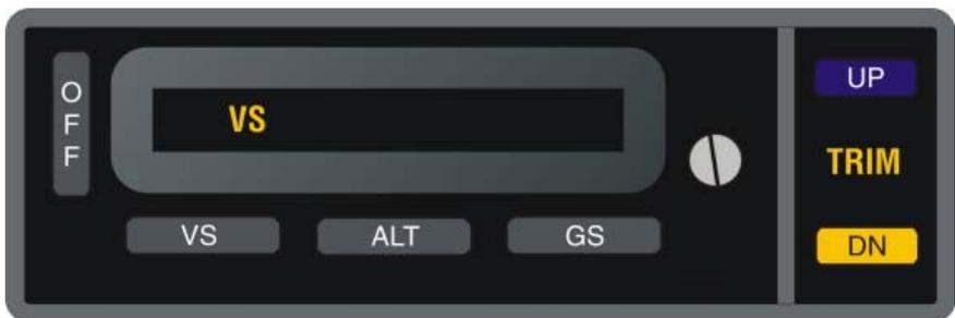
**Fig. 2-5. AP Display, VS Mode Engaged, TRIM Required**
