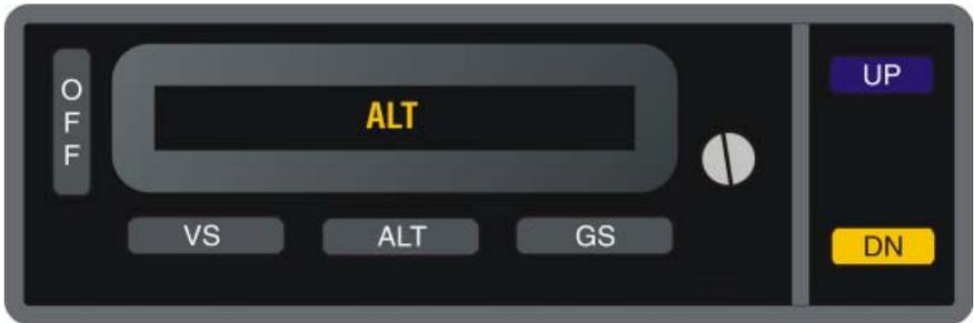
Fig. 3-5. AP Display, ALT HOLD Mode Engaged
