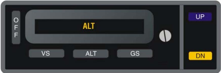
Fig. 3-2. AP Display, ALT HOLD Mode Engaged
