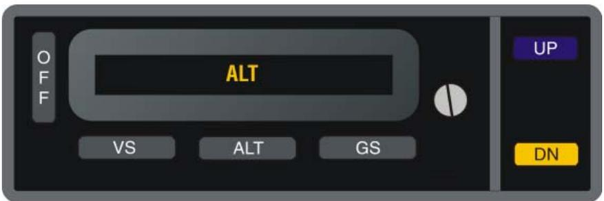
**Fig. 2-4. AP Display, ALT HOLD Mode Engaged**
