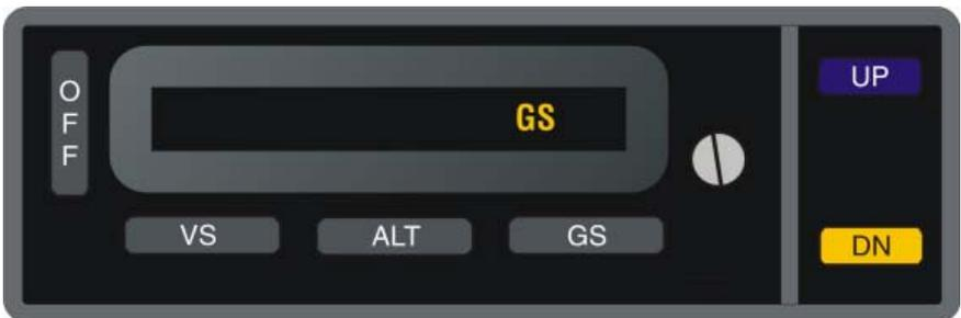
Fig. 3-7. AP Display, GS Mode Engaged
