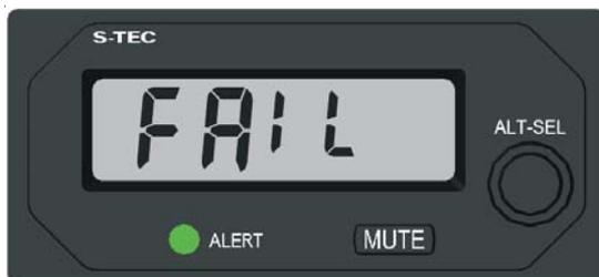
**Fig. 4-1. Altitude Selector / Alerter Fail Indication**
