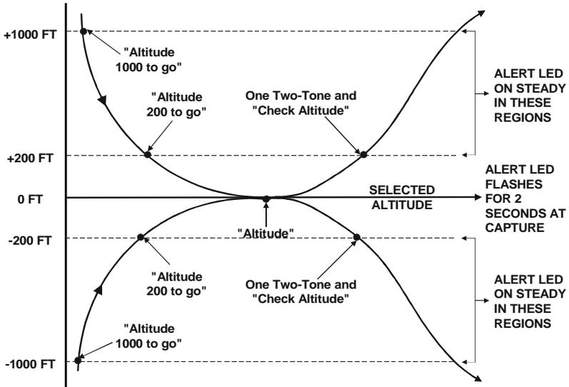
**Fig. 4-2. Altitude Selector / Alerter Annunciation Flight Profile**
