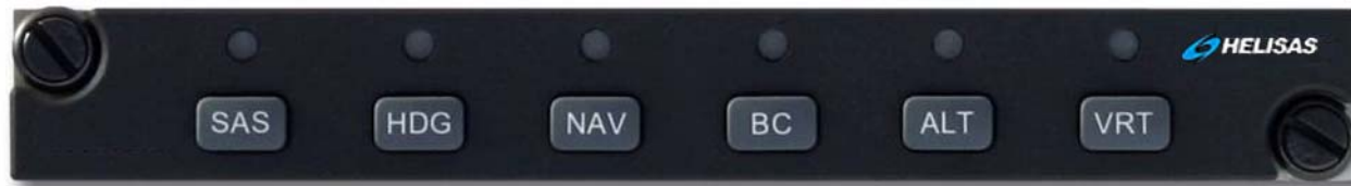
Figure 1 - HeliSAS Control Panel
