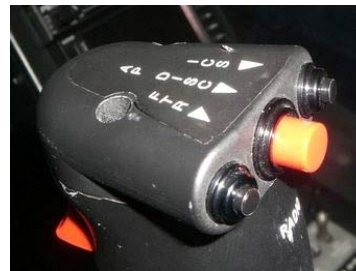
Figure 2 - FTR Switch and AP DISC Switch
