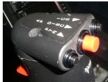
**Figure 2 - FTR Switch and AP DISC Switch**
