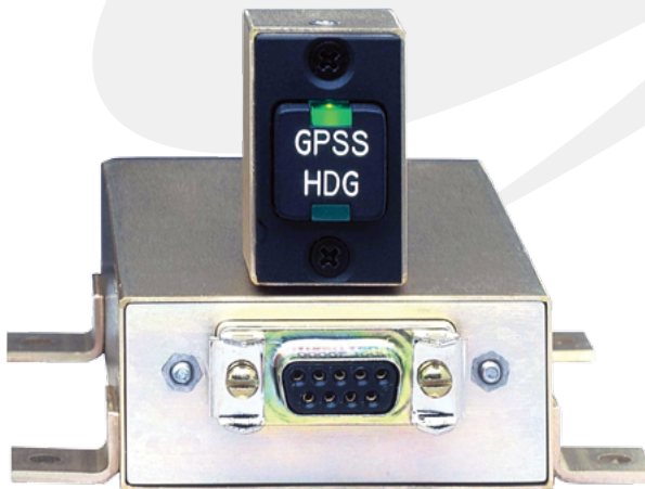
To save valuable panel space, the GPSS converter is configured as a separate panel-mounted switch and remotely-mounted control box. The control switch is 1.32 x .82", and projects only 1" behind the panel (plus cable connector).
