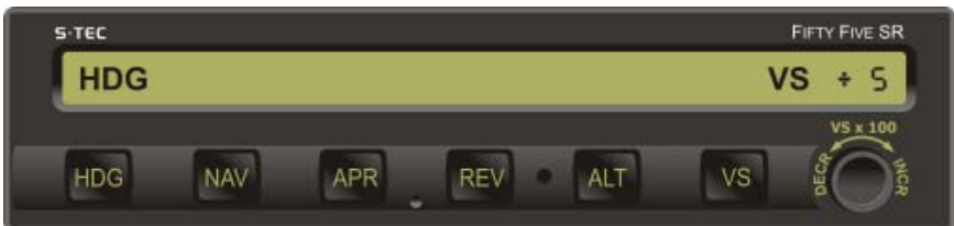
Fig. 2-8. AP Display, HDG and VS Modes Engaged, 500 FPM Climbing (Pre-Flight)
