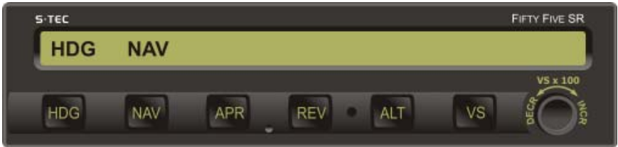
Fig. 3-4. AP Display, HDG Mode Engaged, NAV Mode Armed
