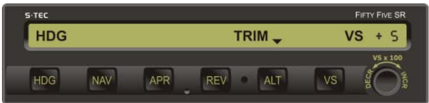
b. TRIM DN in Progress
