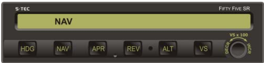
Fig. 3-2. AP Display, NAV Mode Engaged
