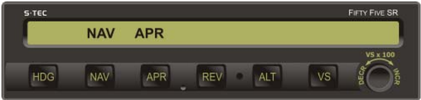
Fig. 3-19. AP Display, NAV APR Mode Engaged, Track VOR Front Course Inbound
