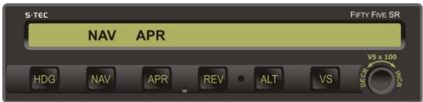
Fig. 3-22. AP Display, NAV APR Mode Engaged, Track LOC Front Course Inbound
