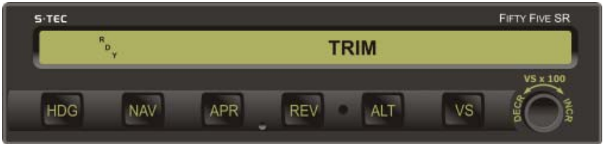
Fig. 3-10. AP Display, Manual Electric Trim in Progress
