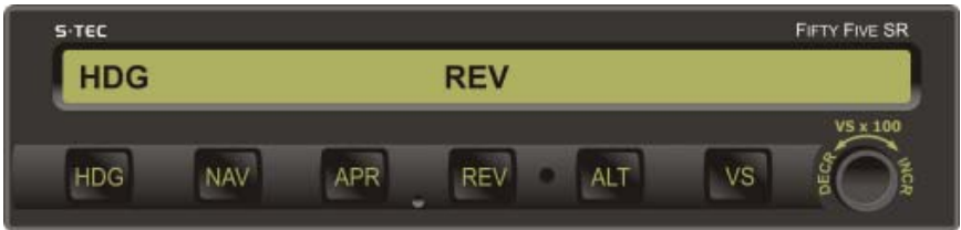
Fig. 3-13. AP Display, HDG Mode Engaged, REV Mode Armed
