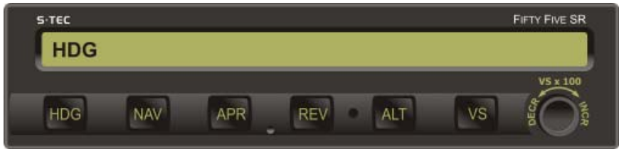
Fig. 3-1. AP Display, HDG Mode Engaged
