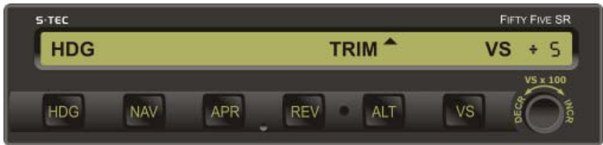
a. TRIM UP in Progress
