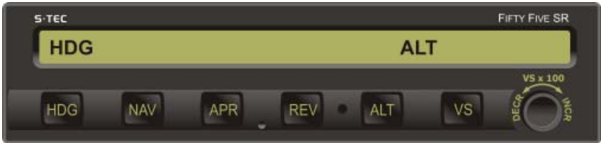
Fig. 2-6. AP Display, HDG and ALT HOLD Modes Engaged (Pre-Flight)
