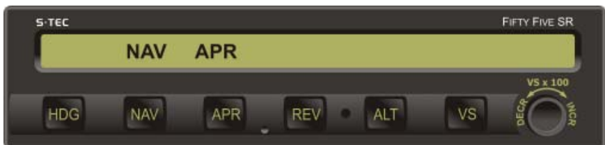
Fig. 3-25. AP Display, NAV APR Mode Engaged, Track VOR Front Course Inbound
