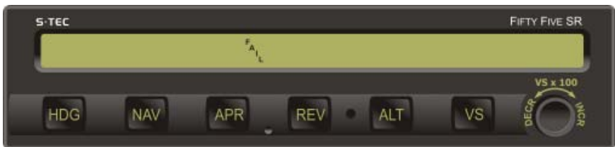
Fig. 2-4. AP Display, Programmer/Computer Failure
